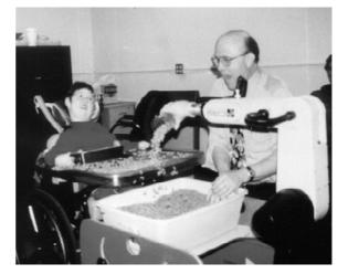
Fig. 1. The robotic system. The robot arm is shown in the foreground. The child was able to dig and find objects hidden in a tub of dry macaroni.
