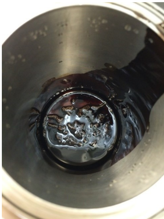
Figure 7-26 View of the emulsion sample at the bottom of autoclave after dewatering by 50 ppm demulsifier B at 80 ^{\circ}\text{C} .
