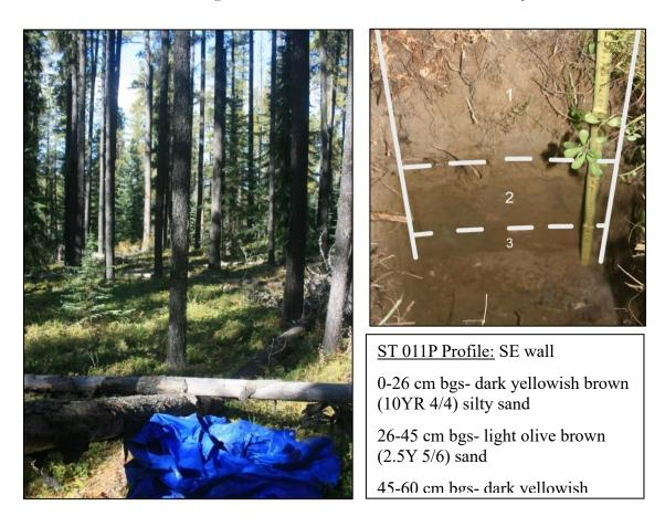
Judgmental slope testing was conducted southeast of Transect 2 on the southeastern nose of the dune. Locations for the tests were selected based on the varying grades and aspects of the slope. A total of three subsurface tests were conducted on the southeastern slope of the dune nose (Photo 11).
