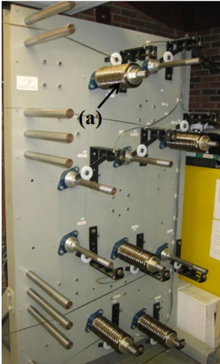
Figure 2-25: The (a) basalt fiber creels attached to the tensioning system
