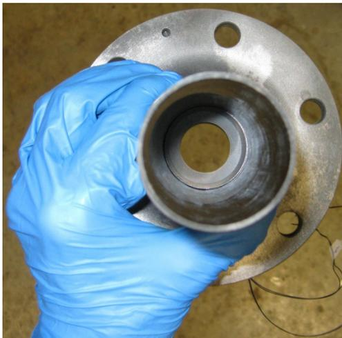
Figure 2-3: A 38.1 mm specimen bonded to the supply flange
