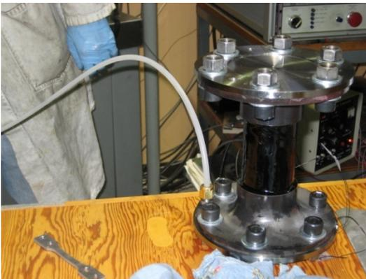
Figure 2-17: The specimen is pressurized with air to 207 kPa.
