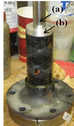
Figure 2-5: The (b) alignment cylinder aligning the 50.8 mm specimen
