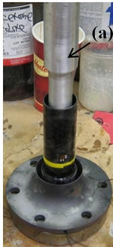
Figure 2-4: A 38.1 mm specimen employing (a) the alignment jig
