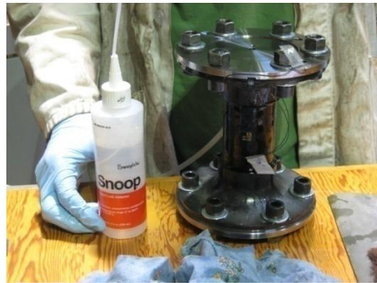
Figure 2-18: Snoop is poured over the specimen to test for leaks.
