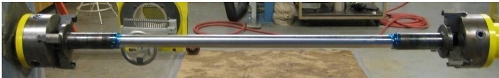
Figure 2-28: An installed 1.5 inch mandrel
