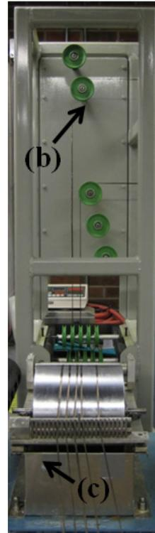
Figure 2-26: The (b) routing system and (c) epoxy bath
