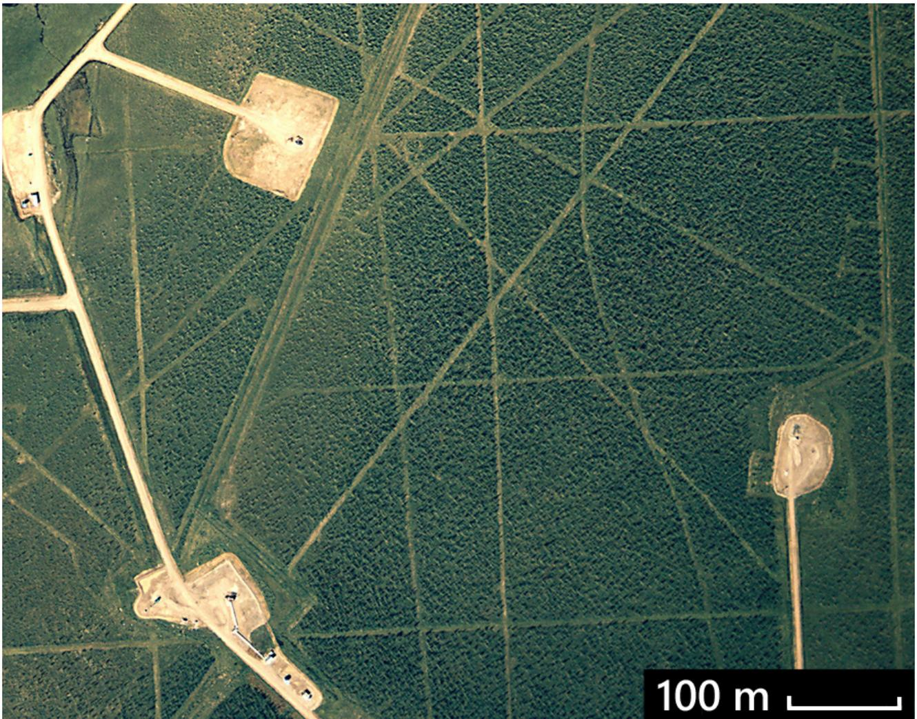
*Fig. 5.11. The industrial footprint of oil and gas development in northern Alberta, illustrating well sites (pale squares), access roads (thick lines), and seismic lines (thin lines). Credit: Air Photo Services.*
