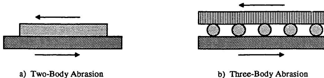
Figure 1-5. Two-Body and Three-Body Abrasion
