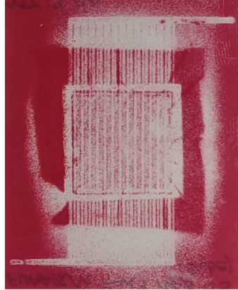
Figure 3.8 – Pressure film measurement demonstrating proper compression of the MEA and sealant of the cell.
