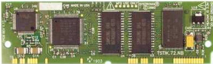
Figure 6 - T-Stik with DS80C400 chip – standard 72 pin DIMM
