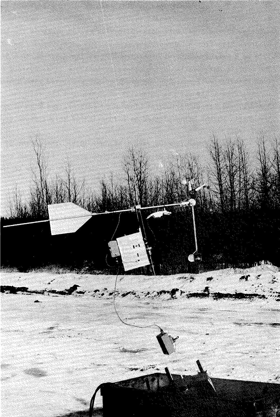
Figure 14. Detailed photograph of the tether sonde package that was used in this study, February 1977.
