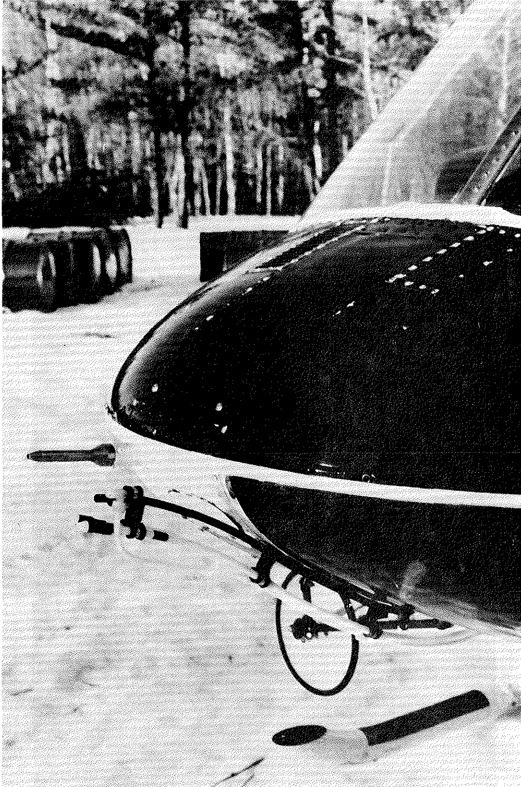
Figure 61. Details of the sample intake mounted on the helicopter.
