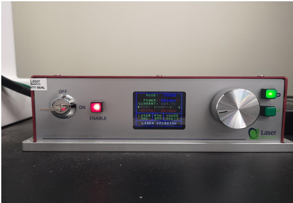
Figure 2.4. Laser system control module. The red “ENABLE” light indicates the laser is on.
