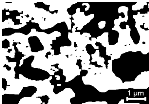
Figure 4.1 – 2D image of an SOFC electrode cross section obtained using FIB-SEM
