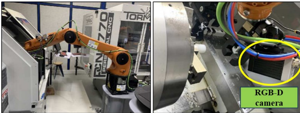
Figure 2.6: The example of machine monitoring, adapted form [24].
