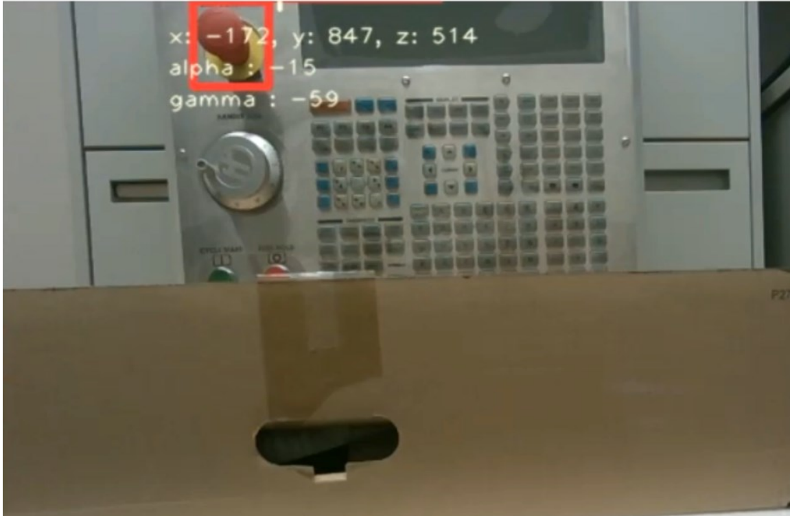
Figure 6.12: The examples of emergency button detection and localization.
