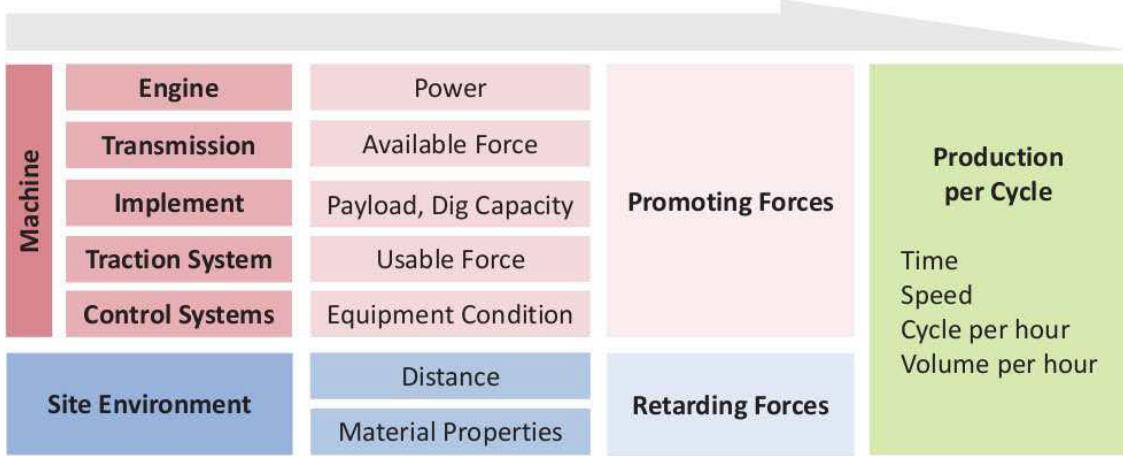
Figure 2.1: Machine and Environmental Factors Contributing to the Production, after [Tatum et al., 2006a]
