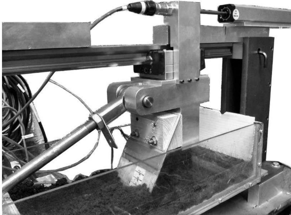
Figure 4.4: Shovel Assembly with the Blade at an Attack Angle of  $\alpha = 70^\circ$
