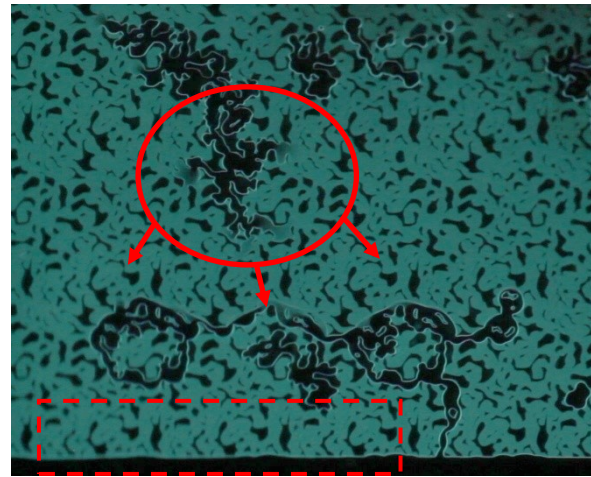
b) Upper vapourized solvent (arrowed circle) expands downward contracting lower vapor region and pushing solvent toward the fracture (dashed square) t=1 sec.
