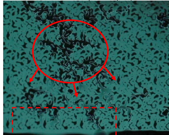
d) Some solvent is driven through the fracture. t=3 sec.
