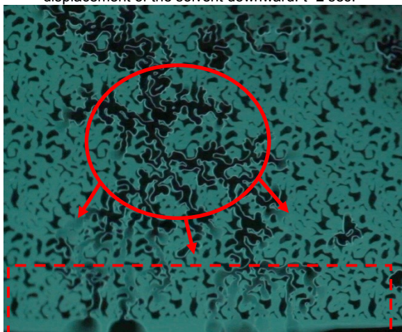
e) Solvent continues producing in the fracture. t=4 sec.
