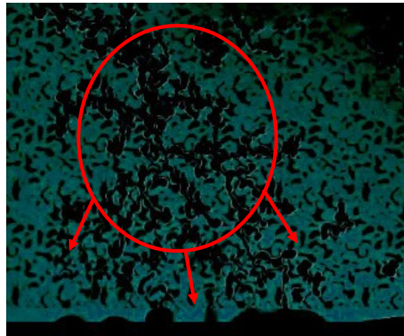
h) Vapor communication starts with the fracture. t=7 sec.
