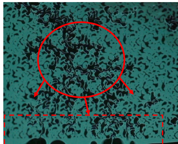
f) Vapor phase growth toward the fracture. t=5 sec.
