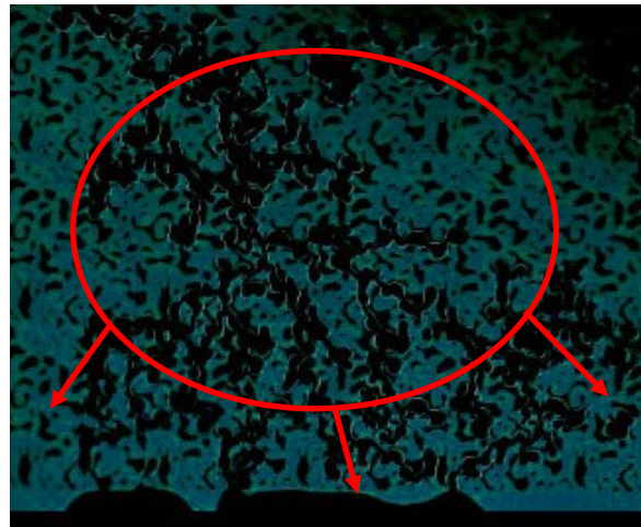
j) Vaporized solvent is drained via fracture by the existent vapor channels and through liquid solvent displacement. t=9 sec.
