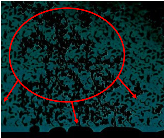
i) More bubbles are connected to the fracture. t=8 sec.
