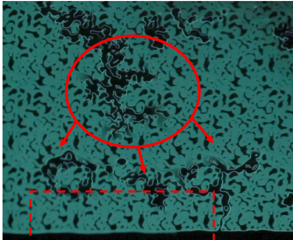
c) Upper solvent vapor continues its expansion by the displacement of the solvent downward. t=2 sec.
