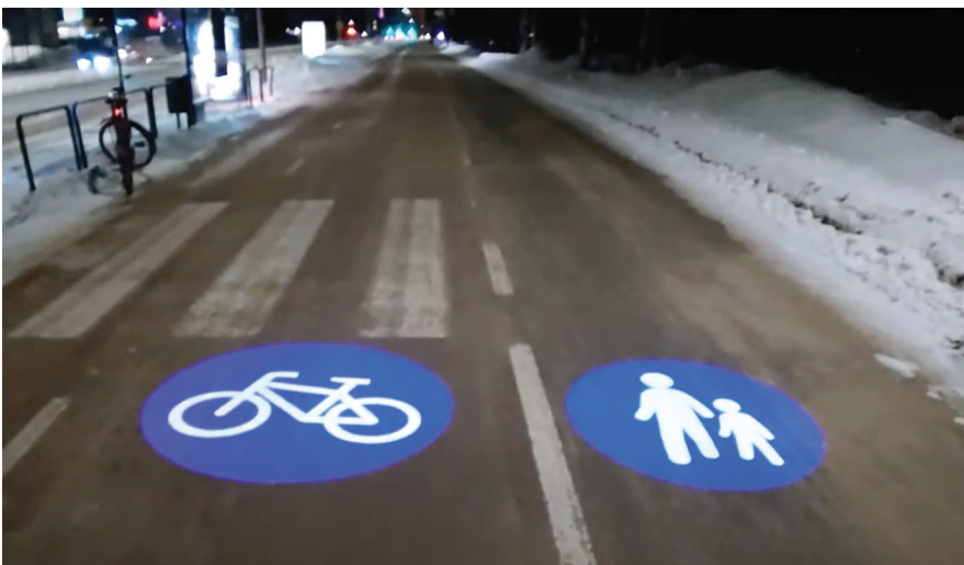
FIGURE 9: A projected light illuminates traffic signs on a snowy surface of a cycling path in Oulu, Finland. Image credit Pekka Tahkola. Image used with permission by Pekka Tahkola.
