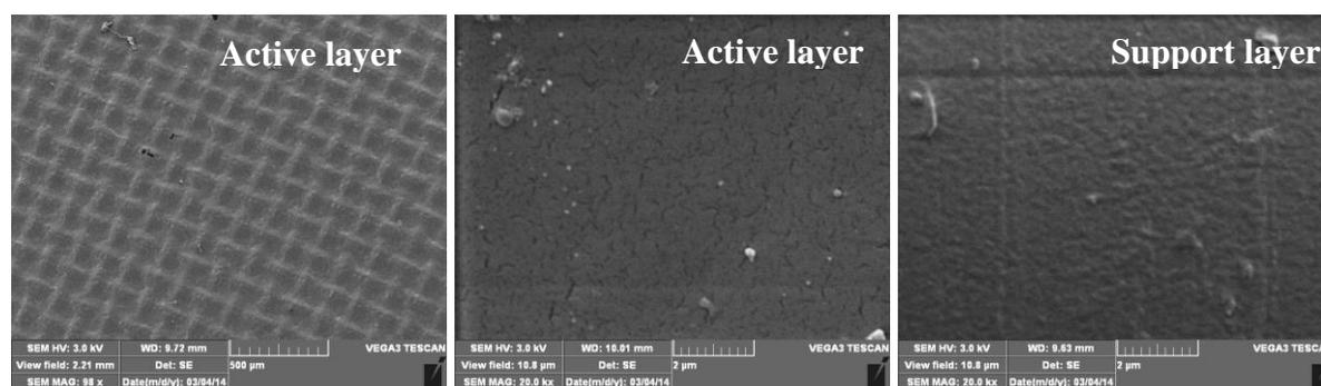
Figure 4. Typical SEM images of FO membranes. A forward osmosis membrane was coated with 5 nm gold by sputter coating and visualized with a Vega-3 SEM.
