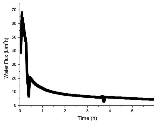
Figure 5. Permeate water flux through FO membrane using 4M  $\text{NH}_4\text{HCO}_3$  as a draw solution.
