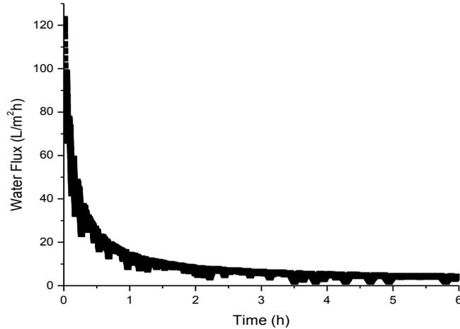
Figure 7. Permeate water flux through FO membrane after water backwash.
