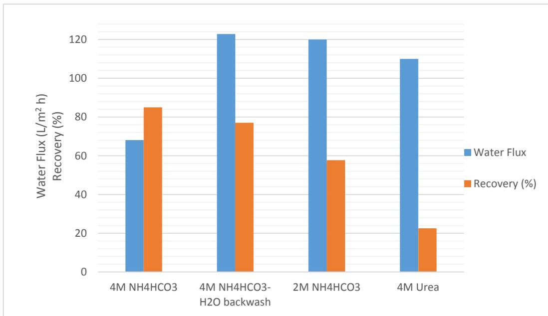
Figure 9. Comparisons of water flux and water recovery through FO membrane using different draw solutions.
