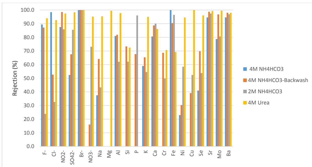
Figure 10. Ion and metal rejection by an FO membrane using different draw solutions.
