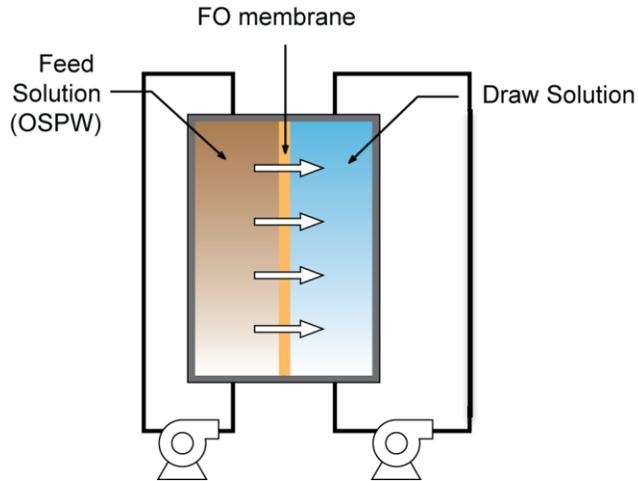
Figure 2. Forward osmosis system design for OSPW treatment.
