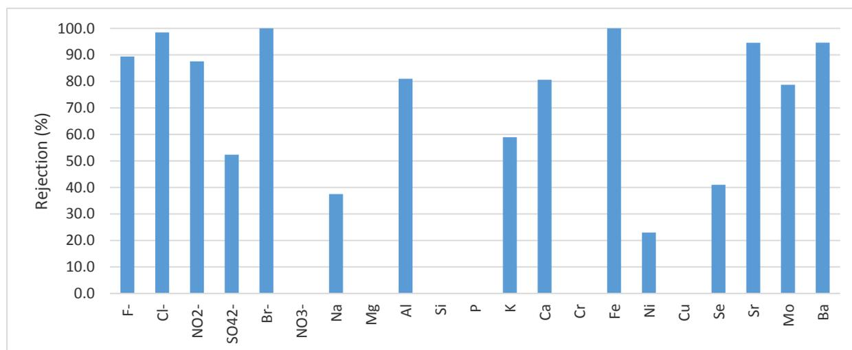
Figure 6. CTA forward osmosis membrane rejection of ions and metals in OSPW.
