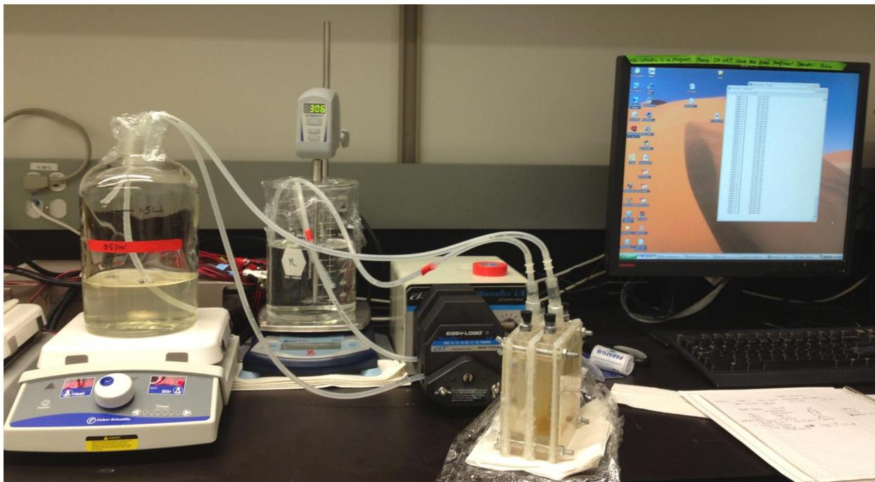
Figure 3. Laboratory scale forward osmosis system for OSPW treatment.
