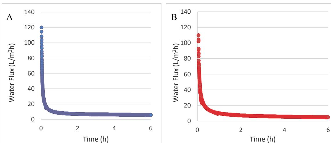
Figure 8. Permeate water flux through forward osmosis membrane for OSPW treatment using 2M  $\text{NH}_4\text{HCO}_3$  (A) and 4M urea (B) as draw solutions.
