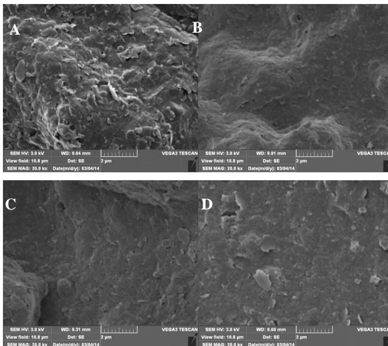
Figure 11. SEM images of OSPW fouled FO membranes. FO was performed using 4M  $\text{NH}_4\text{HCO}_3$  (A, B), 2M  $\text{NH}_4\text{HCO}_3$  (C), and 4M urea (D) as draw solutions. The membrane in B is shown after water backwash.
