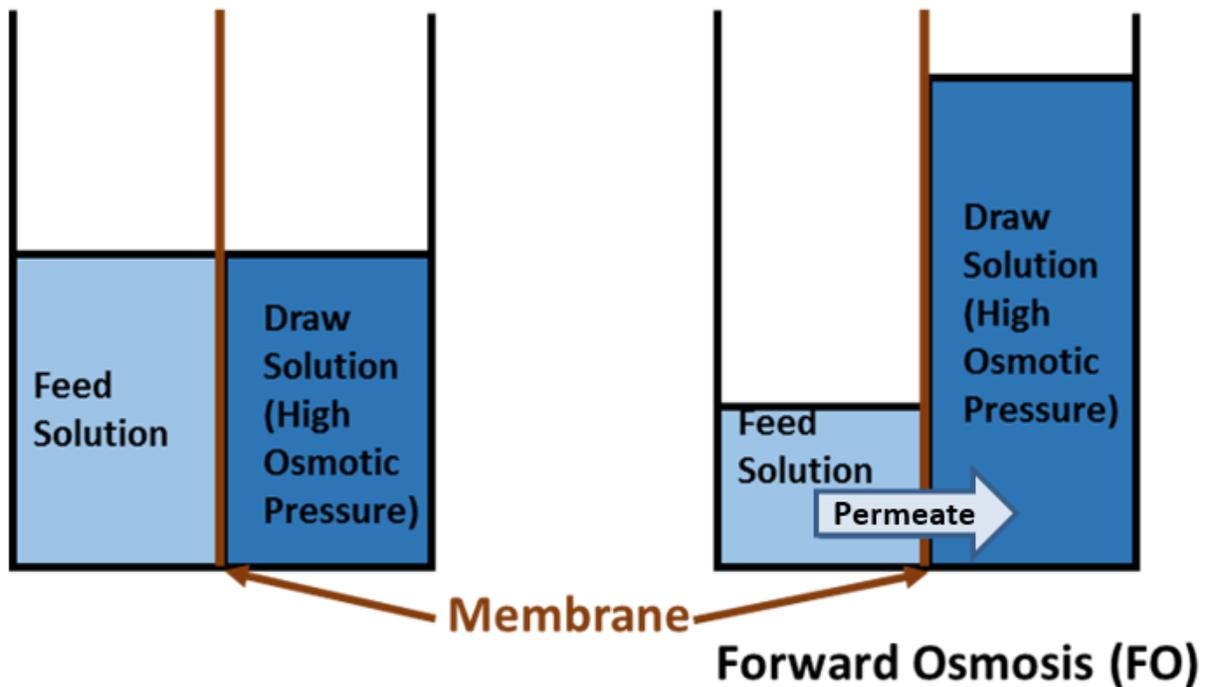
Figure 1. Principle of a forward osmosis treatment system.
