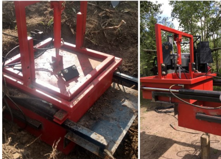
Figure 1: Large-scale shear box built for this study. 0.8 m x 0.8 m x 0.6 m (H) split in half height, the upper part of the box is pushed by two hydraulic cylinders to shear the soil block. There is a lid on the top for Normal force powered by a single hydraulic cylinder with an independent pump. On the right, cylinders fully extended to a displacement of 0.3 m.
