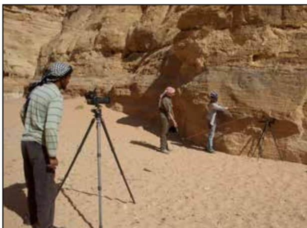
30. Capturing Reflectance Transformation Imaging data on an inscription carved near Ḥumayma's dam.
