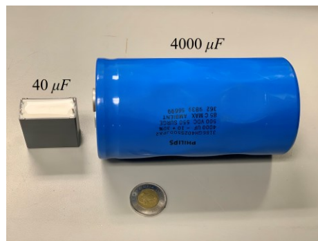
Fig. 3.20: Reduction of capacitor size. Left: 40 \mu\text{F} film capacitor currently used. Right: 4000 \mu\text{F} electrolytic capacitor used before start of research
