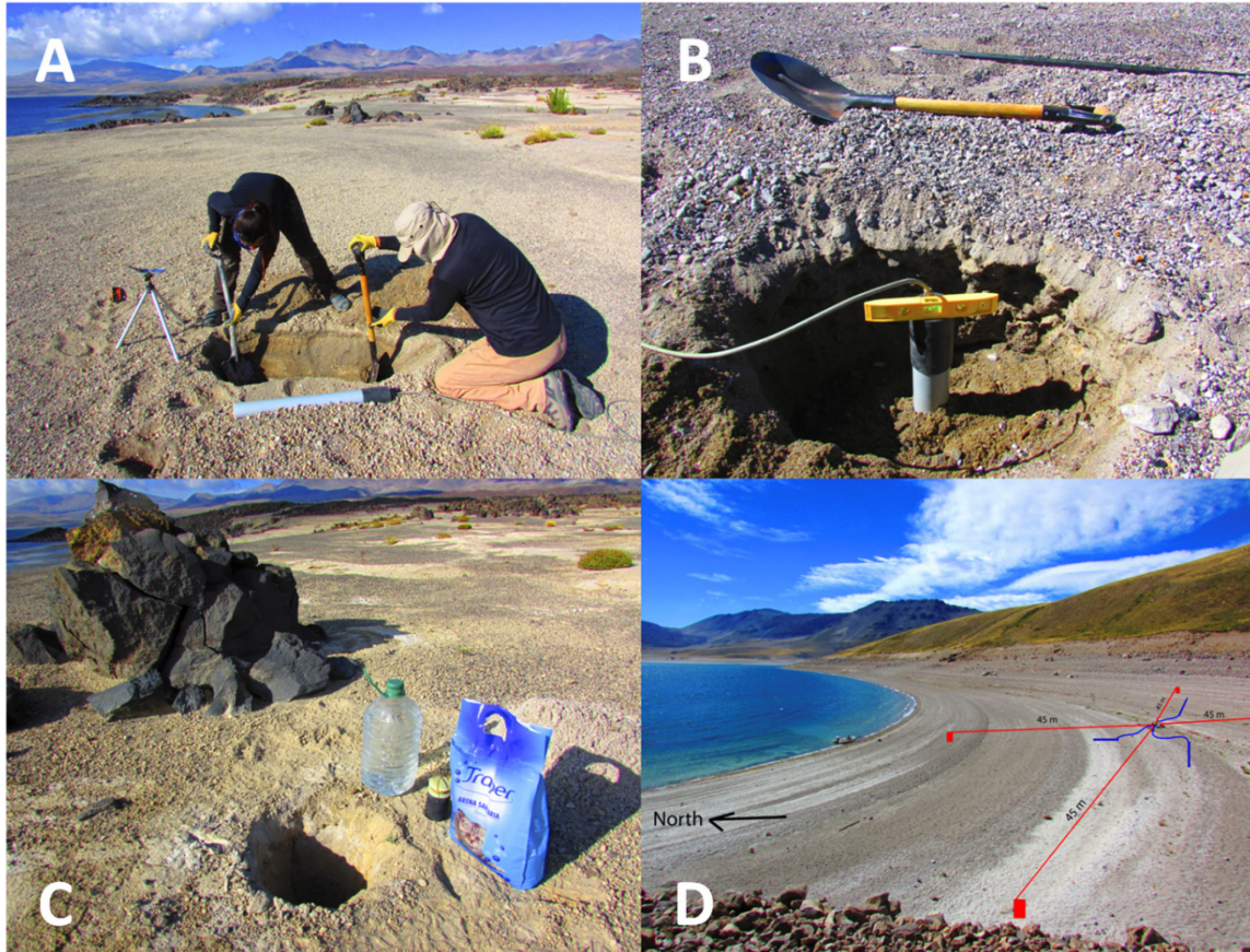
Figure 5.2: Field photos from the field season in 2015. (a) Digging the horizontal H_x induction coil at site LDM013; (b) The vertical H_z induction coil at site LDM013; (c) A hole for the electrode (black cylinder) with water and kitty litter to retain moisture at site LDM013; (d) Site layout on a beach with 90 m dipoles at site LDM006. The inflatable boat is parked on the beach for scale.
