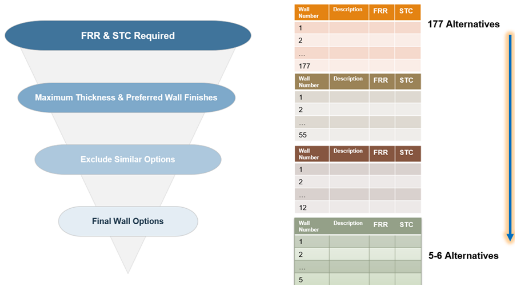
Figure 3-3: Narrowing Down Wall Alternatives
