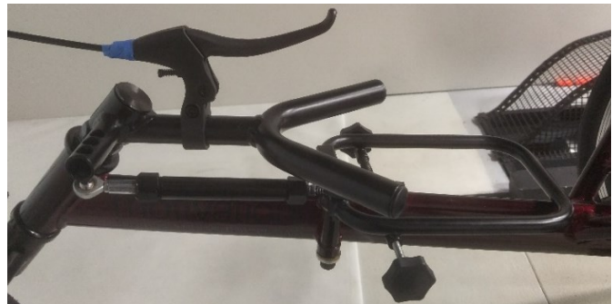
Figure 8. Full view of a racing wheelchair's steering mechanism.
