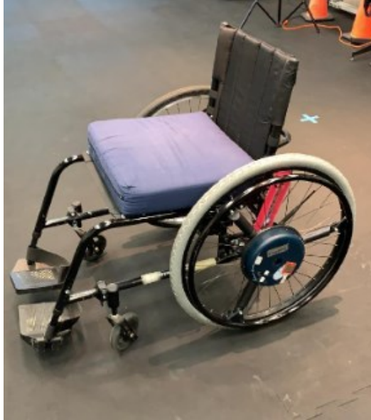
Figure 11. A photo of the SMART wheel designed by Cowan et al. (2008) mounted on the RRL's Quickie four-wheeled manual wheelchair.
