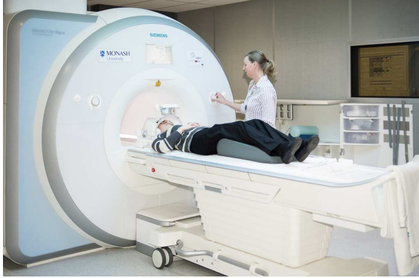
Figure 1.1: fMRI Device (Model: Siemens Skyra). During the fMRI scanning, the subject is placed into the cylindrical magnet machine with strong and homogeneous magnetic field. The neural activity in the brain is observed through imaging blood flow changes. These small changes are detected as minute distortions in the magnetic field by fMRI and employed to generate functional images.
