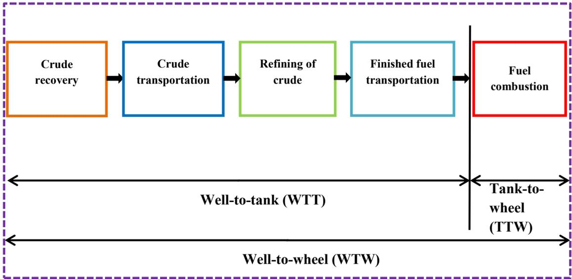
**Figure 10: Life cycle assessment (LCA) boundary**
