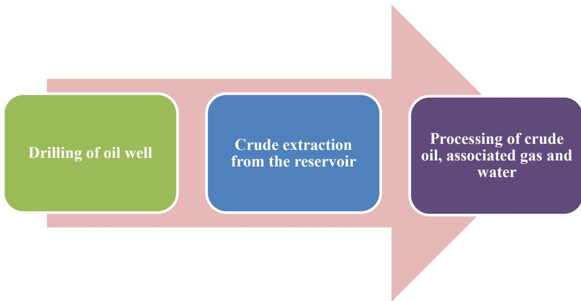
**Figure 2: Crude recovery sub-unit operations**
