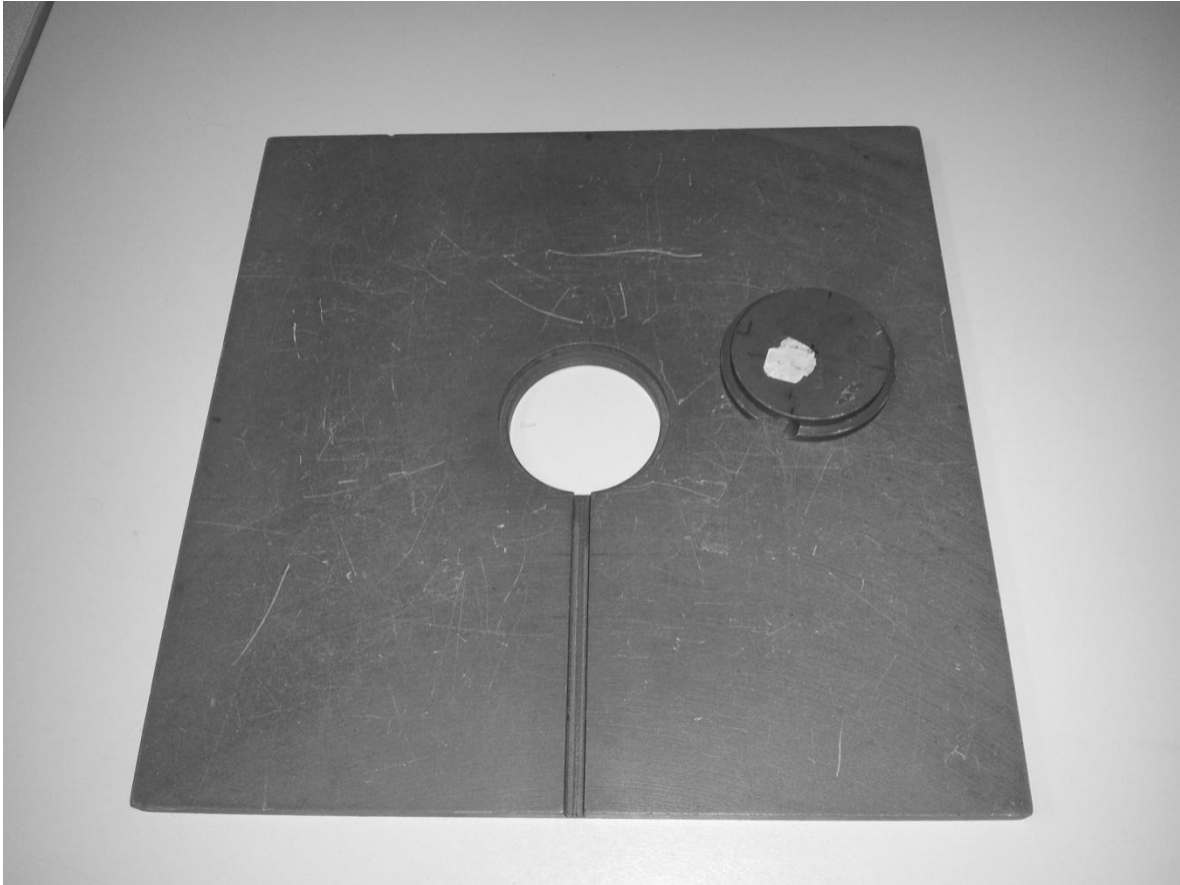
Figure 27: Photograph of solid water slab with insert to house ion chamber.
