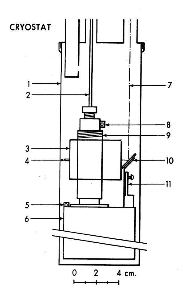
slightly longer dewar (78 cm instead of 73 cm), but with little success. The oscillation would sometime be absent only to appear again spontaneously after the next filling of the dewar. The inside of the dewar is 9 cm and it is connected to a brass head of 12 cm inside diameter and 13 cm length through a Corning flange (Pyrex conical pipe system, Corning Glass works, Corning N. Y.). The round copper can inside the dewar measures 7.5 x 26 cm.
