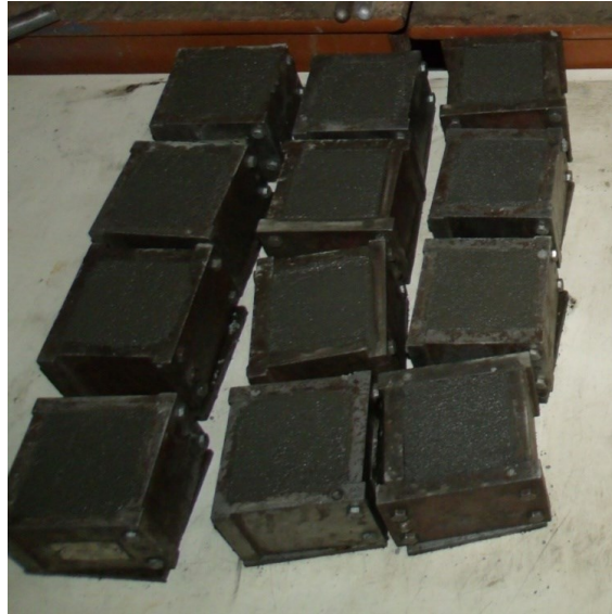
Figure 4-2 Moulds after Being Filled with Cement Mortar Mix and Mechanically Compacted
