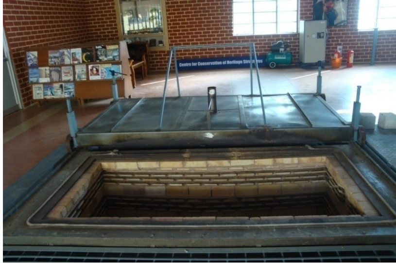
Figure 4-3 Furnace with Capacity of 1000°C
