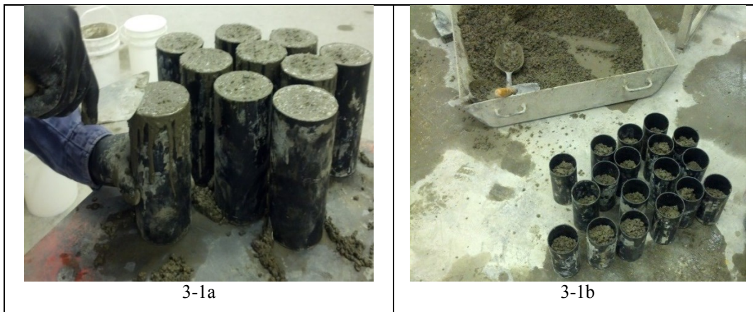
Figure 3-1- Moulds While Being Filled With Concrete Mix on Vibrator
