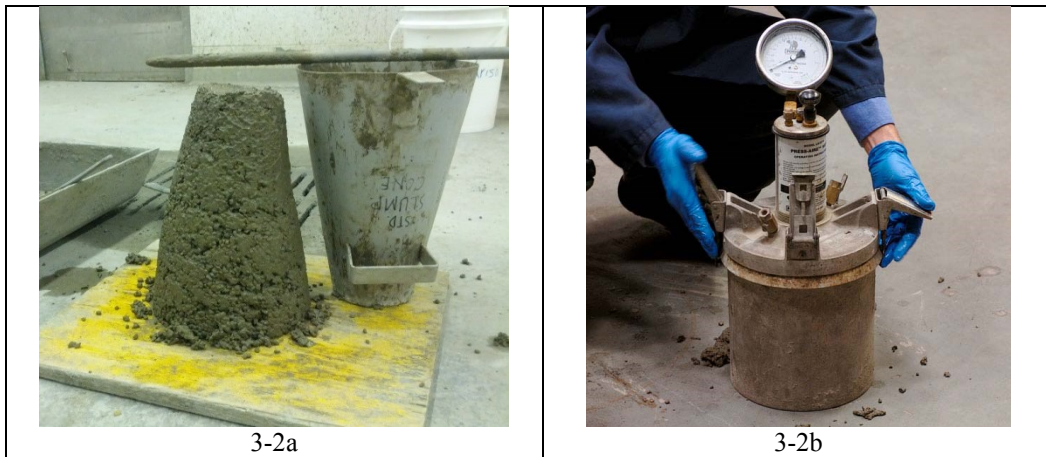
Figure 3-2- Slump Test and Air Content Test
