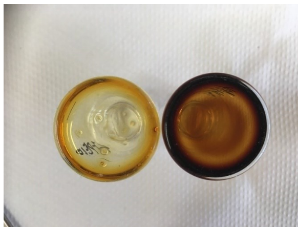
Figure 3.14. the appearance of polyester before(left) and after isomerization (right).
