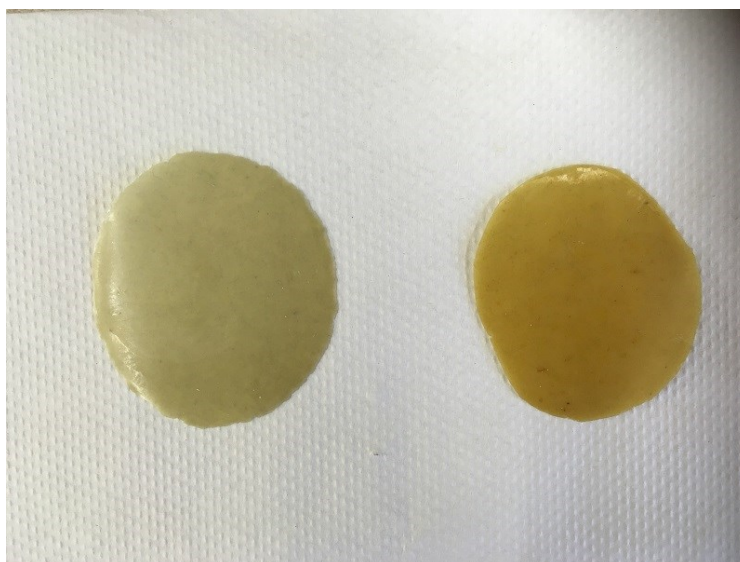
Figure 2.16. Films of polyester from conventional heating (left) and coupled methods (right).
