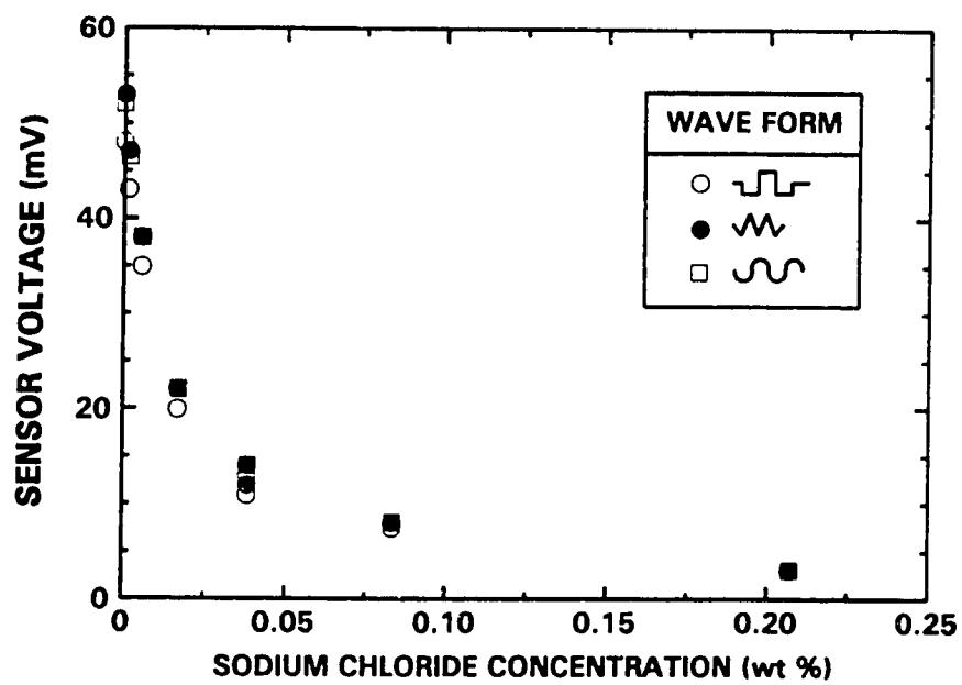
Figure 4.28: Effect of Field Waveform on the Conductivity Probe Sensor Voltage
