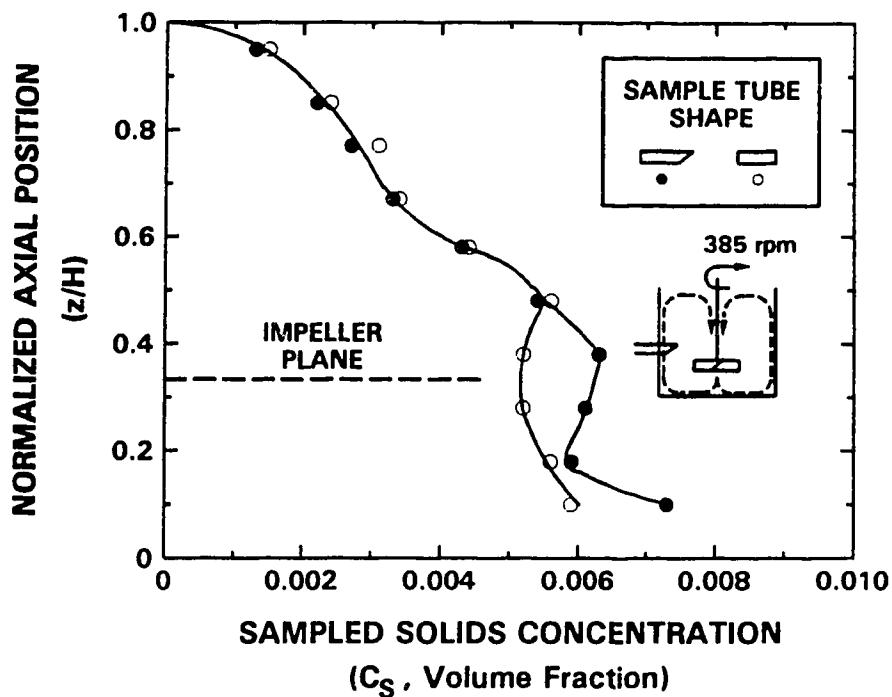
Figure 2.15: Effect of Sampler Shape on Solids Concentration Profiles in a Mixing Tank. Adapted From: Barresi and Baldi (1987a)
