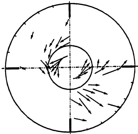
Figure 4.39: Radial-Angular Velocity Field in a Mixing Tank
