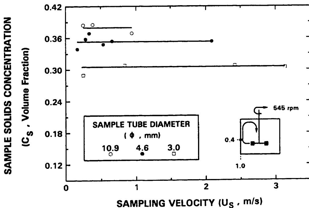
Figure 4.5: Effect of Sampler Diameter on Sample Concentration
