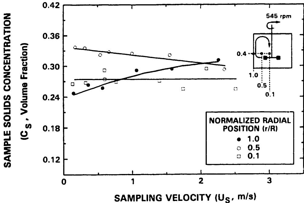
Figure 4.2: Effect of Radial Position on Sample Concentration
