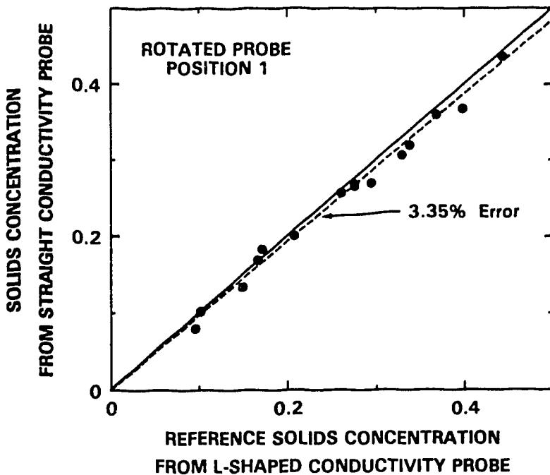
Figure 4.35: Conductivity Probe Calibration Curve from the Slurry Pipeline
