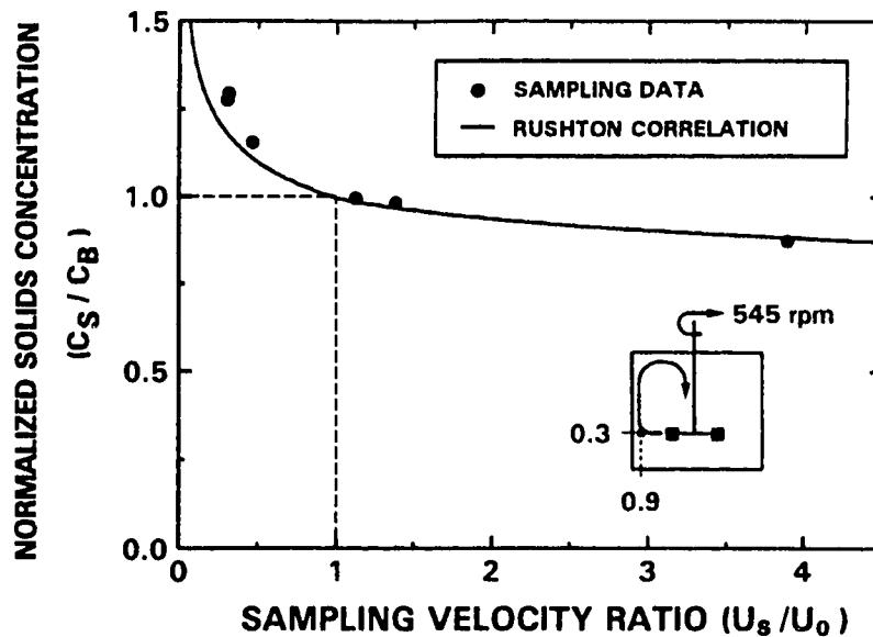
Figure 4.51 Comparison of the Rushton Correlation with Sampling Data
