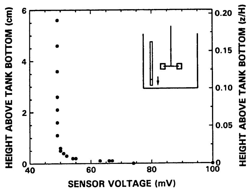
Figure 4.21: Effect of Approaching the Plexiglas Bottom on the Conductivity Probe Sensor Voltage
