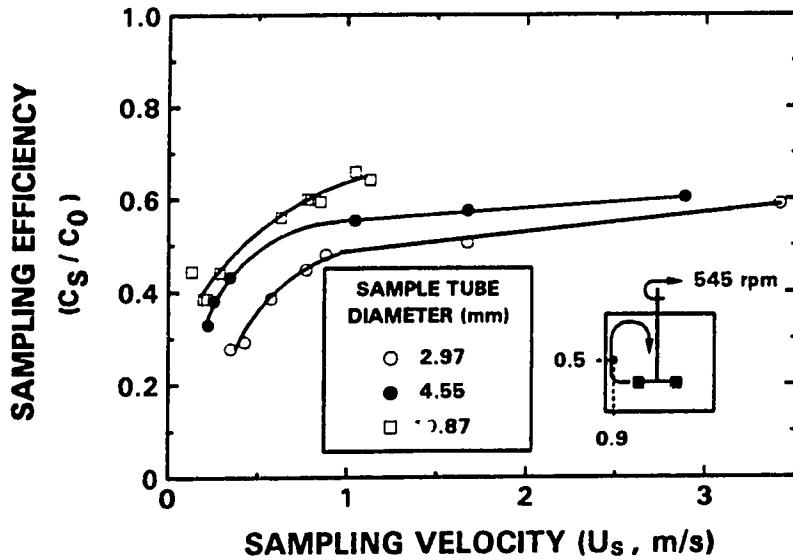
Figure 4.48 Effect of Sample Tube Diameter on Sampling Efficiency in the Mixing Tank
