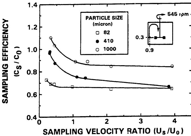
Figure 4.42: Effect of Particle Size on Sampling Efficiency on the Impeller Plane (Tapered Sample Tube)
