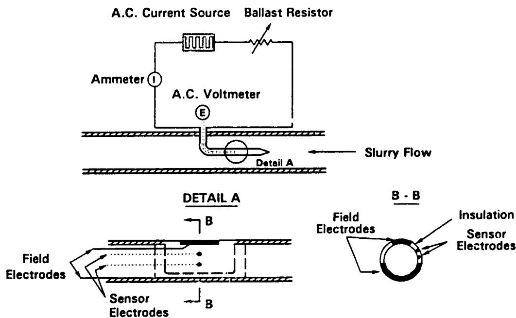
Figure 2.21: Four Electrode Conductivity Probe for a Slurry Pipeline
