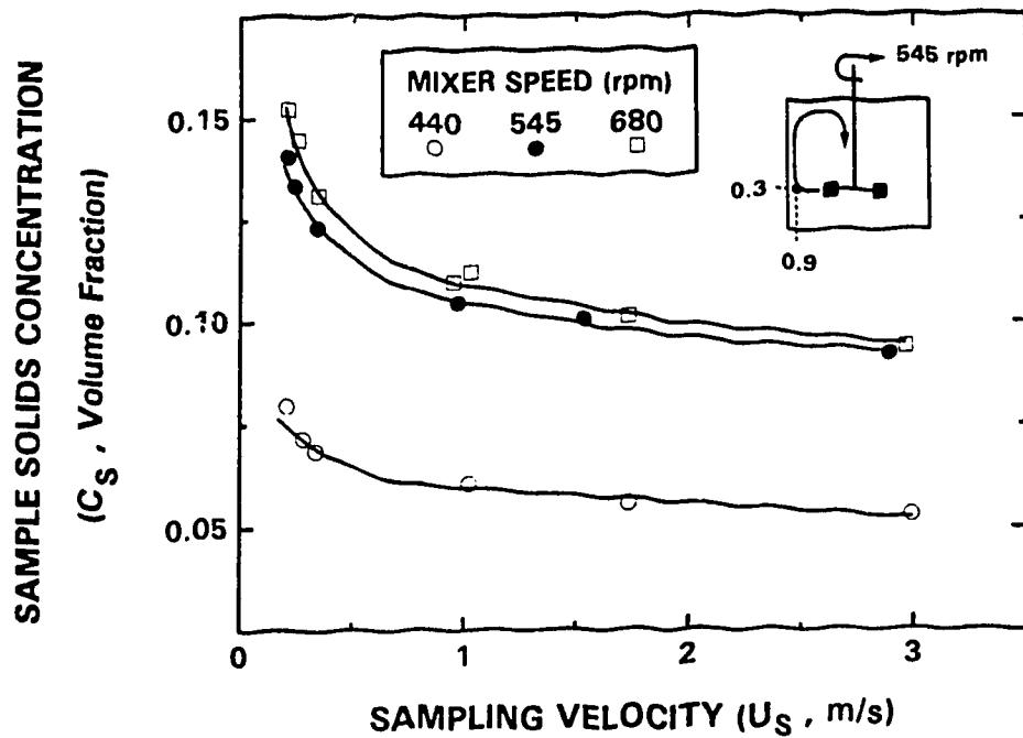
Figure 4.7: Effect of Mixer Speed on Sample Concentration
