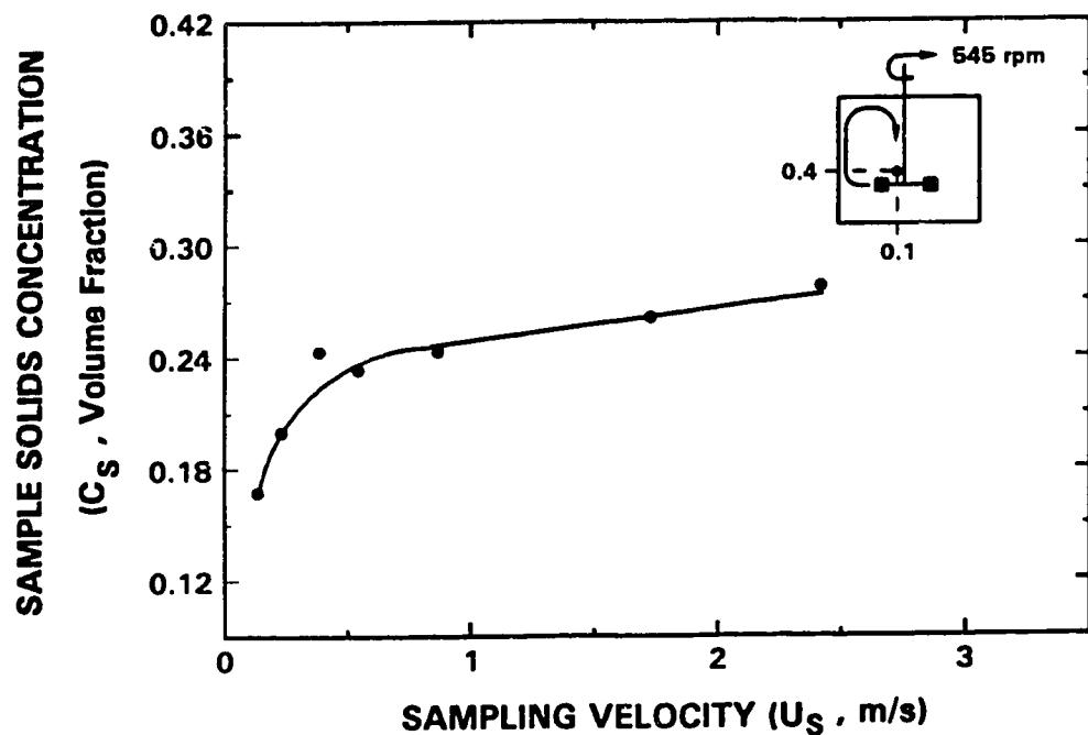
Figure 4.1: Sample Solids Concentration versus Sampling Velocity
