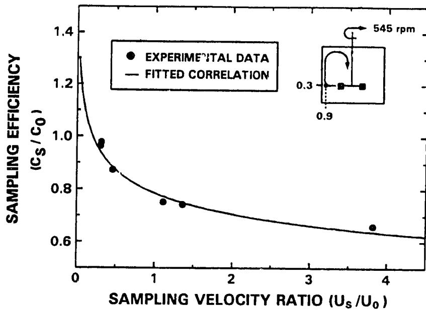
Figure 4.53: Curve Fitted To Sampling Efficiency Data From the Mixing Tank
