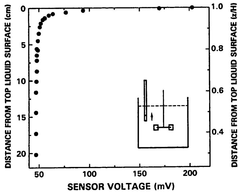
Figure 4.26: Effect of Approaching the Top Liquid Surface on the Conductivity Probe Sensor Voltage
