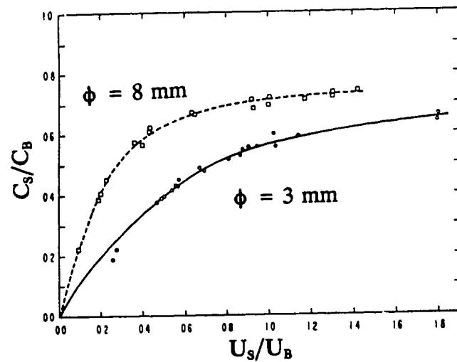
Figure 2.9: Effect of Sample Tube Diameter on Sampling Efficiency for Side Wall Sampling from a Vertical Slurry Pipeline
