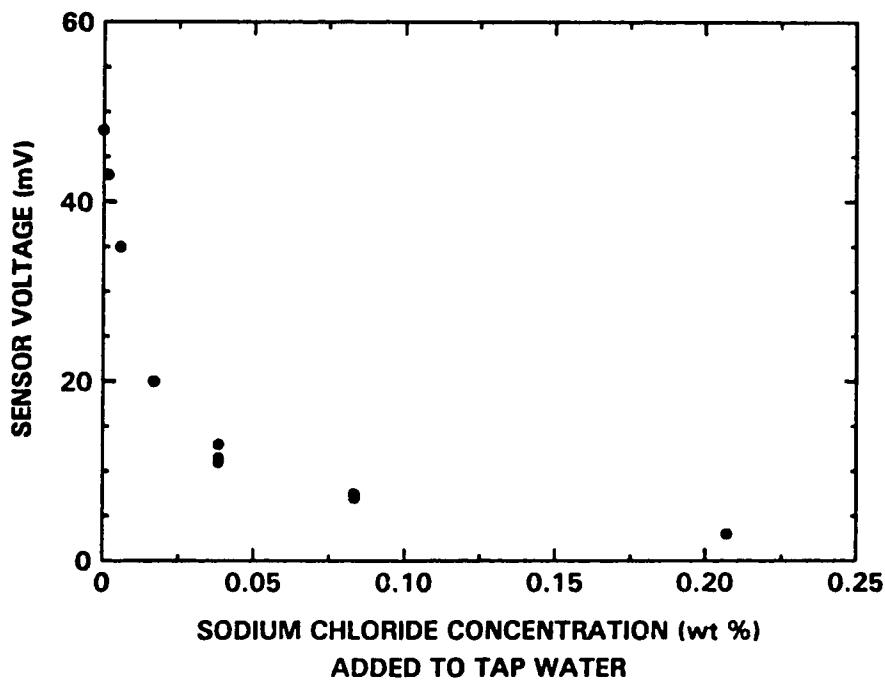
Figure 4.16: Effect of NaCl Concentration on the Conductivity Probe Sensor Voltage
