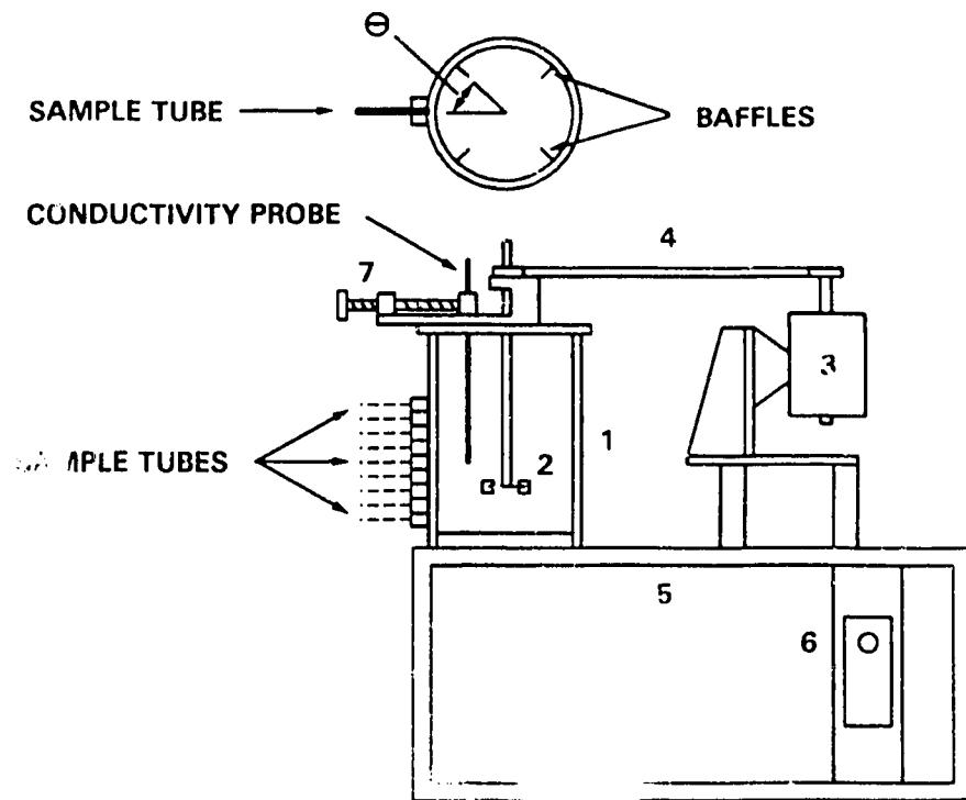
Figure 3.1: Mixing Tank Schematic
