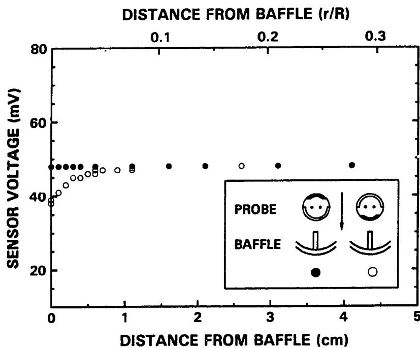
Figure 4.24: Effect of Approaching a Baffle on the Conductivity Probe Sensor Voltage
