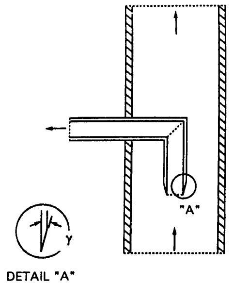
**Figure 2.3:** L-Shaped Sampling Probe in a Vertical Slurry Pipeline
