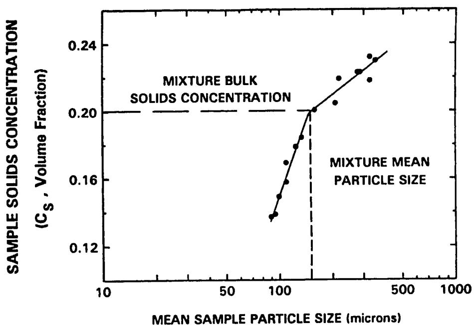
Figure 4.14: Sample Mean Particle Size versus Sample Solids Concentration
