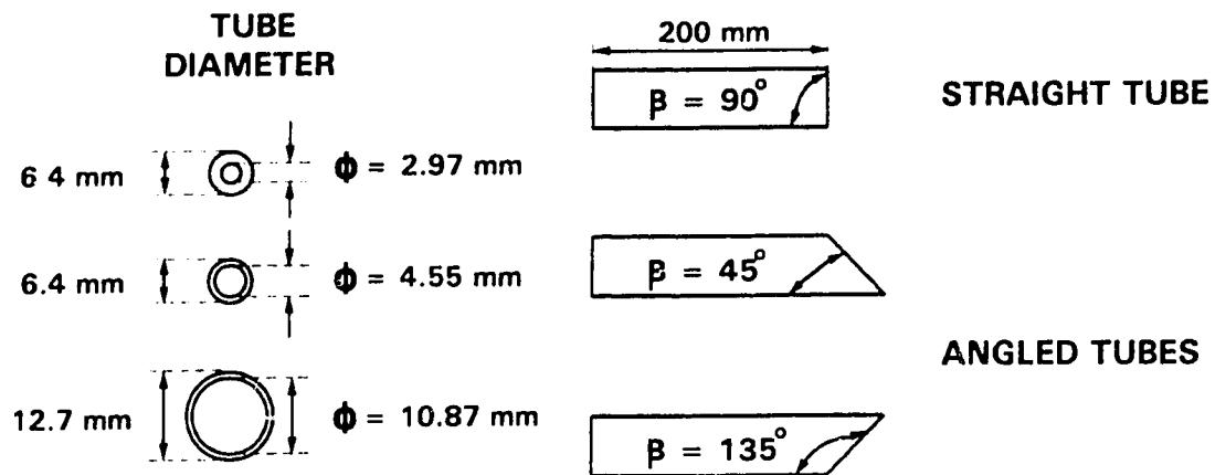
Figure 3.5: Sample Tube Dimensions
