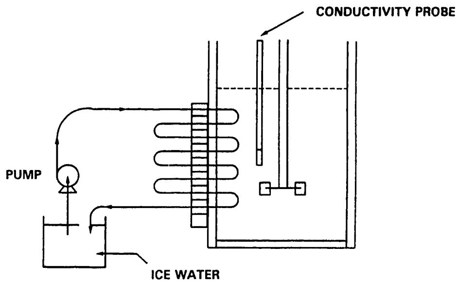
Figure 4.17: Mixing Tank Heat Exchanger System
