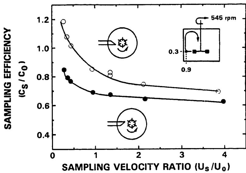
Figure 4.40: Effect of Lateral Sampler Orientation on the Sample Quality on the Impeller Plane.
