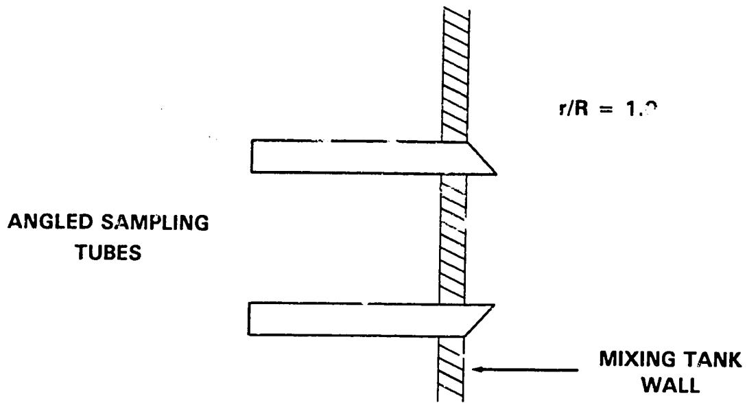
Figure 3.6: Angled Sample Tube Radial Position
