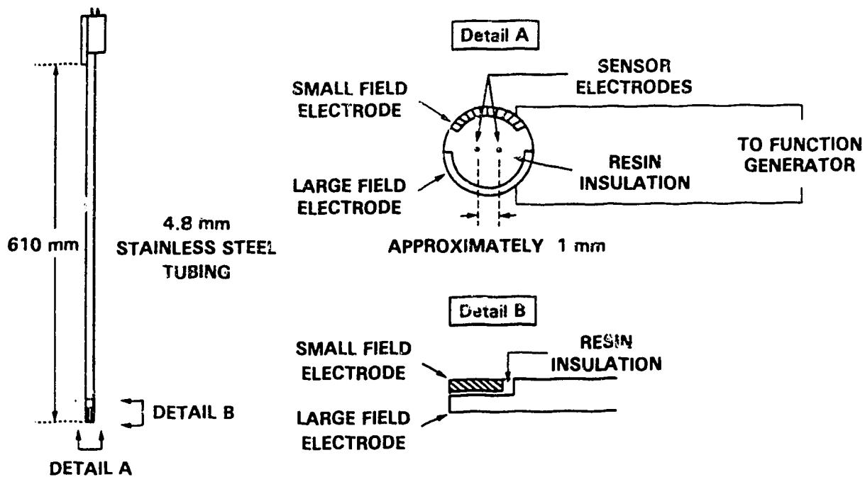
Figure 3.8: Conductivity Probe Schematic
