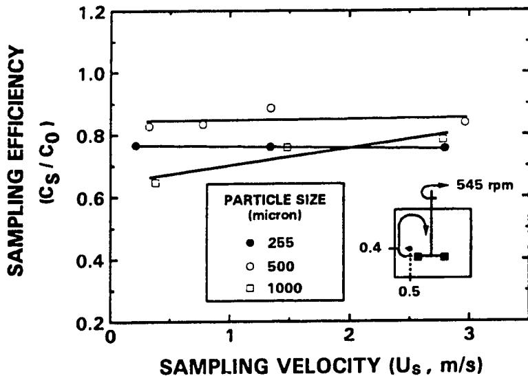
Figure 4.44 Effect of Particle Size on Sampling Efficiency for Mixed Flow in the Mixing Tank
