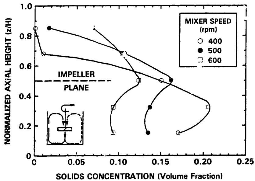
Figure 2.19: Mixing Tank Solids Concentration Profiles
