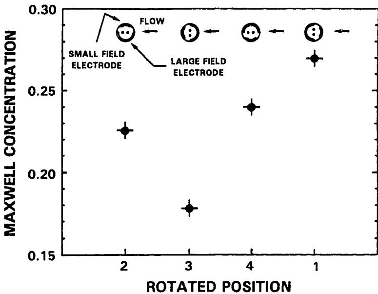
Figure 4.33: Effect of Probe Rotation on Measured Concentration in the Slurry Pipeline
