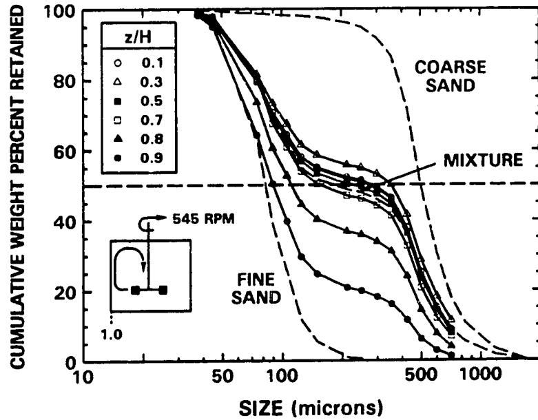
Figure 4.13: Variation of Particle Size Distribution with Axial Position
