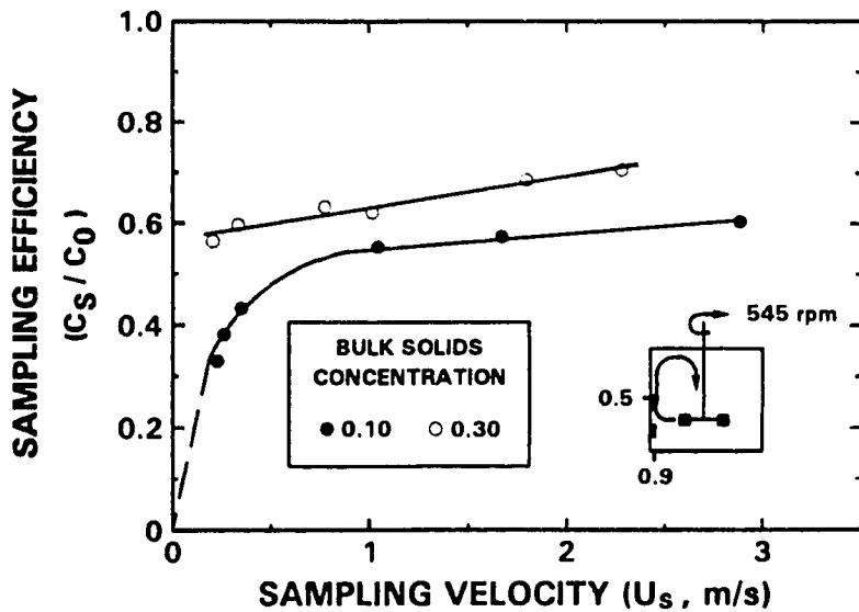
Figure 4.45 Effect of Bulk Solids Concentration on Sampling Efficiency for Sampling Perpendicular to the Flow in the Mixing Tank
