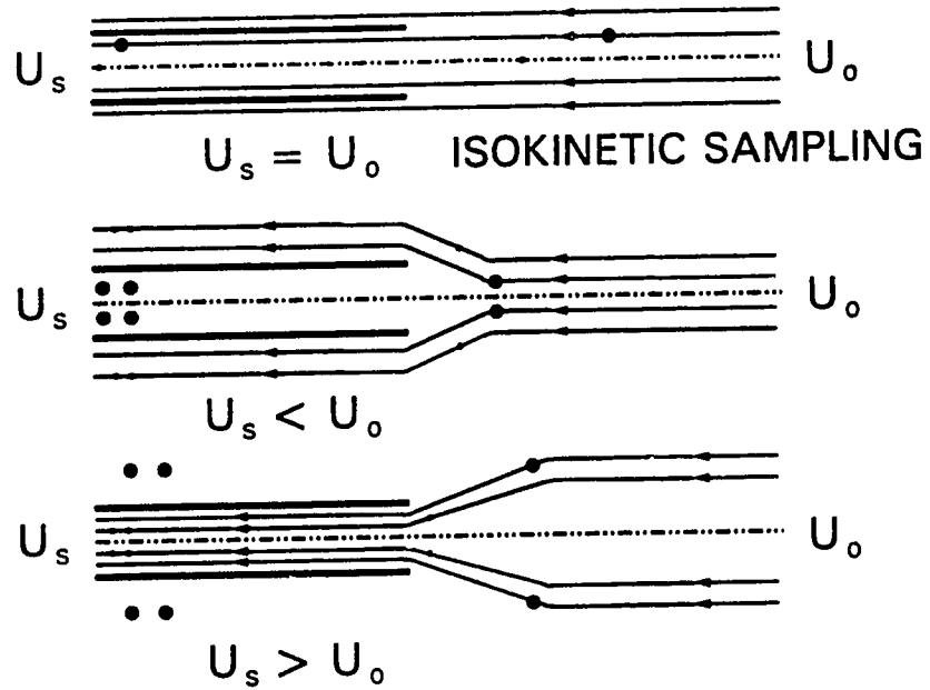
**Figure 2.4:** Flow Streamlines Ahead of a Sampler
