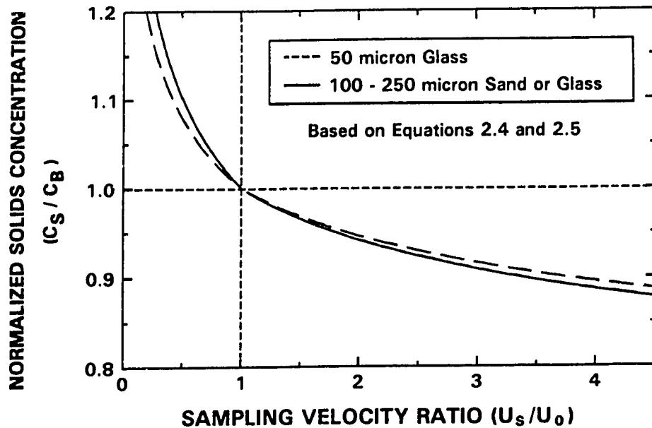
Figure 2.14: Effect of Particle Size on Sample Concentration From the Impeller Plane of a Mixing Tank
