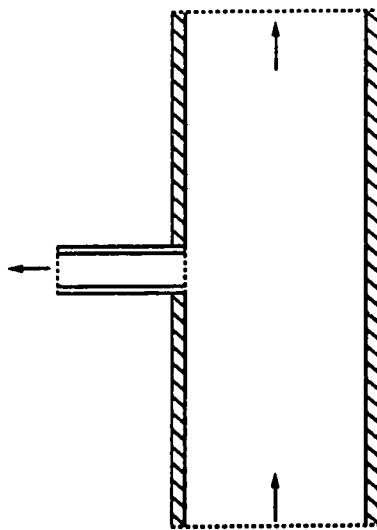
Figure 2.7: Side-Wall Sampling from a Vertical Slurry Pipeline
