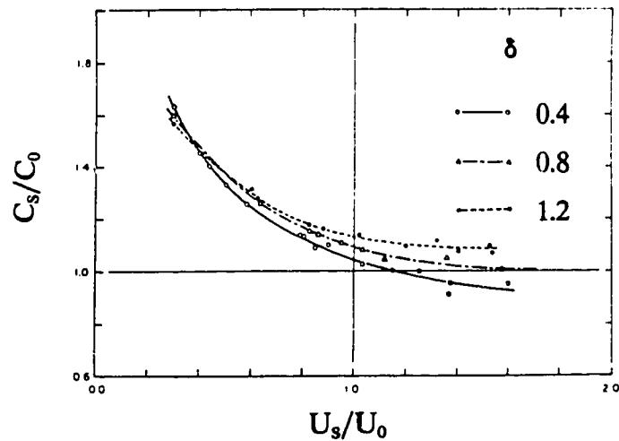
**Figure 2.6:** Effect of Probe Wall Thickness on Sampling Efficiency
