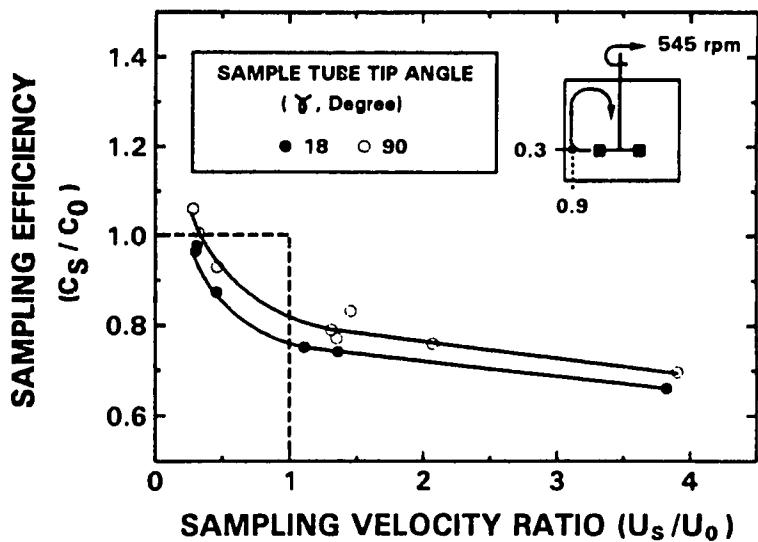
Figure 4.46 Effect of Sampler Tip Angle when Sampling Parallel to the Flow in the Mixing Tank  $d_{50} = 410 \mu m$ ,  $C_B = 0.10$ ,  $\phi = 4.6$  mm,  $\beta = 90^\circ$ ,  $\delta = 0.4$ ,  $z/H = 0.3$ ,  $r/R = 0.9$
