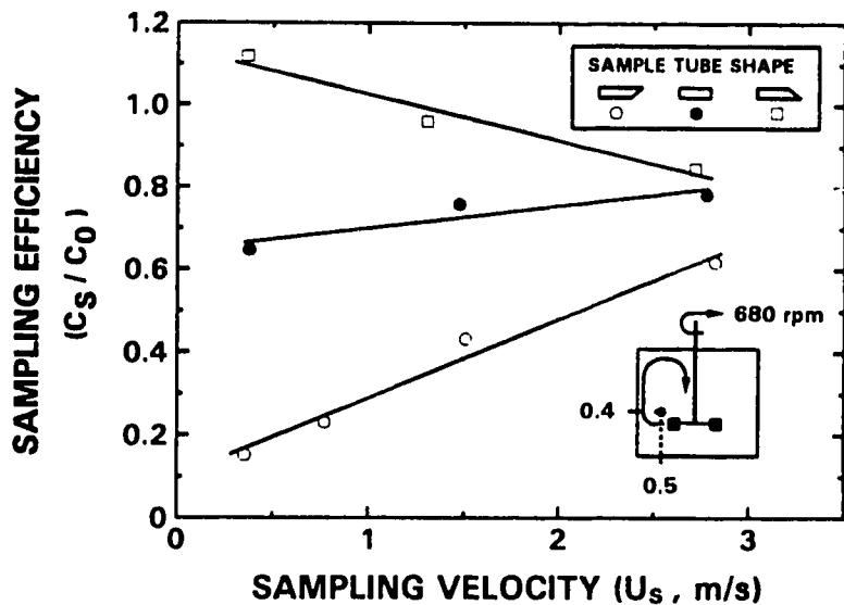
**Figure 4.50 Effect of Sampler Shape on Sampling Efficiency in the Mixing Tank**
