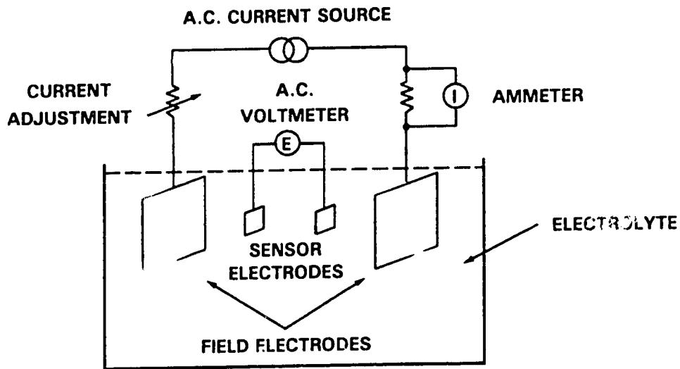
Figure 2.22: Four-Electrode Conductivity Circuit Used by Considine and Considine (1985)
