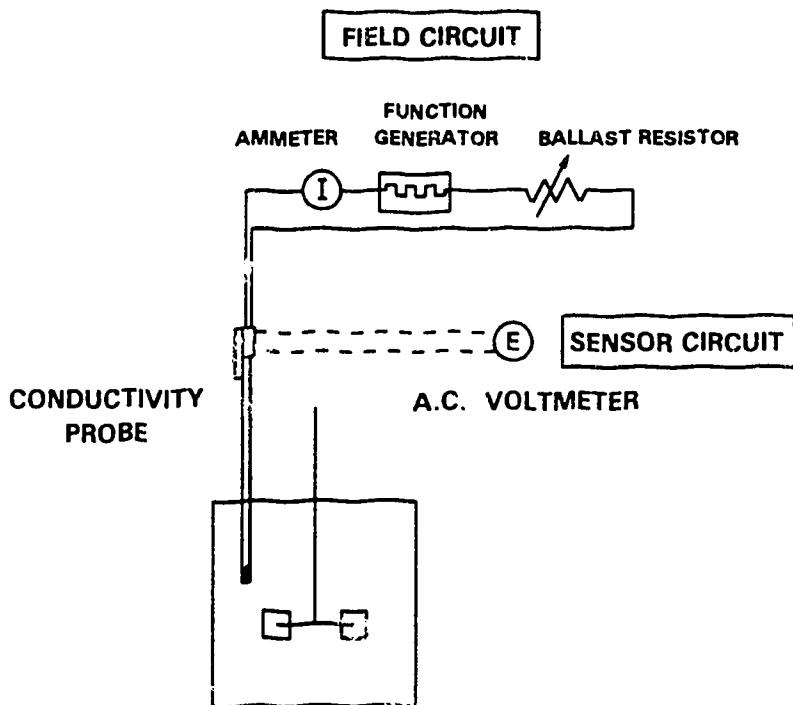
Figure 3.9: Conductivity Probe Circuit
