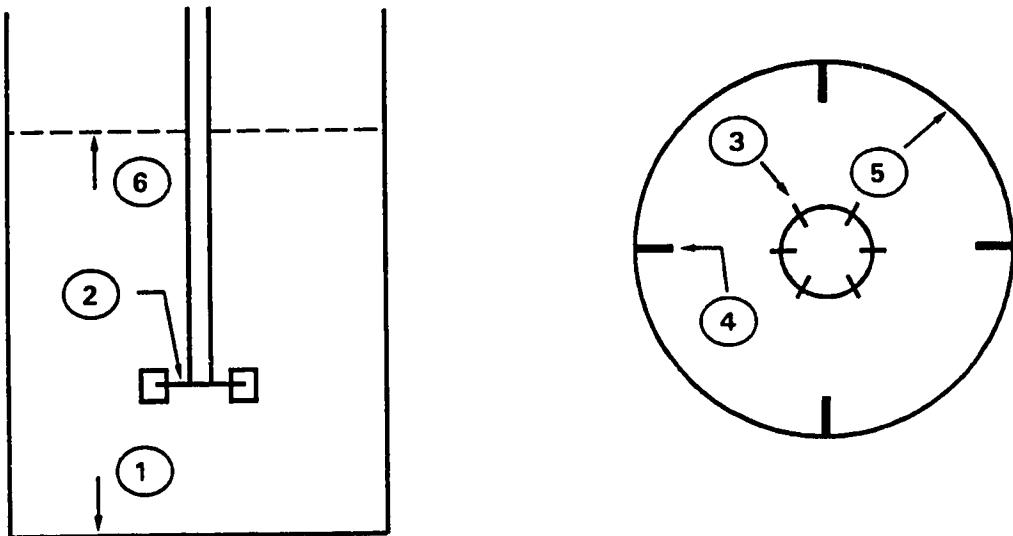
Figure 4.20: Mixing Tank Boundaries Approached by the Conductivity Probe
