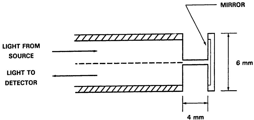
**Figure 2.17: Light Transmission Probe**
