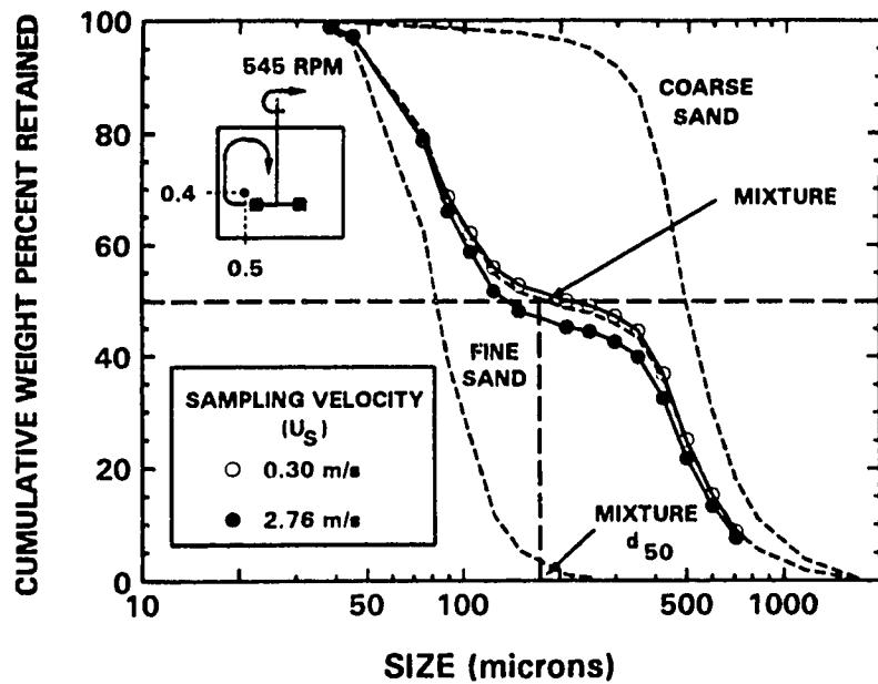
Figure 4.10: Effect of Sampling Velocity on Sample Particle Size Distribution (Runs 814 and 816)
