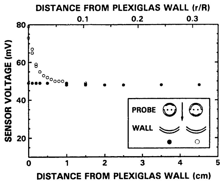
Figure 4.25: Effect of Approaching the Plexiglas Wall on the Conductivity Probe Sensor Voltage
