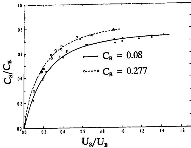
Figure 2.8: Effect of Sampling Velocity and Bulk Solids Concentration on Sampling Efficiency for Side-Wall Samplers
