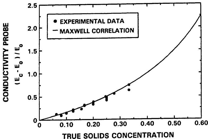
Figure 4.36: Conductivity Probe Calibration Curve from Sedimentation Experiments
