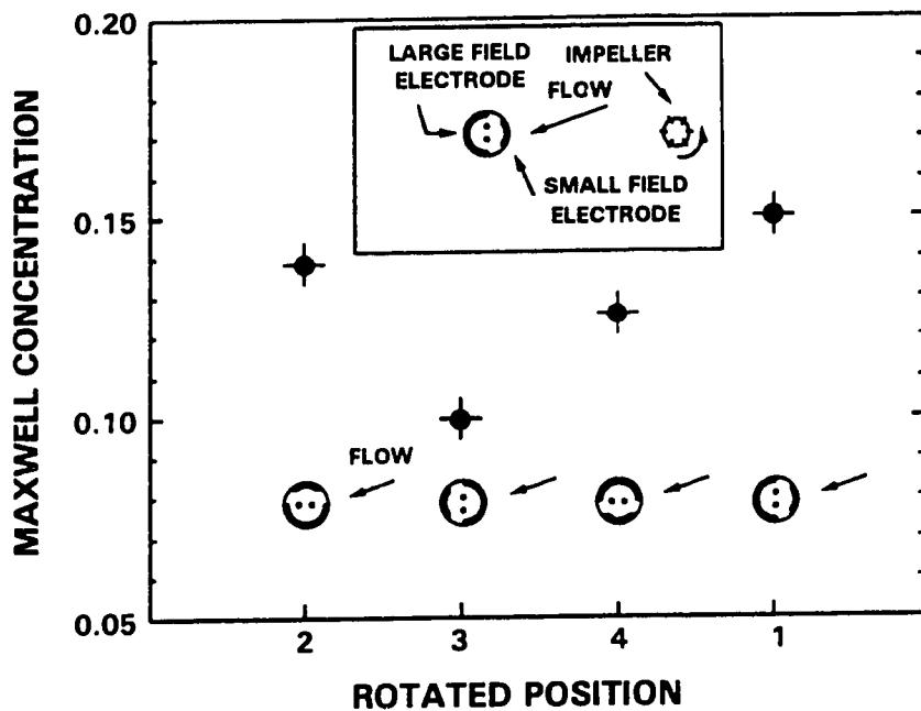
Figure 4.31: Effect of Probe Rotation on Measured Solids Concentration in the Mixing Tank (With Slurry)
