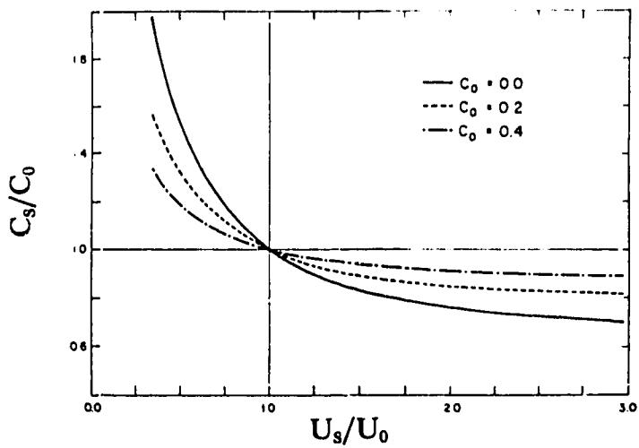
**Figure 2.5:** Effect of Solids Concentration on L-Shaped Probe Sampling Efficiency
