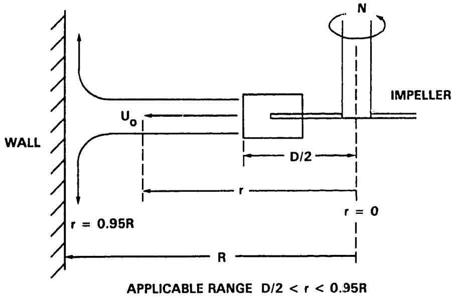
Figure 2.13: Radial Velocity From a Radial Flow Impeller
