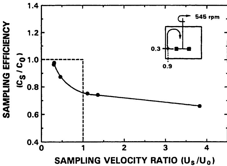
Figure 4.38: Sampling Efficiency on the Impeller Plane (Tapered Sample Tube)
