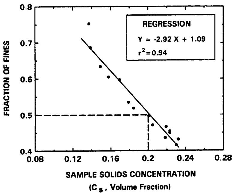
Figure 4.15: Sample Fines Fraction versus Sample Solids Concentration
