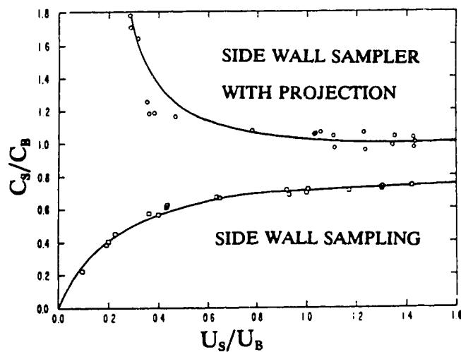
Figure 2.12: Sampling Efficiency of Side-Wall Samplers With and Without a Projection. Adapted From: Nasr-El-Din (1989)
