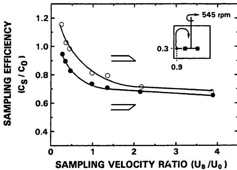
Figure 4.41: Effect of Vertical Sampler Orientation on the Sample Quality on the Impeller Plane
