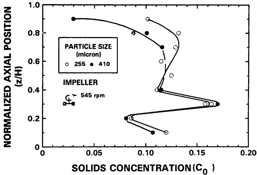
Figure 4.37: Mixing Tank Solids Concentration Profiles Measured with the Conductivity Probe ( $r/R = 0.6$ ,  $C_B = 0.10$ )
