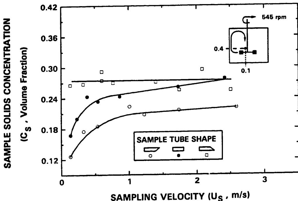
Figure 4.4: Effect of Sampler Shape on Sample Concentration
