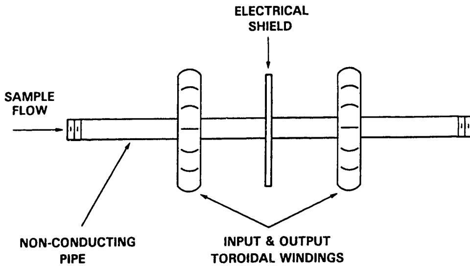
Figure 2.2: Electrodeless Conductivity Cell
