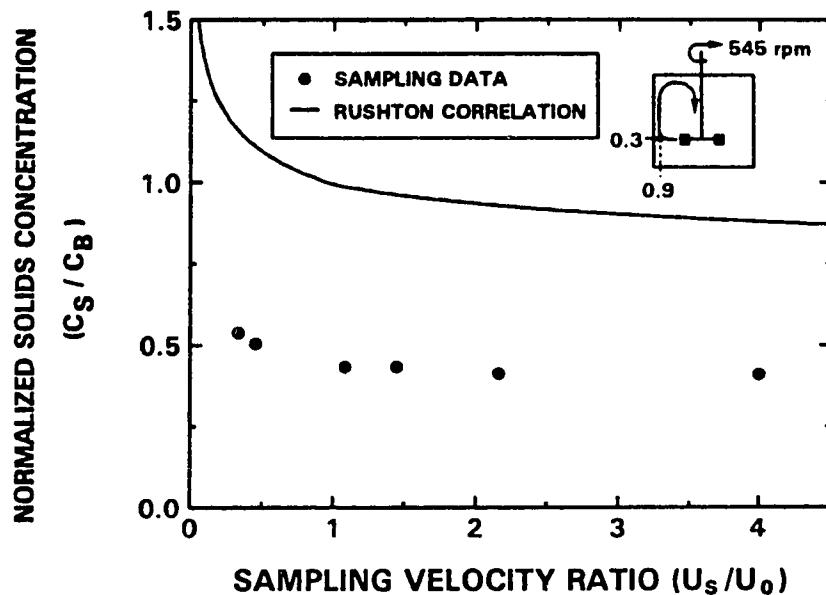
Figure 4.52 Comparison of the Rushton Correlation with Sampling Data
