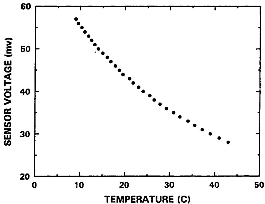
Figure 4.18: Effect of Temperature on the Conductivity Probe Sensor Voltage
