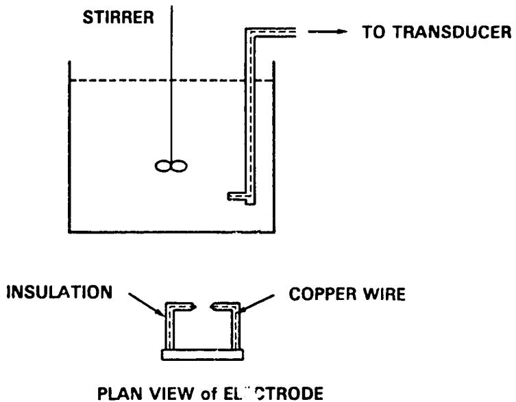
Figure 2.20: Conductivity Probe for a Mixing Tank
