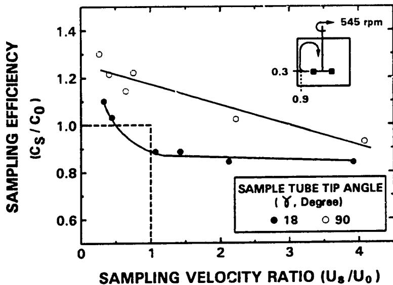
Figure 4.47 Effect of Sampler Tip Angle when Sampling Parallel to the Flow in the Mixing Tank  $d_{50} = 1000 \mu m$ ,  $C_B = 0.10$ ,  $\phi = 4.6$  mm,  $\beta = 90^\circ$ ,  $\delta = 0.4$ ,  $z/H = 0.3$ ,  $r/R = 0.9$
