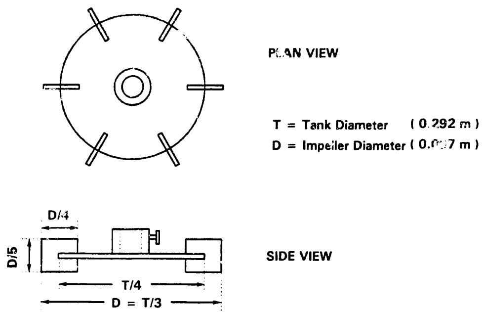
Figure 3.3: Radial Flow Impeller
