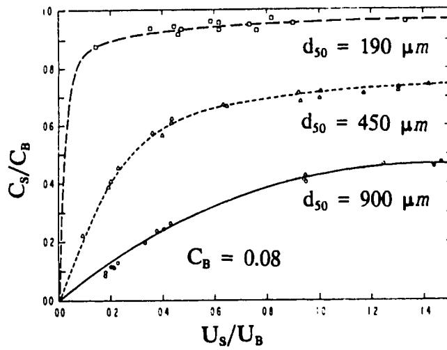
Figure 2.10: Effect of Particle Size on Sampling Efficiency for Wall Sampling from a Vertical Slurry Pipeline
