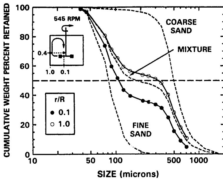
Figure 4.12: Variation of Particle Size Distribution with Radial Position
