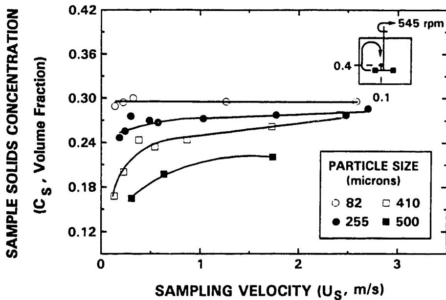
Figure 4.8: Effect of Particle Size on Sample Concentration
