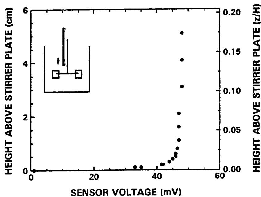
Figure 4.22: Effect of Approaching the Impeller Plate on the Conductivity Probe Sensor Voltage
