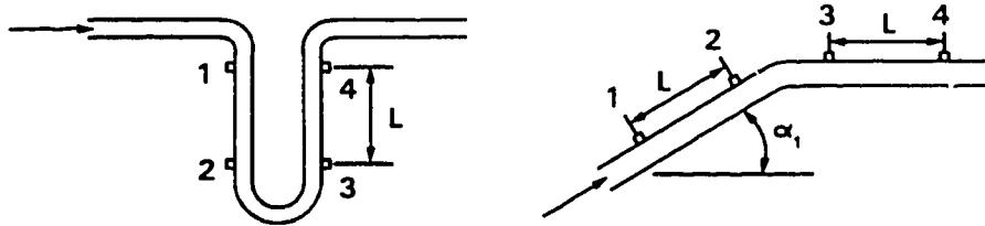
(A) VERTICAL COUNTERFLOW METER      (B) INCLINED PIPE CONCENTRATION METER
