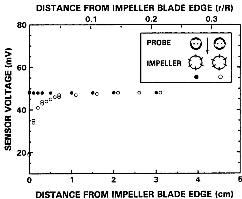
Figure 4.23: Effect of Approaching the Impeller Blade on the Conductivity Probe Sensor Voltage
