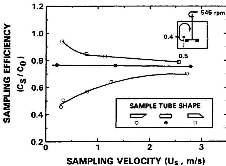
Figure 4.49 Effect of Sampler Shape on Sampling Efficiency in the Mixing Tank
