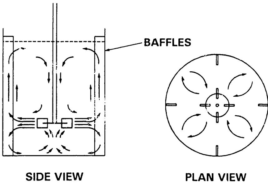
Figure 3.4: Typical Flow Patterns in a Mixing Tank Stirred with a Radial Flow Impeller
