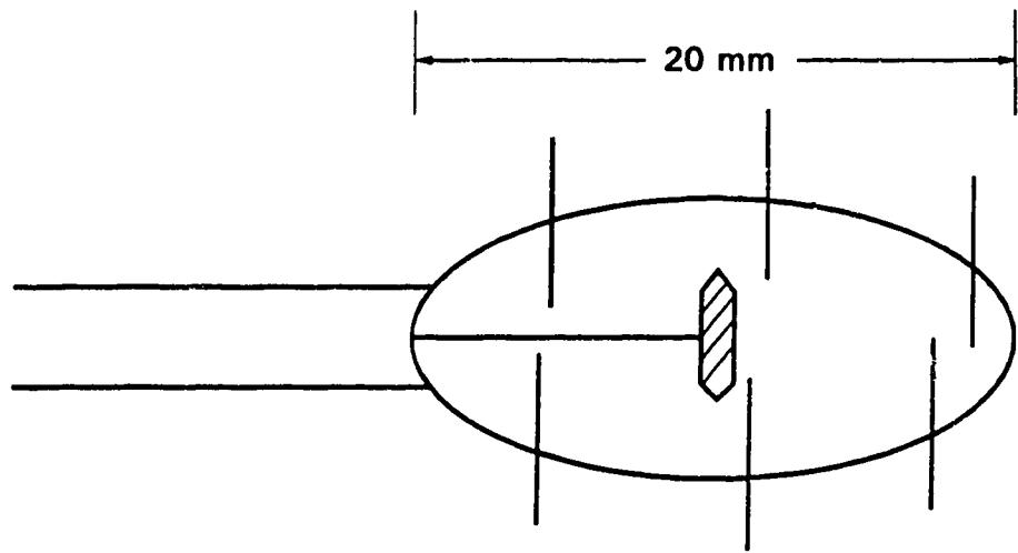
Figure 2.18: Conductivity Probe for Measuring Local Solids Concentration
