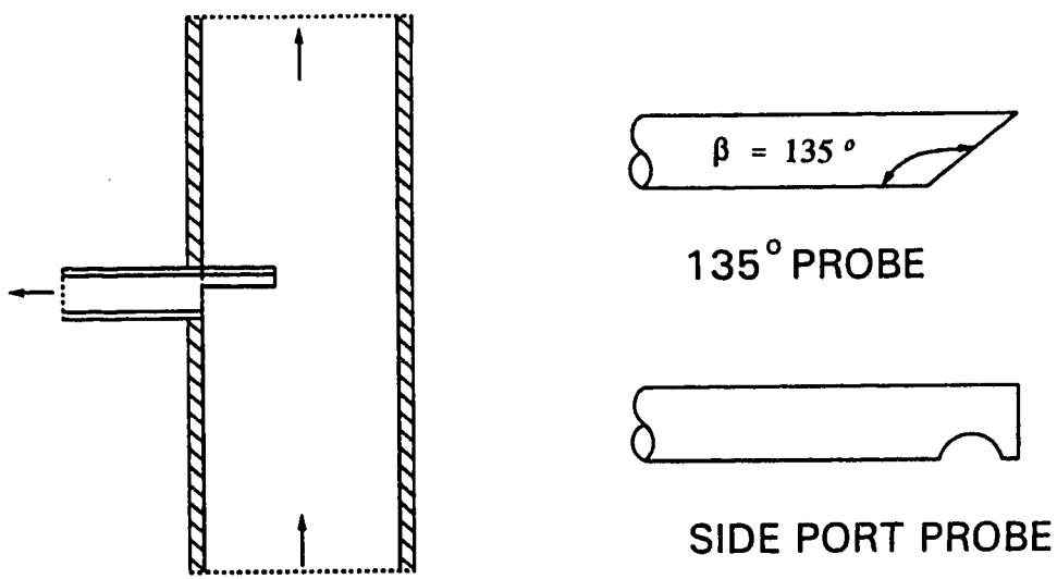
Figure 2.11: Side-Wall Samplers With a Projection
