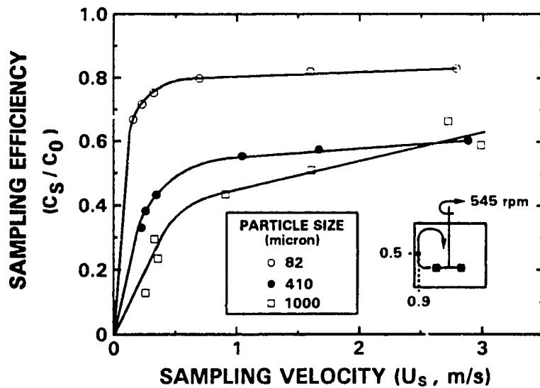
Figure 4.43: Effect of Particle Size on Sampling Efficiency with Flow Perpendicular to the Sample Tube in the Mixing Tank
