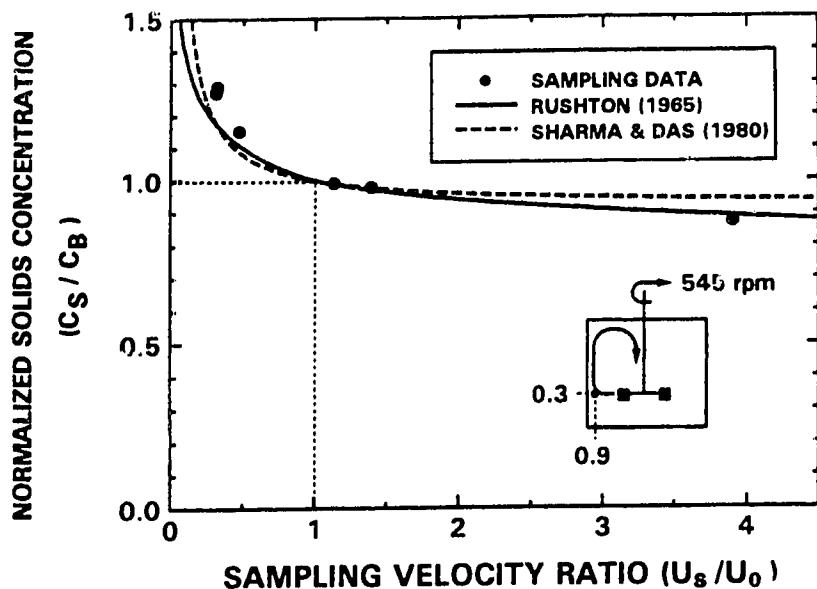
Figure 4.54: Comparison of the Rushton and Sharma and Das Correlations with Experimental Data
