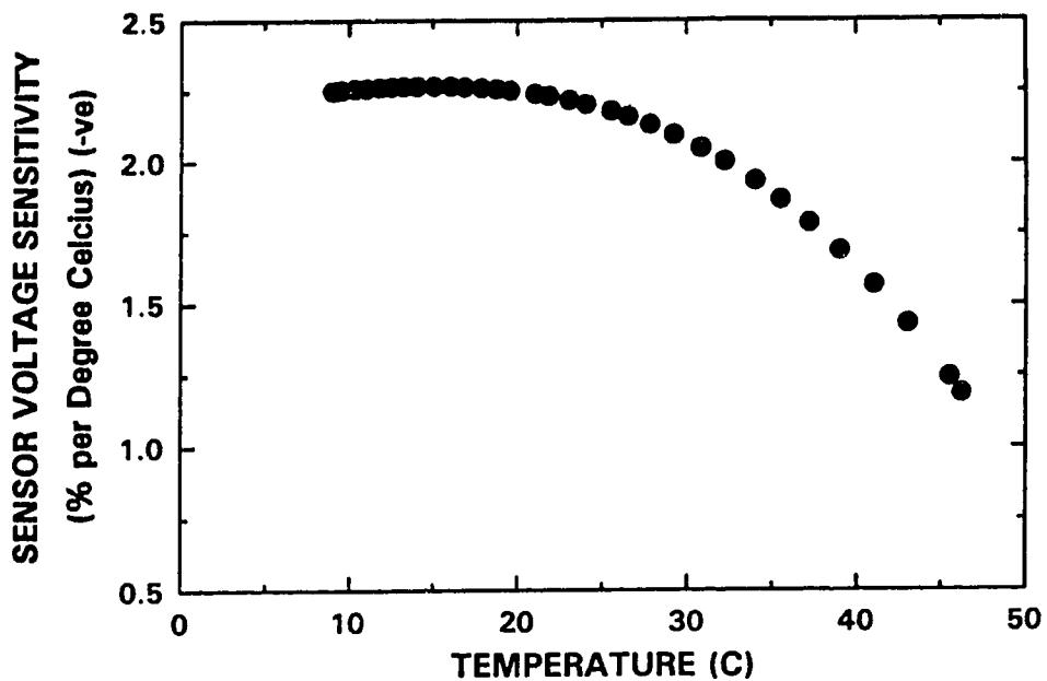
Figure 4.19: Sensitivity of Conductivity Probe Sensor Voltage to Temperature
