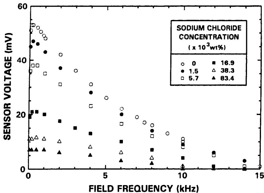
Figure 4.29: Effect of Field Frequency on the Conductivity Probe Sensor Voltage
