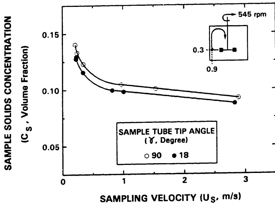
Figure 4.6: Effect of Sampler Tip Angle on Sample Concentration
