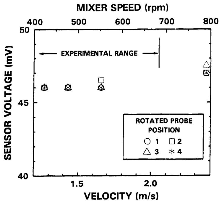
Figure 4.34: Effect of Probe Rotation on the Conductivity Probe Sensor Voltage in the Mixing Tank (Water Only) ( $z/H = 0.3$ ,  $r/R = 0.4$ )
