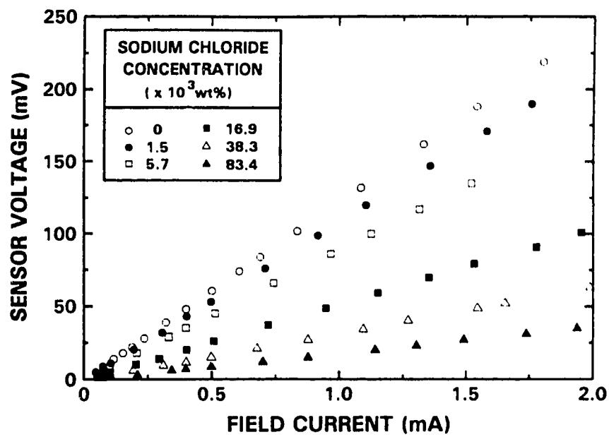
Figure 4.27: Effect of Field Current on the Conductivity Probe Sensor Voltage
