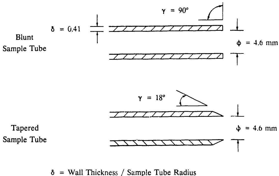
Figure 3.1: Sample Tube Tip Angle
