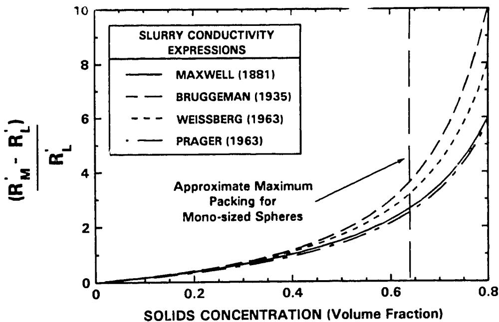
Figure 2.23: Slurry Electrical Conductivity Expressions
