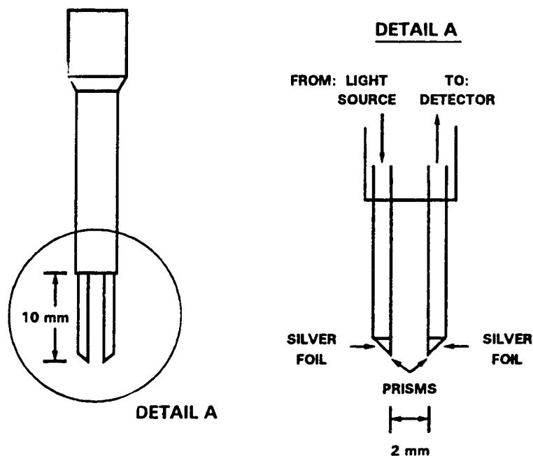
Figure 2.16: Light Transmission Probe
