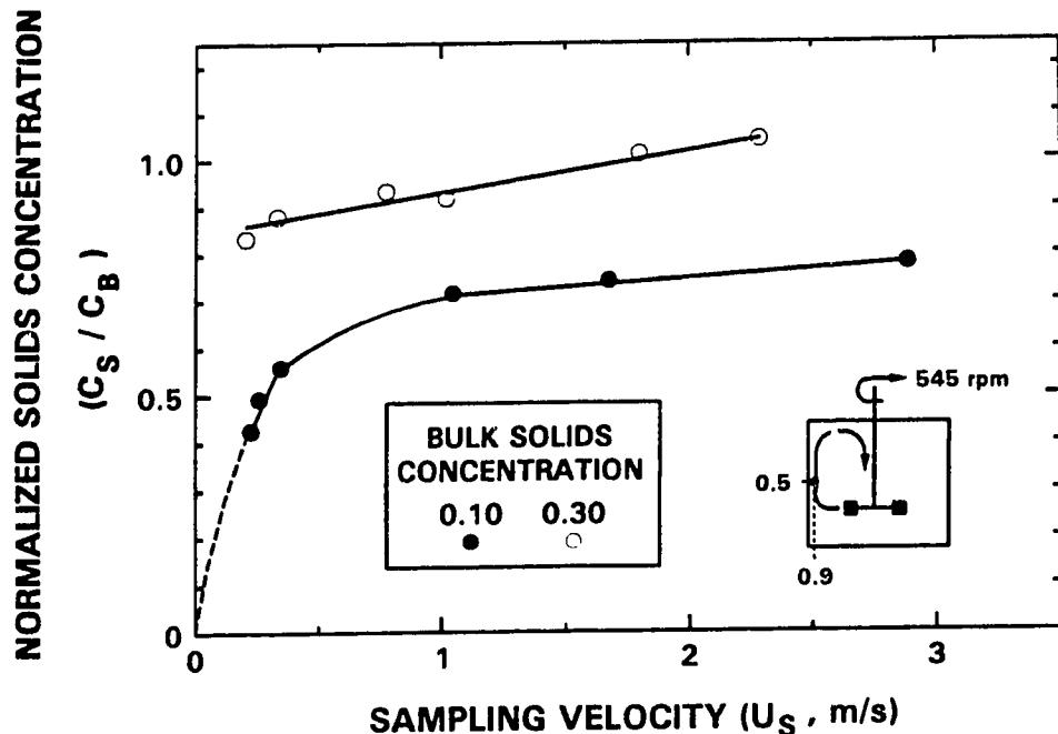
Figure 4.9: Effect of Bulk Solids Concentration on Sample Concentration
