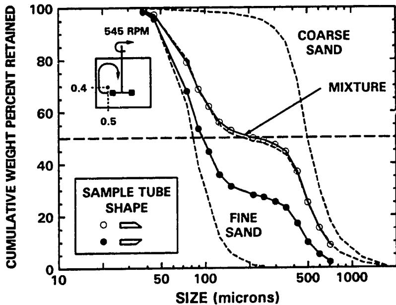
Figure 4.11: Effect of Sampler Shape on Sample Particle Size Distribution (Runs 813 and 814)
