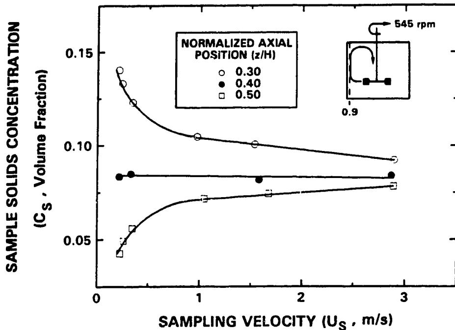
Figure 4.3: Effect of Axial Location on Sample Concentration
