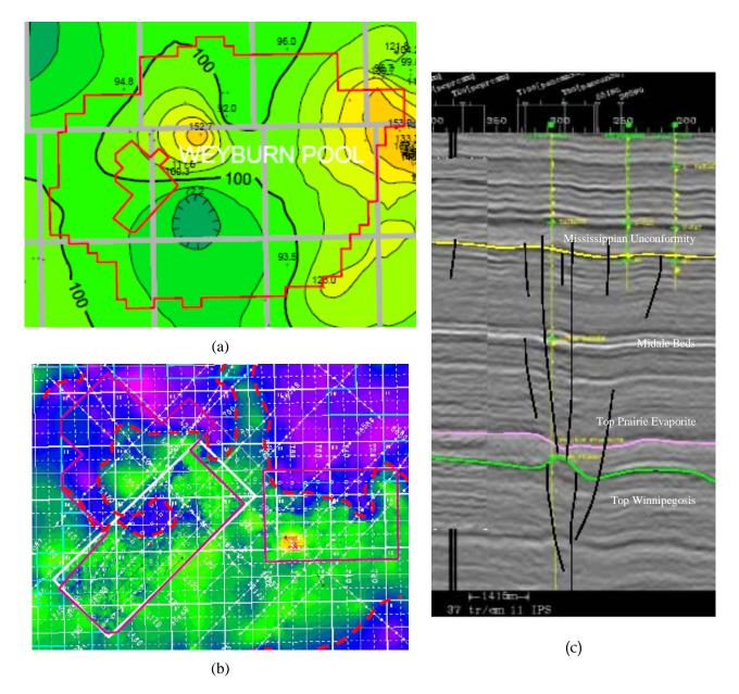
Figure 9-2. (a) Minor salt dissolution feature east of Phase 1A, below Phase 1B. This feature has been observed in (b) seismic, and (c) there is a fault that pass by the dissolution zone, after Kreis [223], and Bunge [202]
