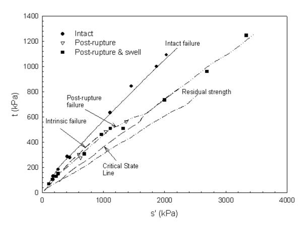
Figure 6-3. Intact, intrinsic and post-rupture failure envelopes as well as residual strength for Todi Clay, modified after Burland [116] and Burland et al. [129]
