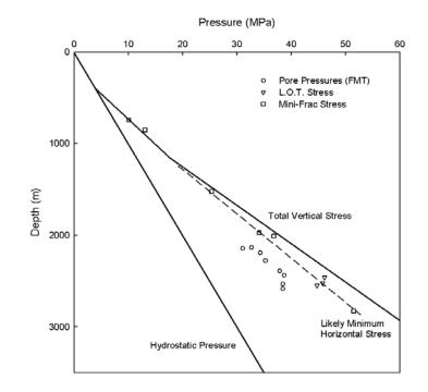
Figure 3-5 shows that the present pressures are about 82% of the vertical effective stress, which is about 90% of the fracture pressure from minifrac and leak-off tests, suggesting that leakage occurs through existing fractures instead of the formation of new ones [50]. Therefore, it appears there is a critical pressure at which these fractures open as flow channels.
