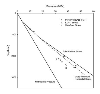
Figure 3-5. (a) Lithostratigraphy of the Viking Graben; and (b) Distribution of fluid pressures, minimum horizontal stress, and vertical stresses in the Snorre area, modified after Caillet [50]
