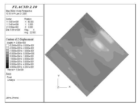
Figure B-41. Vertical displacement in the Lower Vuggy Formation.
