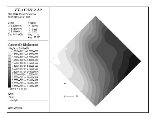
Figure B-28. West-East displacement in the Upper Vuggy Formation.
