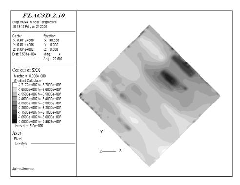
Figure B-6. West-East stresses in the Frobisher Evaporite Formation.
