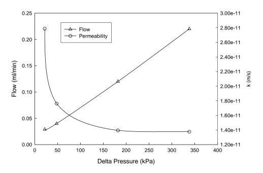
Figure 5-21. Average flow rates for different gradients, and permeability values measured. Notice how stable the measurements are once the flow is more than 0.05 ml/min
