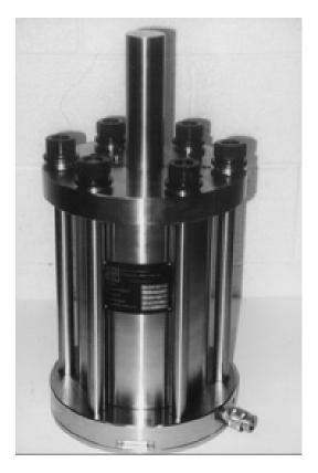
Figure 5-2. High-pressure, high-temperature triaxial cell. The cell is 70 cm tall
