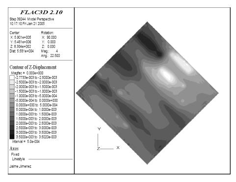
Figure B-39. Vertical displacement in the Marly Formation.
