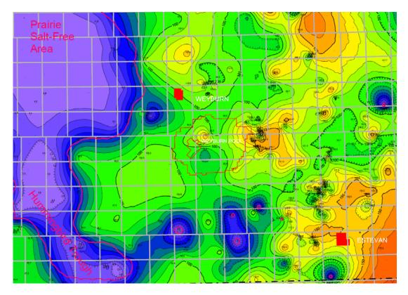
Figure 7-4. Areas of massive salt dissolution around the risk assessment area at Weyburn, after Kreis et al. [223]
