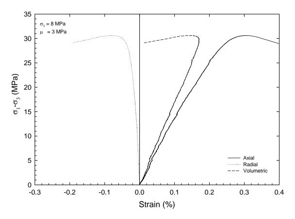
Figure 6-24. Test No. 2, triaxial compression of a Three Fingers sample carried out under a confining stress of 8 MPa and a pore pressure of 3 MPa
