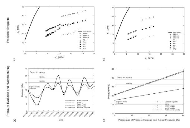
Figure 8-14. Stress results from the geomechanical models and pressure evolution. Plots (a), (c), (e), (g), (i), (k) illustrate pre-CO<sub>2</sub> injection results and plots (b), (d), (f), (h), (l) illustrate post-EOR CO<sub>2</sub> storage results where injection pressures have been elevated above operating pressures to test performance limits of caprock.
