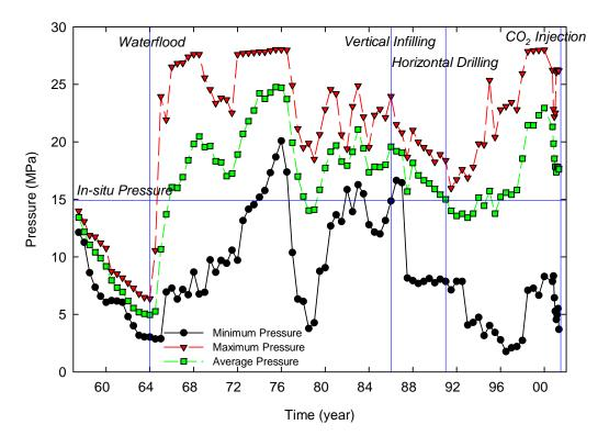
Figure 8-5. Reservoir pressure history at Phase 1A depicted through maximum, minimum and average pressure. Notice how the reservoir pressure has been maintained in average above the in-situ pressure since the waterflood
