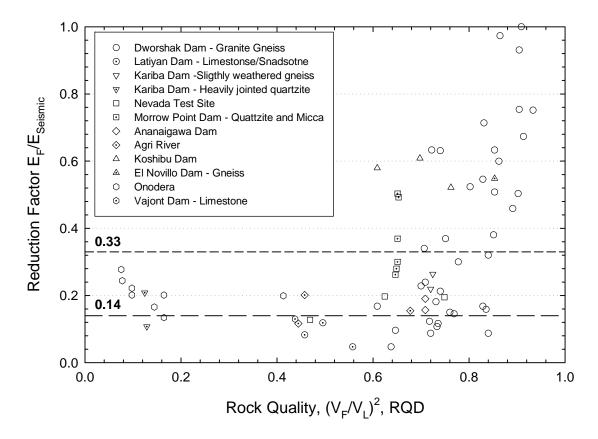
Figure 7-15. Variation of field over dynamic moduls against rock quality for dams built in different lithologies, modified after Deere [175]
