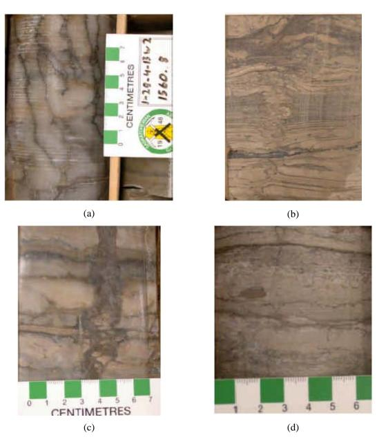
Figure 7-8. Fractures in the Midale Evaporite: (a) synsedimentary cracks, (b) dewatering fractures, (c) fracturing, and (d) long-elongated fractures; after Nickel [197]
