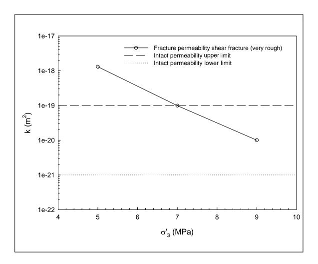
Figure 6-26. Test No. 2, permeability in the fractured Three Fingers sample compared with average intact values for anhydritic samples
