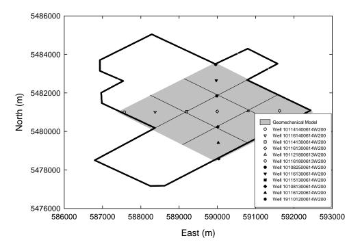
Figure 8-1. Nine-pattern spot at Phase 1A used for geomechanical modeling with the location of the wells used to track displacements
