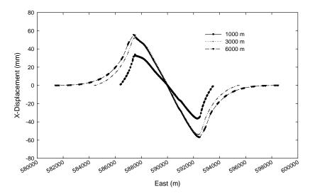
Figure 8-2. Displacements in the west-east direction for different "buffer zone" sizes. A buffer zone of 6 km was used for the geomechanical modeling as displacements were becoming insensitive to the size of the buffer
