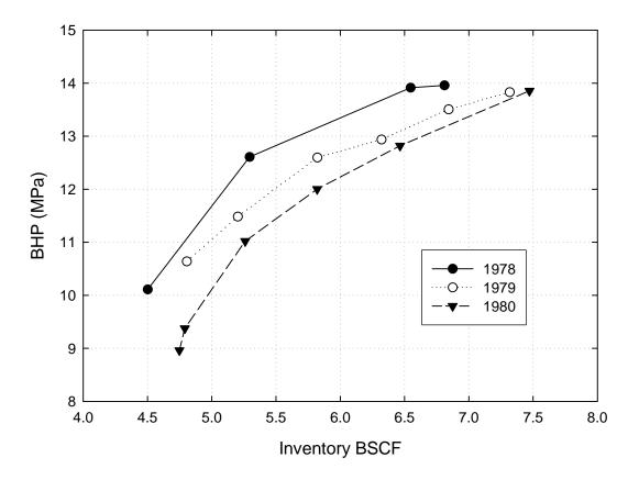
Figure 3-8. Injection curves for 1978, 1979, and 1980 in the Leroy Storage facility, modified after Araktingi et al. [56]
