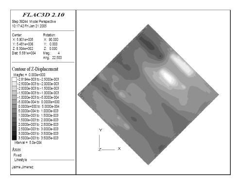
Figure B-40. Vertical displacement in the Upper Vuggy Formation.
