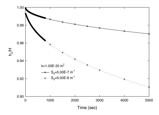
Figure 5-13. Upstream pressure decay for different values of specific storage
