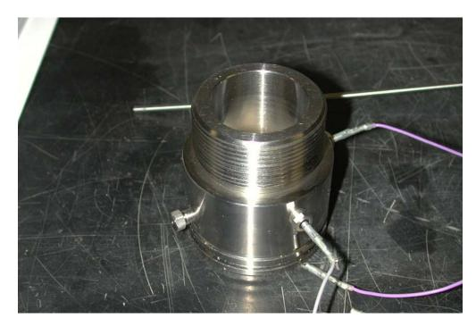
Figure 5-3. Detailed of the 2.5" (6.35 cm) platens. Notice the connectors for acoustic measurements
