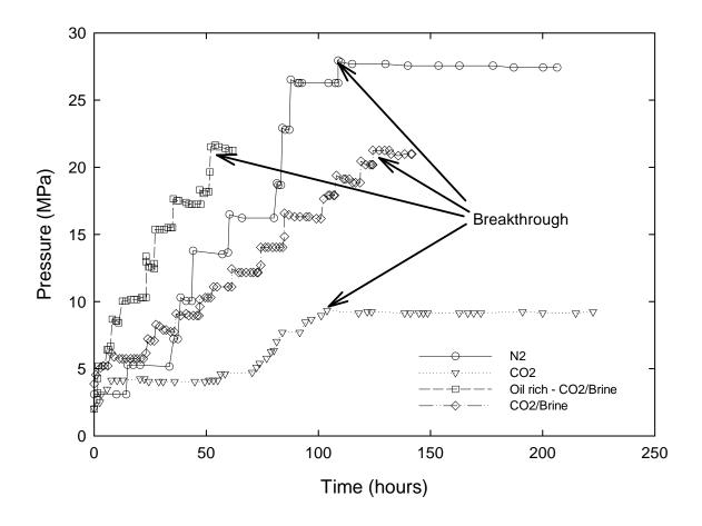
Figure 6-34. Breakthrough pressure test history from similar samples from Weyburn caprock samples using N<sub>2</sub>, pure CO<sub>2</sub>, oil-saturated CO<sub>2</sub>/brine system and pure CO<sub>2</sub>/brine system, modified after Dong et al. [70]
