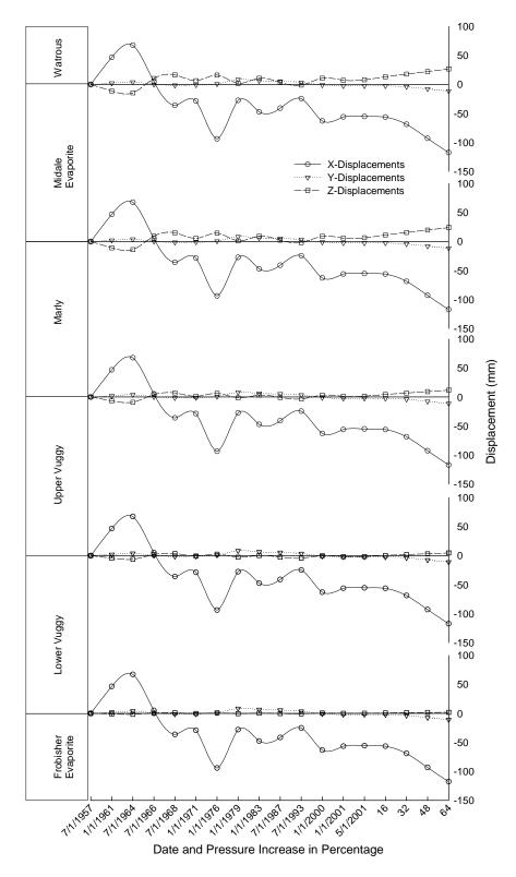
Figure 8-15. Displacements at every formation in the Well 101-14-14-006-14W200 (location shown in Figure 8-1) for the base case cenario.
