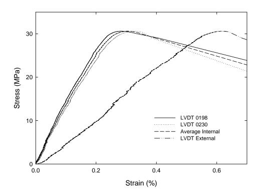
Figure 5-8. Contrast between internal and external LVDTs during an entire test
