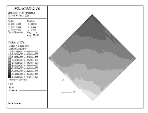
Figure B-14. Vertical stresses in the Midale Evaporite Formation.
