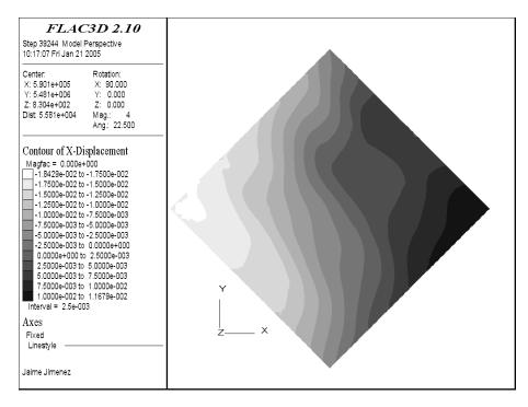
Figure B-27. West-East displacement in the Marly Formation.
