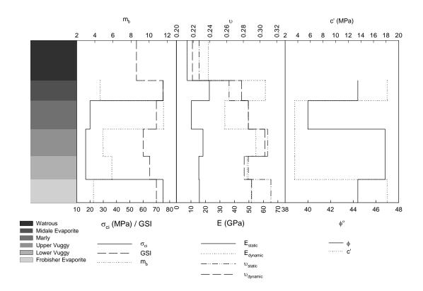
Figure 7-16. Elastic and mechanical properties of the caprock system at Weyburn, Phase 1A
