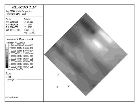
Figure B-38. Vertical displacement in the Midale Evaporite Formation.
