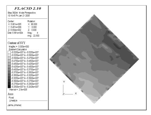
Figure B-8. North-south stresses in the Midale Evaporite Formation.
