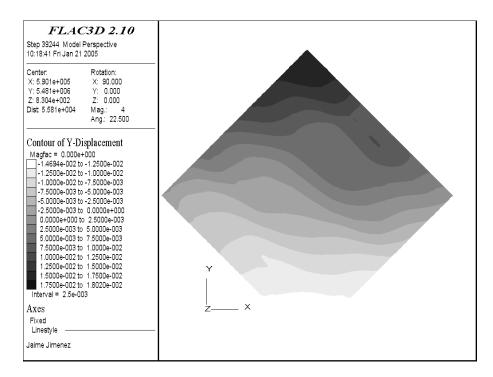
Figure B-36. North-South displacement in the Frobisher Evaporite Formation.
