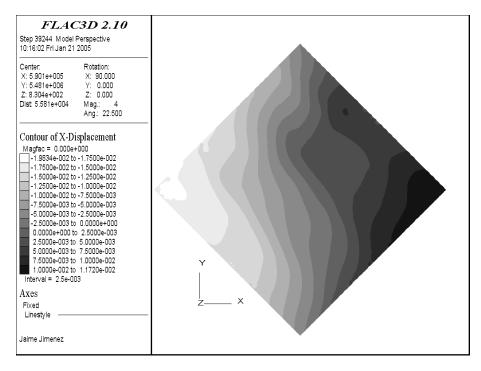
Figure B-25. West-East displacement in the Watrous Formation.
