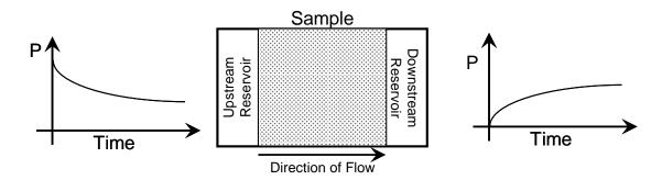
Figure 5-11. Pulse pressure transient technique
