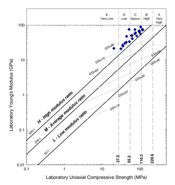
Figure 6-16. Deere classification updated with the Geological Strength Index (GIS) by Martin et al. [186] for the anhydrite database
