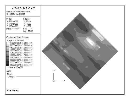
Figure B-24. Pore pressures in the Frobisher Evaporite Formation.
