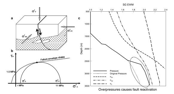
Figure 3-6. (a) Three-dimensional block diagram including the fault that may have reactivated; (b) Mohr circle during fault reactivation. Failure envelope calculated from shales at ~1800 m that are used as analogues; (c) Pressure and stress versus depth as specific gravity, modified after Grauls and Baleix [54]
