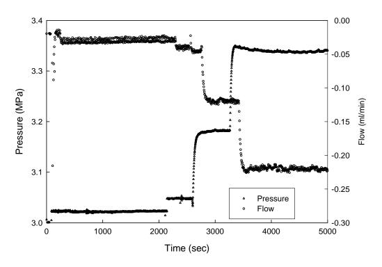
Figure 5-20. Pressure and flow measurements during constant flow permeability measurements
