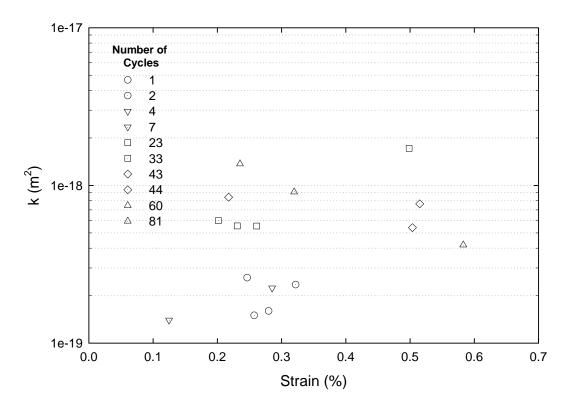
Figure 6-32. Test No. 4, permeability evolution of a Midale Evaporite sheared cyclically under a confining stress of 3 MPa and a pore pressure of 1 MPa against axial strain
