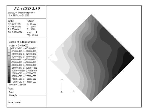
Figure B-26. West-East displacement in the Midale Evaporite Formation.
