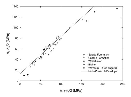
Figure 6-19. Mohr-Coulomb envelope for anhydrites
