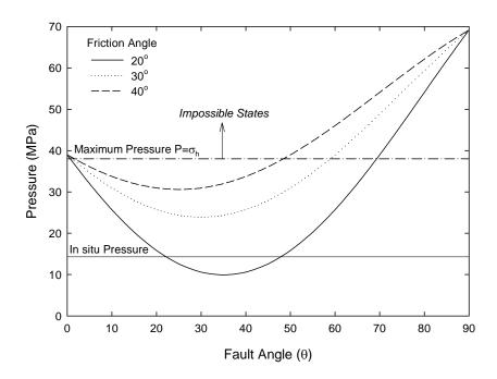
Figure 8-21. Pressure to induce fault reactivation for the base case scenario in a strike slip regime
