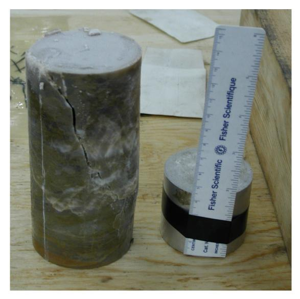
Figure 6-25. Test No. 2, brittle failure of a Three Fingers sample sheard under a confining effective stress of 5 MPa. Notice the well-defined shear plane at 32° with the axis of the sample, and the damage induced throughout the sample. The rule measures 15 cm
