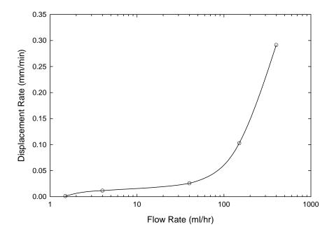
Figure A-6. Displacement rate vs. flow rate for loading system pump.
