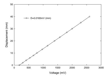
Figure A-2. Calibration of external LVDT.
