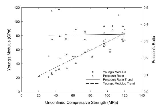
Figure 6-18. Relation between elastic properties and unconfined compressive strength for the anhydrites database
