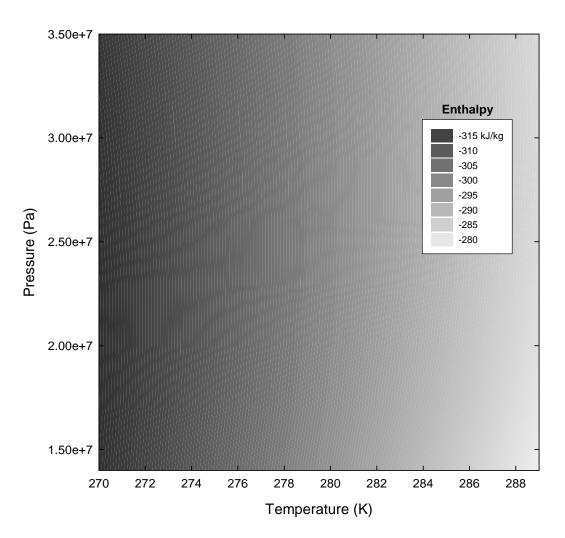
Figure 10-3. CO<sub>2</sub> enthalpy at different pressures and temperatures
