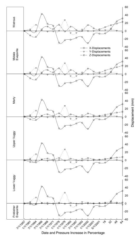
Figure 8-17. Displacements at every formation in the Well 101-16-13-006-14W200 (location shown in Figure 8-1) for the base case scenario
