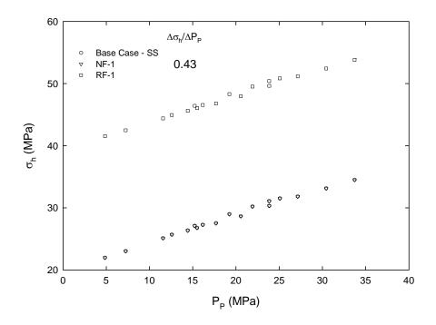
Figure 8-9. Change in horizontal stress due to depletion in the Upper Vuggy at Weyburn from the geomechanical simulations
