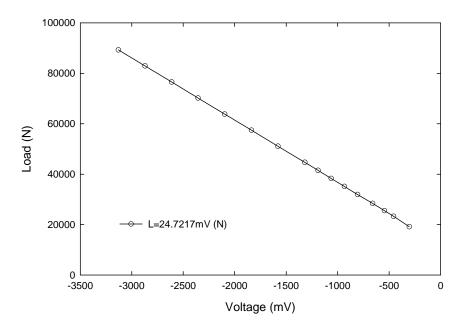
Figure A-5. Calibration of load cell.
