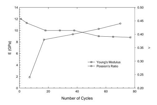
Figure 6-31. Test No. 4, evolution of elastic properties of a Midale Evaporite sample sheared cyclically under a confining effective stress of 2 MPa
