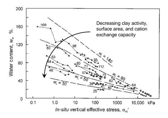
Figure 6-2. Sedimentation compression curves for natural clays, modified after Skempton [118]
