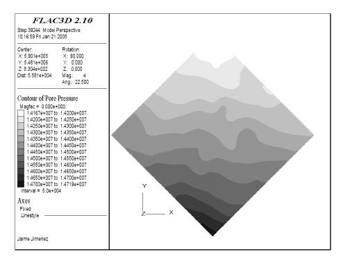
Figure B-20. Pore pressures in the Midale Evaporite Formation.
