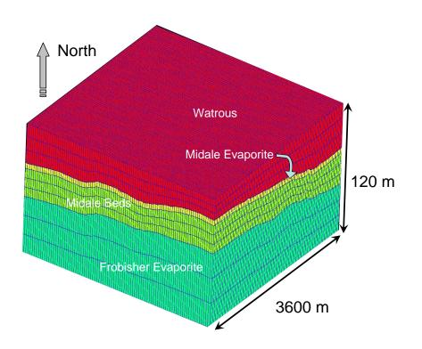
Figure 8-4. FLAC 3D grid used for the geomechanical modeling. The grid honors the geological structure as much as possible
