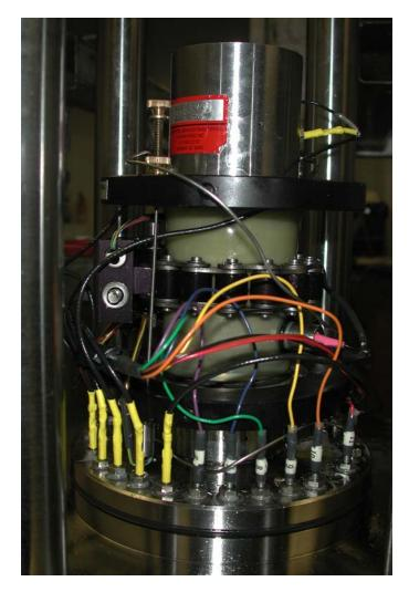
Figure 5-10. Detailed view of side bottom mounted in the sample for radial acoustic measurements
