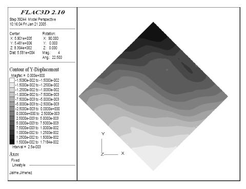
Figure B-31. North-South displacement in the Watrous Formation.
