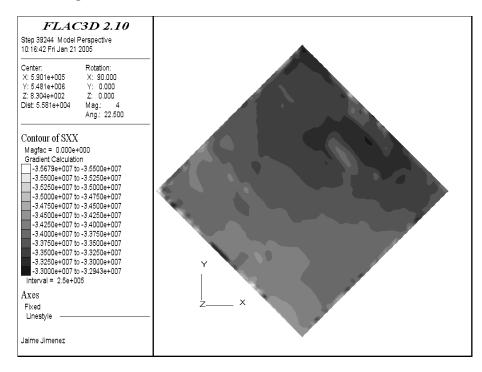
Figure B-2. West-East stresses in the Midale Evaporite Formation.
