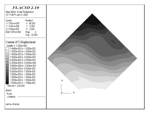
Figure B-33. North-South displacement in the Marly Formation.
