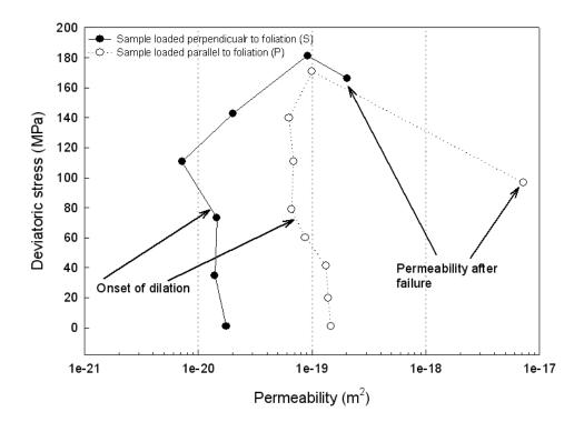
Figure 6-13. Permeability evolution during triaxial compression in Swiss Alps shales, modified after Renner et al. [164]
