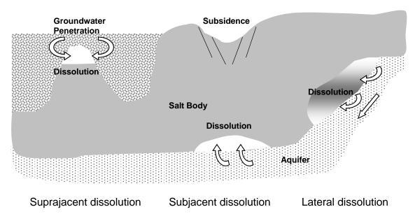
Figure 9-1. Modes of salt dissolution [250]: suprajacent dissolution resulting from groundwater penetration; subjacent dissolution resulting from groundwater flow along sub-salt aquifer units; and, lateral dissolution resulting from circulation along the lateral margins of the salt body
