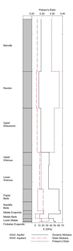
Figure 7-13. Elastic properties of the stratigraphic column at Weyburn
