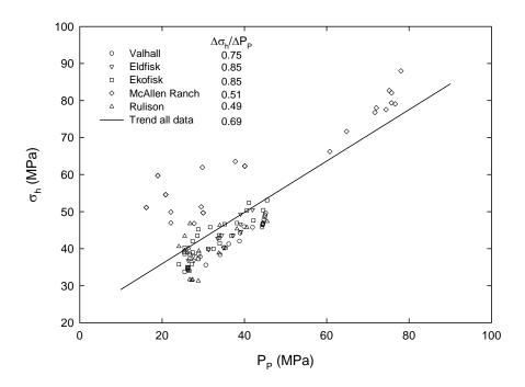
Figure 8-7. Change of horizontal stress with pressure during depletion for multiple oilfields worldwide, data from Teufel [237]
