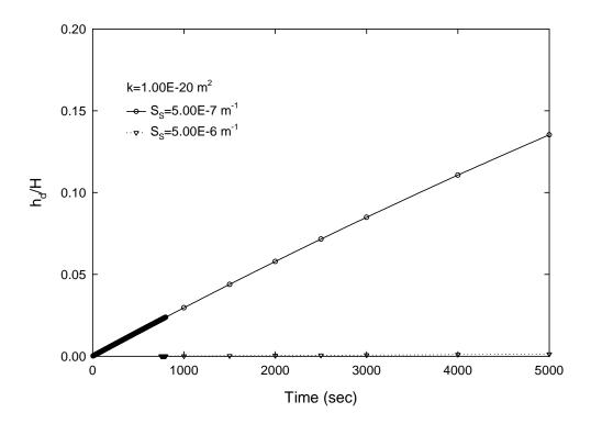
Figure 5-14. Downstream pressure increase for different values of specific storage
