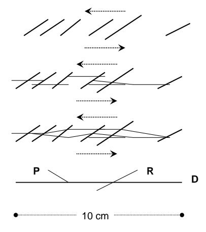
Figure 6-6. Schematic representation of the development and evolution of shear zones, modified after Skempton and Petley [132]
