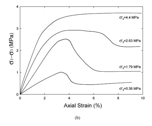
Figure 6-4. Stress-strain behaviour of mudstones: (a) generalized picture; and (b) London clay, modified after Petley [127] and Johnston and Novello [107]
