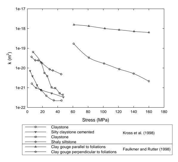
Figure 6-9. Permeability at large pressures for different argillaceous materials
