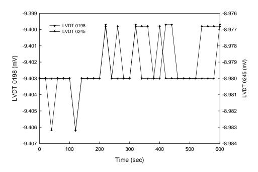
Figure 5-6. Stability of internal LVDT readings. The LVDT 0198 measures axial displacements while the LVDT 0245 radial. The fluctuations account to 5\*10<sup>-4</sup> and 6\*10<sup>-4</sup> mm respectively
