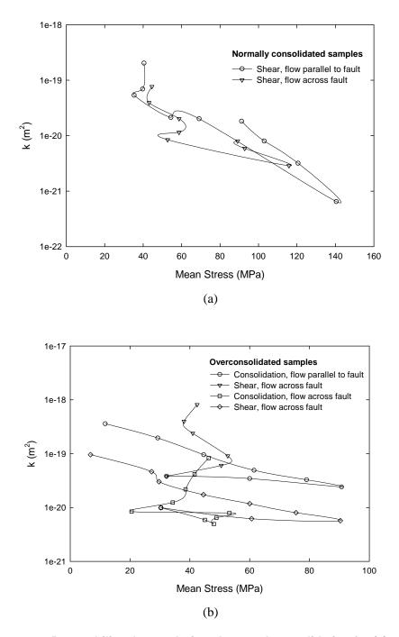
Figure 6-10. Permeability change during shear and consolidation for (a) normally consolidated sample; and, (b) overconsolidated sample. Notice the increment in permeability during shear for OC samples, modified after Zhang and Cox [161]
