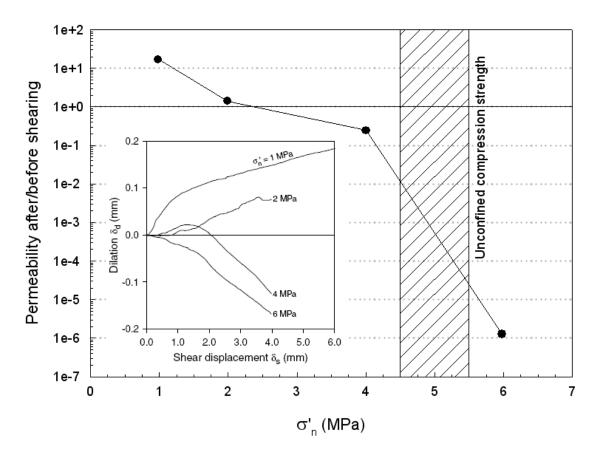
Figure 6-15. (a) Dilation vs. shear displacement for four samples sheared at different effective normal stress; and., (b) change in fracture permeability after shearing the fractures, modified after Gutierrez et al. [77]
