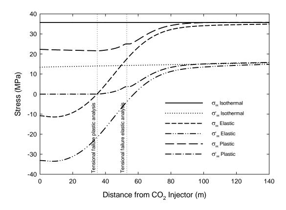
Figure 10-4. Horizontal stresses along the centerline of the reservoir for isothermal and non-isothermal cases, after 208 days of CO<sub>2</sub> injection
