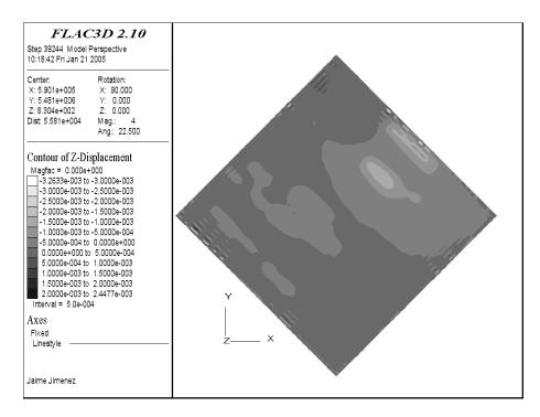
Figure B-42. Vertical displacement in the Frobisher Evaporite Formation.
