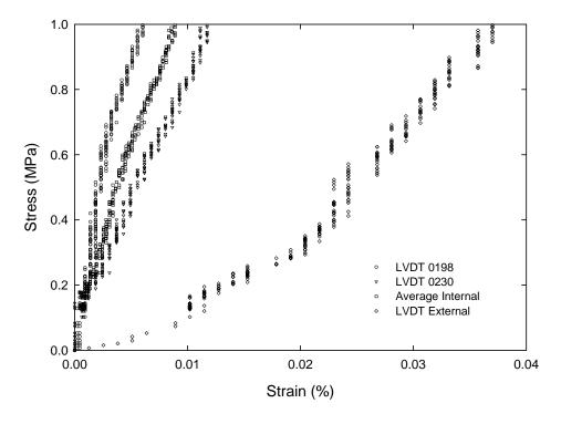
Figure 5-7. Contrast between internal and external LVDT readings
