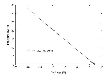
Figure A-4. Calibration of cell pressure gauge.
