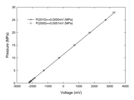
Figure A-3. Calibration of pore pressure gauges.
