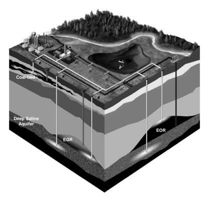
Figure 2-2. Geological storage options, courtesy of ARC
