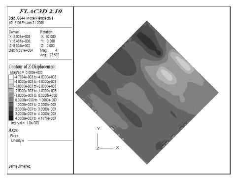
Figure B-37. Vertical displacement in the Watrous Formation.
