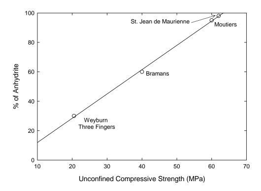
Figure 6-17. Unconfined compressive strength as a function of anhydrite content
