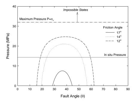
Figure 8-23. Pressure to induce fault reactivation in a normal fault setting
