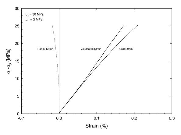
Figure 6-28. Test No. 3, triaxial compression of a Midale Evaporite sample carried out under a confining stress of 30 MPa and a pore pressure of 3 MPa. It was not possible to achieve failure due to equipment limitations
