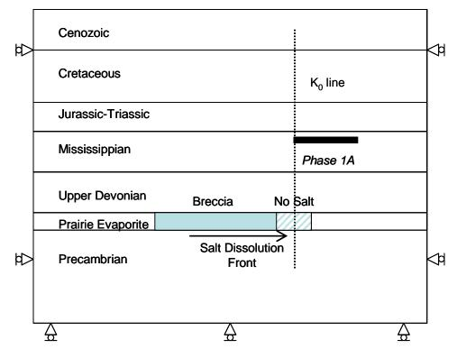
Figure 9-3. Schematic of the geomechanical model
