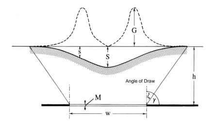
Figure 9-6. Subsidence profile and terminology, modified after Whittaker and Reddish [269]
