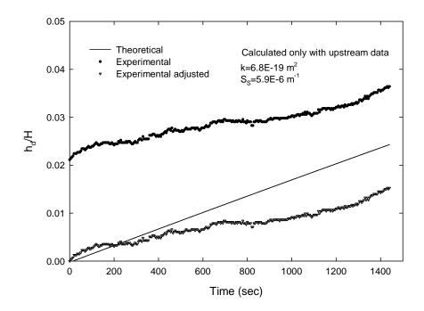
Figure 5-18. Downstream readings during a pulse pressure tests. Because of the low pulse applied and the instantaneous jump in pressure, it is impossible to use these readings to calculate permeability
