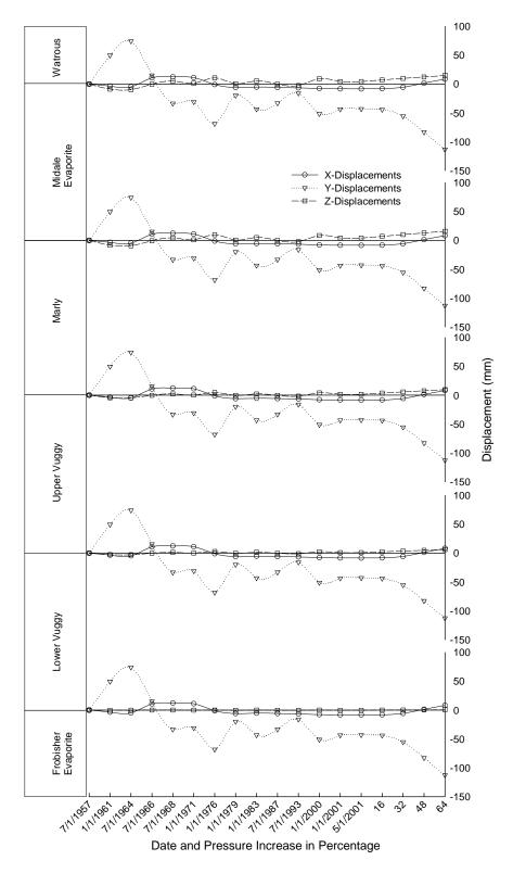
Figure 8-16. Displacements at every formation in the Well 191-10-12-006-14W200 (location shown in Figure 8-1) for the base case scenario
