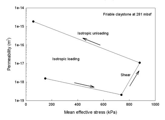
Figure 6-14. Permeability- mean effective stress relationship for a friable claystone retrieved during ODP Leg 170, modified after Bolton et al. [185]
