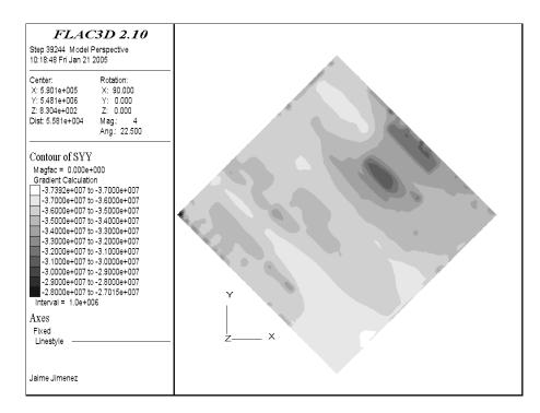
Figure B-12. North-South stresses in the Frobisher Evaporite Formation.
