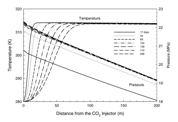
Figure 10-2. Temperature and pressure profiles along the centerline of the carbonate reservoir from 17 days to 208 days of injection
