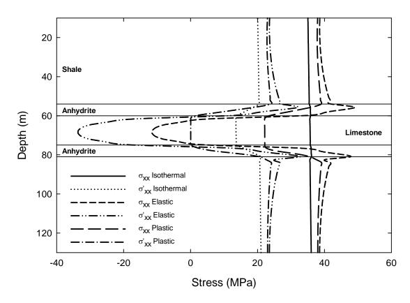
Figure 10-5. Horizontal stresses from top to bottom of the model at a distance of 7.5 m from the injector, after 208 days of CO<sub>2</sub> injection
