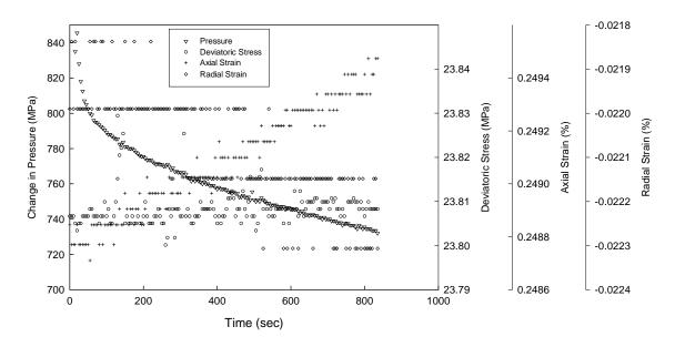
Figure 5-19. Change in deviatoric stress and deformation induced by pulsing
