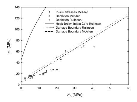
Figure 8-12. Principal stresses for the Rulison (before and after depletion), and the McAllen field (after depletion). Notice that in both cases the final state of stresses is below the damage line. Strength data from Lin [240] and Salz [241]
