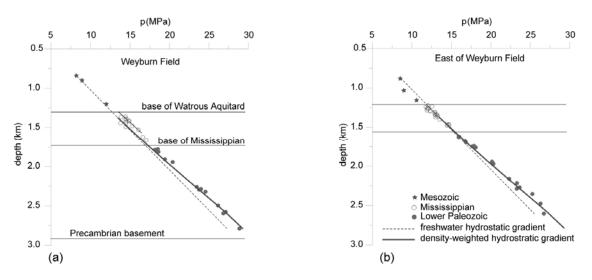
Figure 7-6. Pressure versus depth profile (a) in the Weyburn Fiel, and (b) east of the Weyburn Field, after Khan and Rostron [192]
