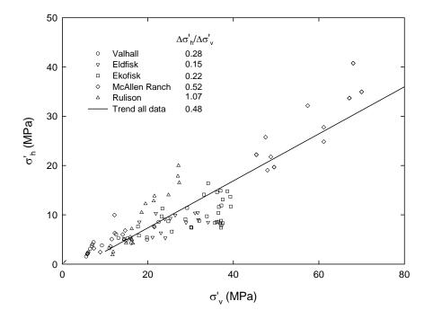
Figure 8-8. Change of both horizontal and vertical effective stress during depletion for multiple oilfields worldwide, data from Teufel [237]
