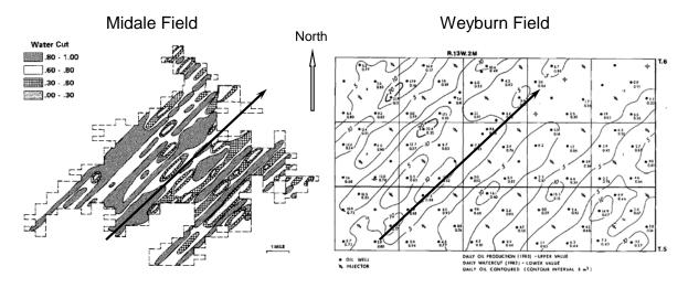
Figure 7-7. Water Cut profile at the Midale Field (Beliveau [201]) and water cut profile at the Weyburn Field (Ko et al. [205]). Notice how both fields follow a NE trend similar to the fractures in both fields
