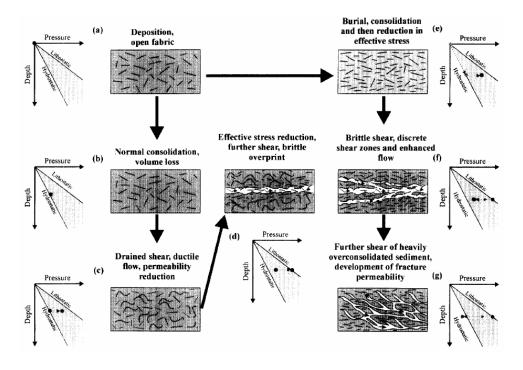
Figure 6-11. Diagrammatic illustration of the different structures observed during the geotechnical cycle, and interpreted fluid pressure relative to hydrostatic. Dots on the respective graphs indicate the fluid pressure at the onset of shear, modified after Bolton and Maltman [163]
