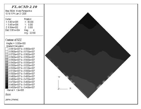
Figure B-13. Vertical stresses in the Watrous Formation.
