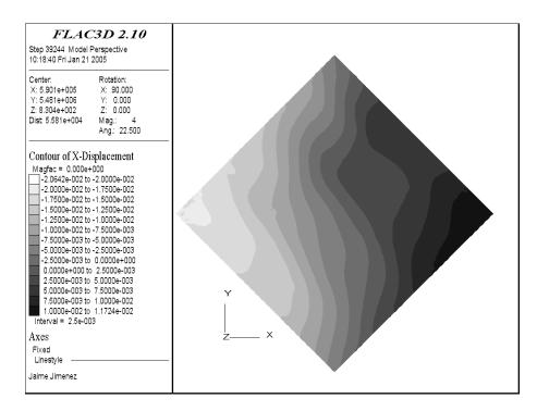
Figure B-30. West-East displacement in the Frobisher Evaporite Formation.
