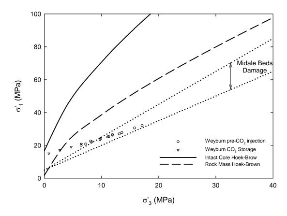
Figure 8-13. Principal stresses for the Weyburn field (before and after CO<sub>2</sub> injection) for the base case scenario. Notice that the final state of stresses is below the damage line during the history of the reservoir. However, once injection pressures are increased around 16% from actual pressures the boundary is crossed
