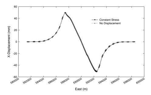
Figure 8-3. Displacements in the west-east direction for both constant stress and fixed boundary conditions
