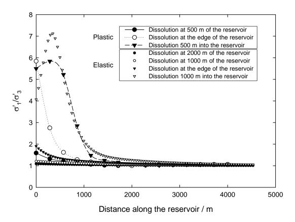
Figure 9-5. Elastic and plastic analysis for 50 m of salt dissolution,  $K_0$ =1.0
