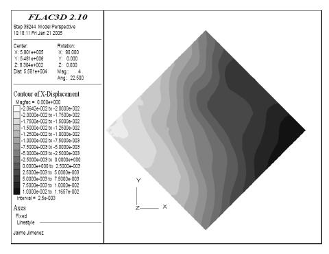
Figure B-29. West-East displacement in the Lower Vuggy Formation.
