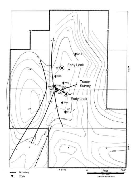
Figure 3-7. Map of the Leroy Storage facility showing the wells with early leaks and the first tracer survey, modified after Araktingi et al. [56]
