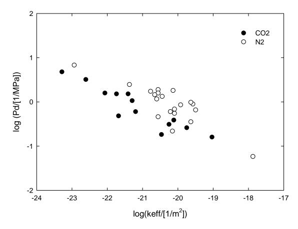
Figure 6-33. Effective permeability and minimum capillary displacement pressure for different argillaceous materials using N2 and CO2, modified after Hildenbrand and Krooss [66]
