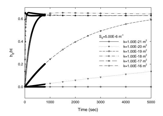
Figure 5-16. Downstream pressure increase for different permeabilities
