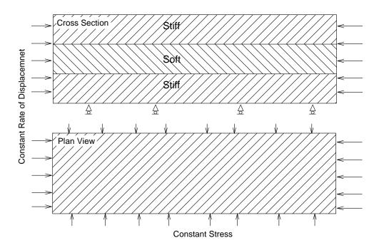
Figure 7-10. Model used to analyze the change in stresses in formations with different stiffnes due to shortening in one direction
