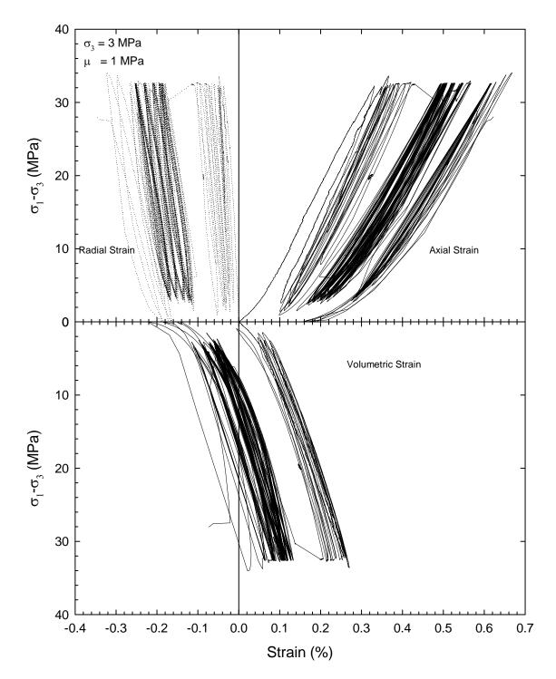
Figure 6-30. Test No. 4, cyclic shear of a Midale Evaporite sample carried out under a confining stress of 3 MPa and a pore pressure of 1 MPa
