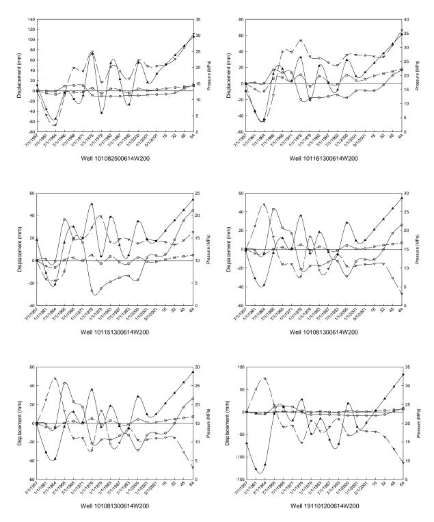
Figure 8-20. Displacement at each well location showed in Figure 8-1 at the Midale Evaporite for the base case scenario
