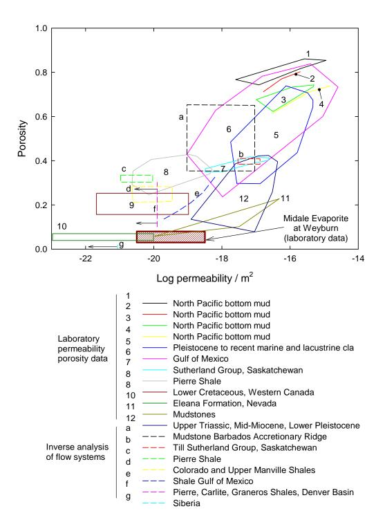
Figure 6-7. Permeability of argillaceous material from both laboratory and inversion of flow systems, modified after Neuzil [156]. The range of permeabilities and porosities measured measured in the laboratory for the Midale Evaporite in this thesis and by Dong et al. [70] are included
