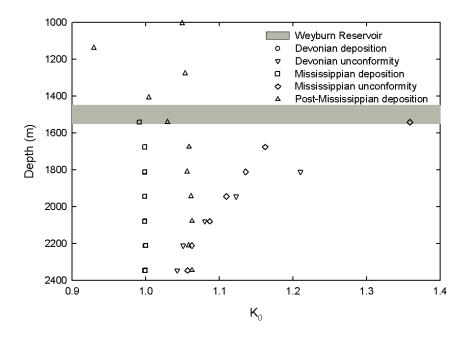
Figure 7-5. Influence of salt dissolution and erosive periods in the in-situ stresses at the Weyburn Field, Phase 1A
