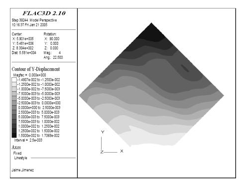
Figure B-32. North-South displacement in the Midale Evaporite Formation.
