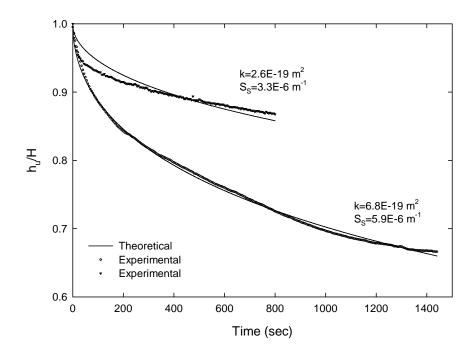
Figure 5-17. Example of two readings and evaluation of permeability using the pulse pressure technique. Only upstream data were acceptable for calculations
