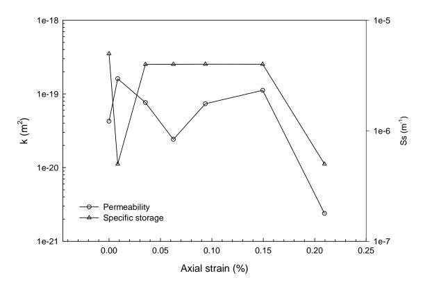
Figure 6-29. Test No. 3, evolution of permeability and specific storage during shear of a Midale Evaporite sample carried out under a confining stress of 30 MPa. The lack of significant change in properties is due to the inability to induce damage in the sample with the experimental equipment available at such a large confining stress
