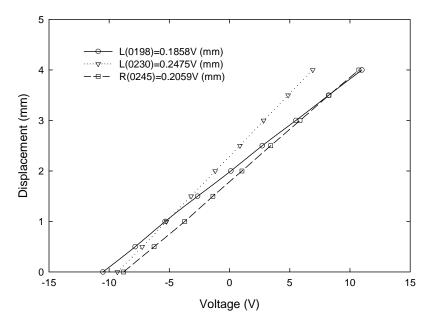
Figure A-1. Calibration of internal LVDTs, axial (L) and radial (R).
