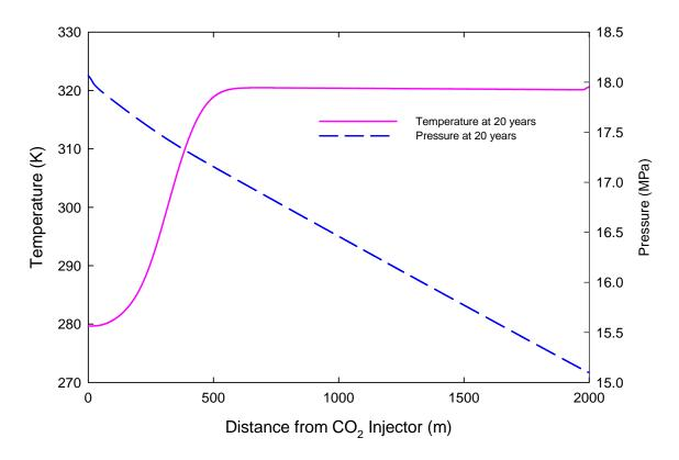
Figure 10-6. Temperature and pressure profile along the centerline of the formation after 20years of CO<sub>2</sub> injection, deep saline aquifer
