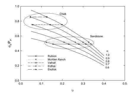
Figure 8-11. Theoretical relation between horizontal stress and pore pressure as a function of Poisson's ration and Biot's coefficient. Notice that the chalk reservoirs presented large subsidence while the sandstone reservoirs did not
