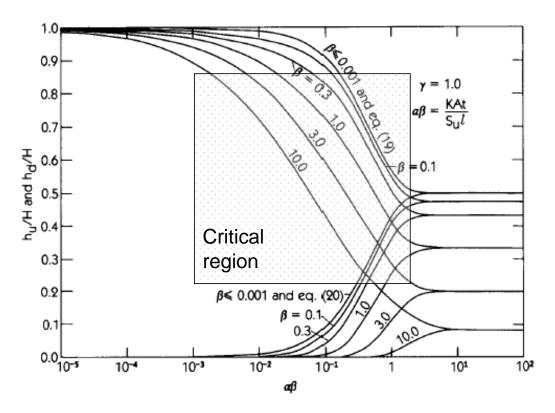
Figure 5-12. Graphical solution to the TPT, modified after Hsieh et al. [97]
