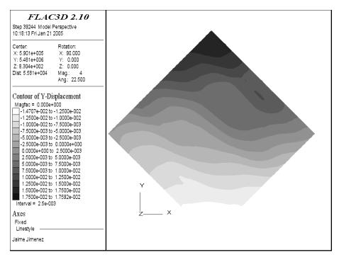
Figure B-35. North-South displacement in the Lower Vuggy Formation.
