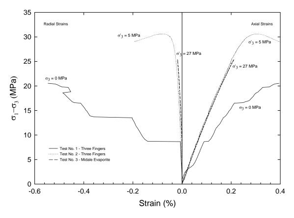
Figure 6-21. Summary of triaxial tests carried out in the both the Three Fingers and Midale Evaporite
