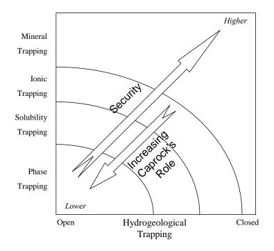
Figure 2-1. Trapping mechanisms for geological storage, modified after Benson et al. [12]
