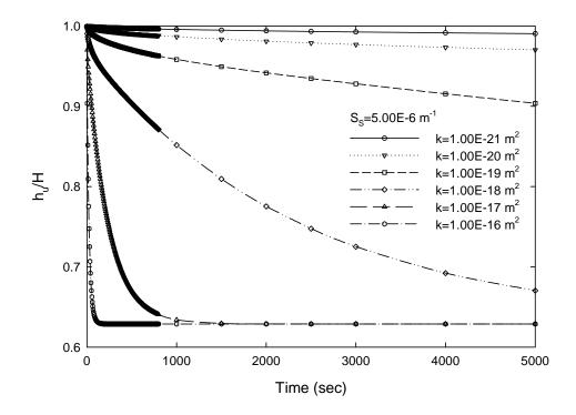
Figure 5-15. Upstream pressure decay for different permeabilities
