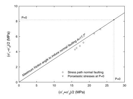
Figure 8-24. Maximum friction angle at which it is possible to induce normal fault reactivation at Weyburn
