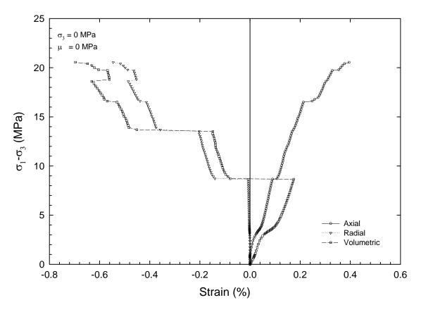
Figure 6-22. Test No. 1, unconfined compression of a Three Fingers sample
