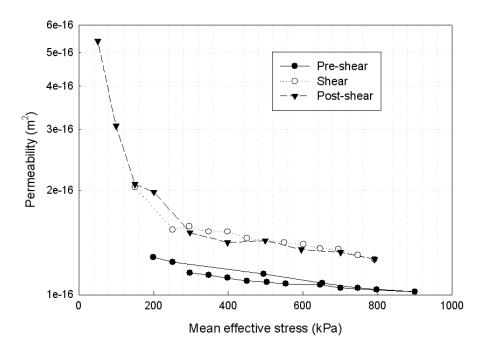
Figure 6-12. Permeability evolution with mean stress for the overconsolidated sample. Notice the permeability dependence on the mean effective stress post-shear, modified after Bolton and Maltman [76]
