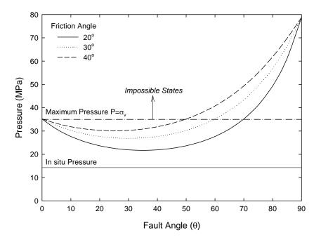
Figure 8-22. Pressure to induce fault reactivation in a reverse fault setting
