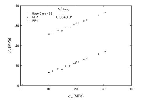
Figure 8-10. Change of horizontal and vertical effective stresses at Weyburn from the geomechanical simulations
