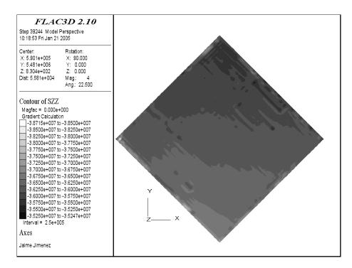
Figure B-18. Vertical stresses in the Frobisher Evaporite Formation.
