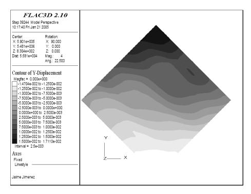
Figure B-34. North-South displacement in the Upper Vuggy Formation.
