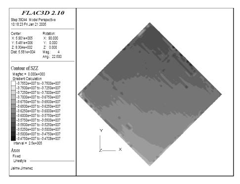
Figure B-17. Vertical stresses in the Lower Vuggy Formation.
