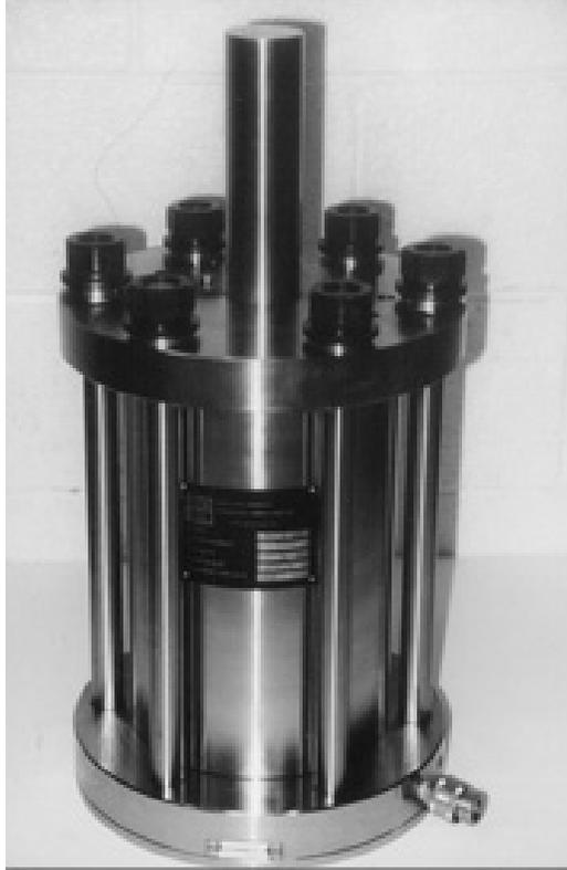
Figure 5-2. High-pressure, high-temperature triaxial cell. The cell is 70 cm tall
