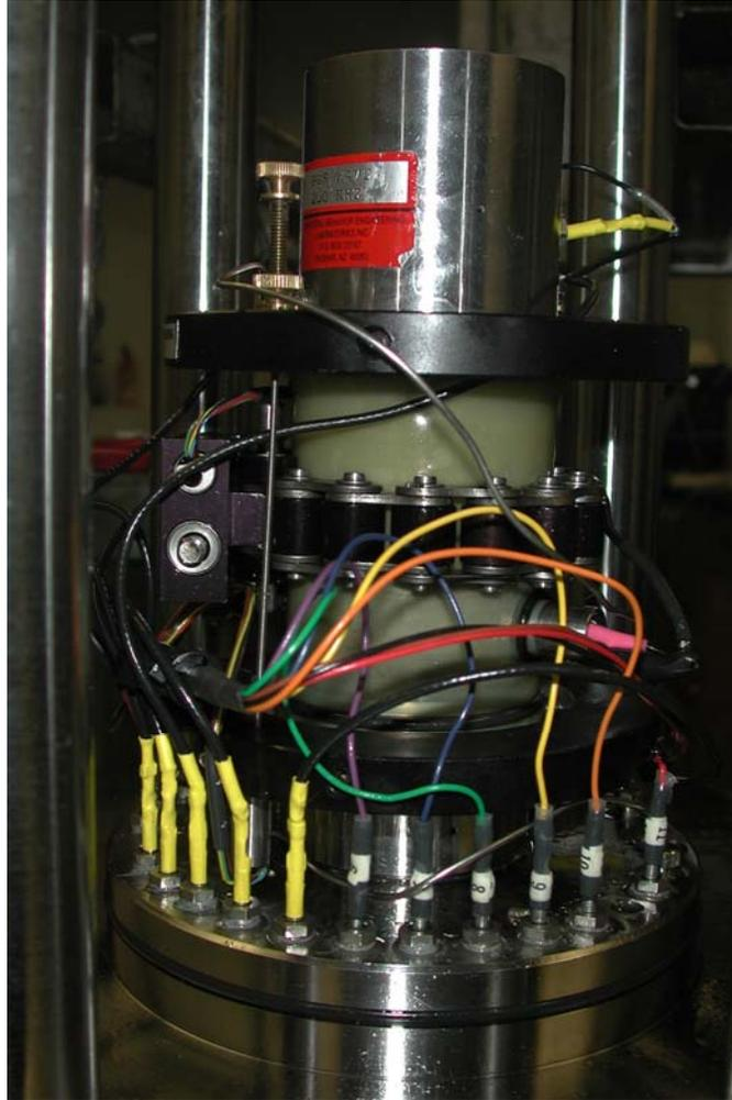
Figure 5-10. Detailed view of side bottom mounted in the sample for radial acoustic measurements
