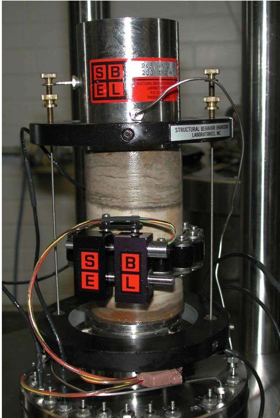
**Figure 5-5. Close-up view of the internal LVDTs system mounted on a sample. Two LVDTs are mounted parallel to the sample to measure axial displacements, and one LVDT mounted in a change measures radial displacements**
