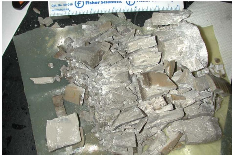
Figure 6-23. Test No. 1, brittle failure of a Three Fingers sample in an unconfined compression test
