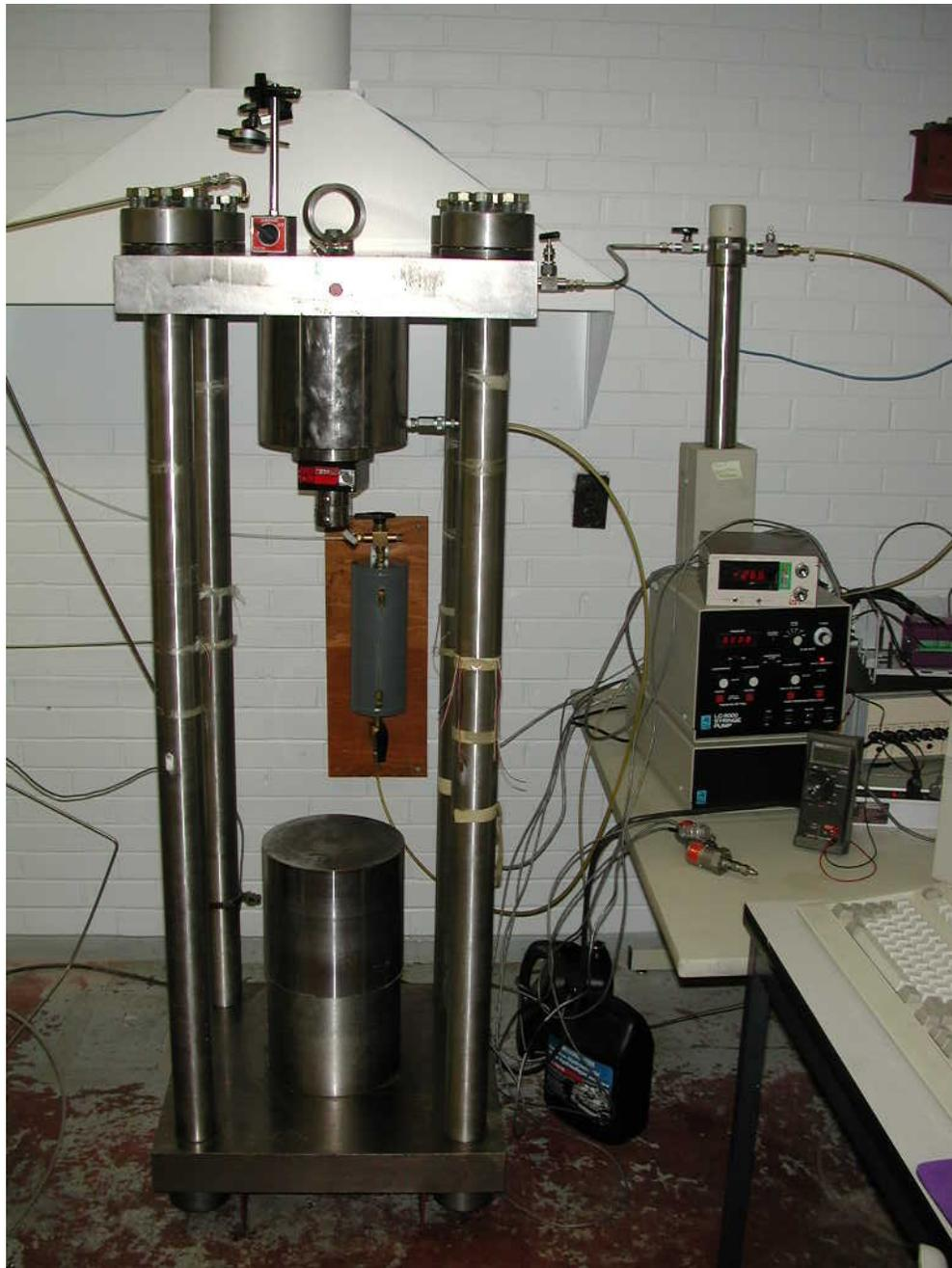
**Figure 5-4. Loading frame and servo-controlled pump for constant strain rate testing**
