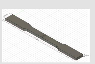
Fig. 5 ASTM-E8 Sample
