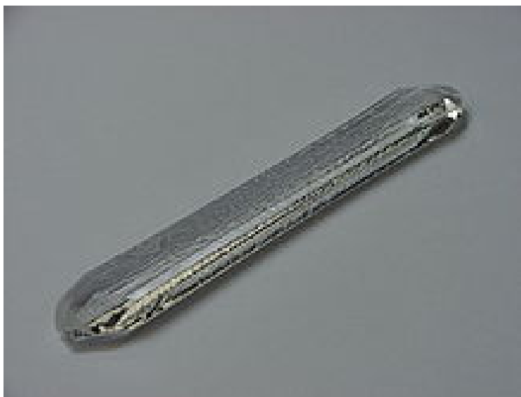
Figure 2.1 A synthetic quartz crystal grown by the hydrothermal method
