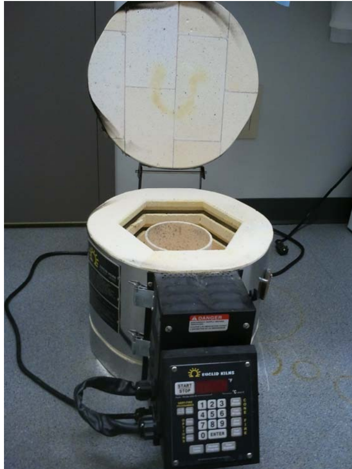
Figure 3.2 The kiln used for sintering
