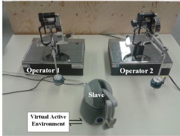
FIGURE 5.8: Trilateral teleoperation experimental setup with the slave robot interacting with virtual active environment
