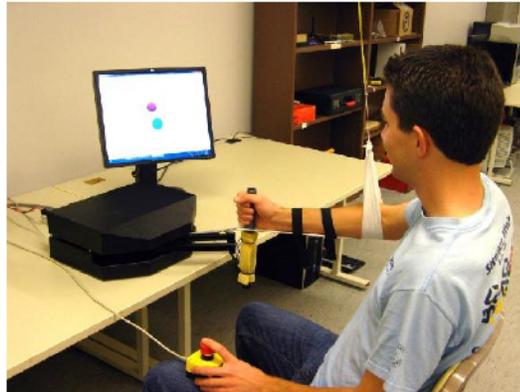
Figure 1: Experiment setup for arm impedance measurement
