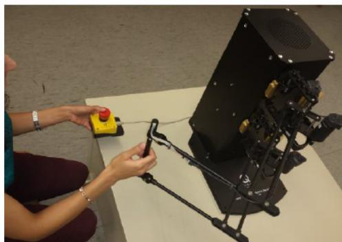
Figure 2: Experiment setup for wrist impedance measurement
