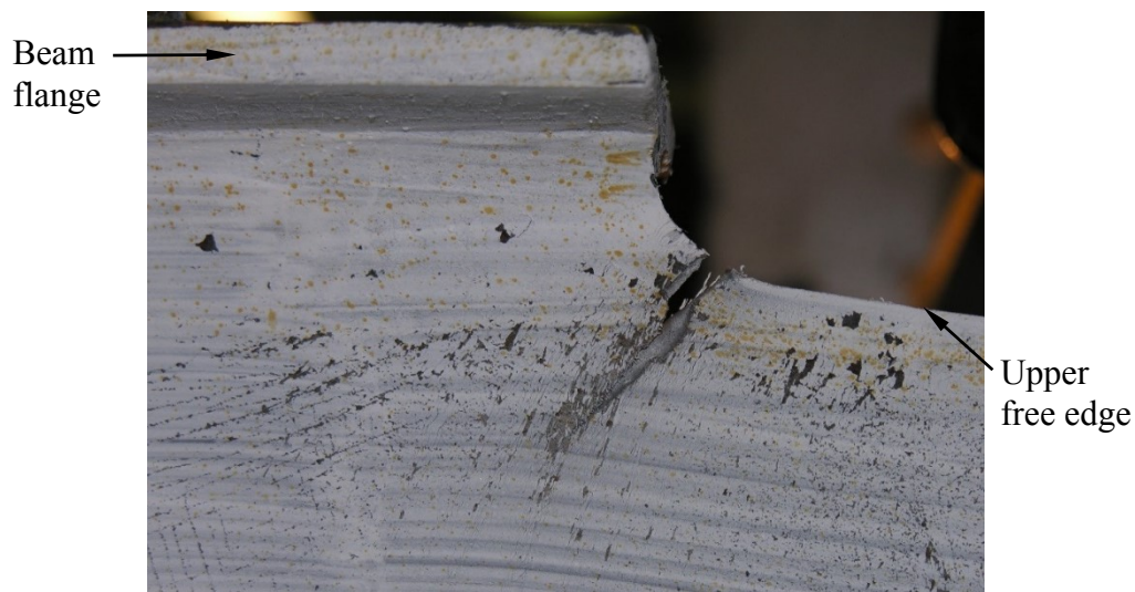
Figure 4-7: In-plane tear in specimen 3A-2-100T-NR
