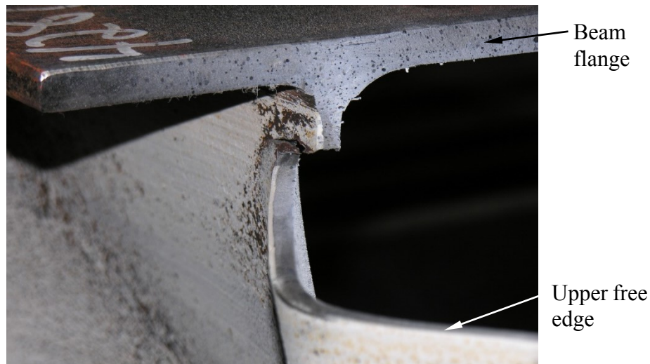
Figure 4-8: Out-of-plane tear in specimen 4B-3-300C-R
