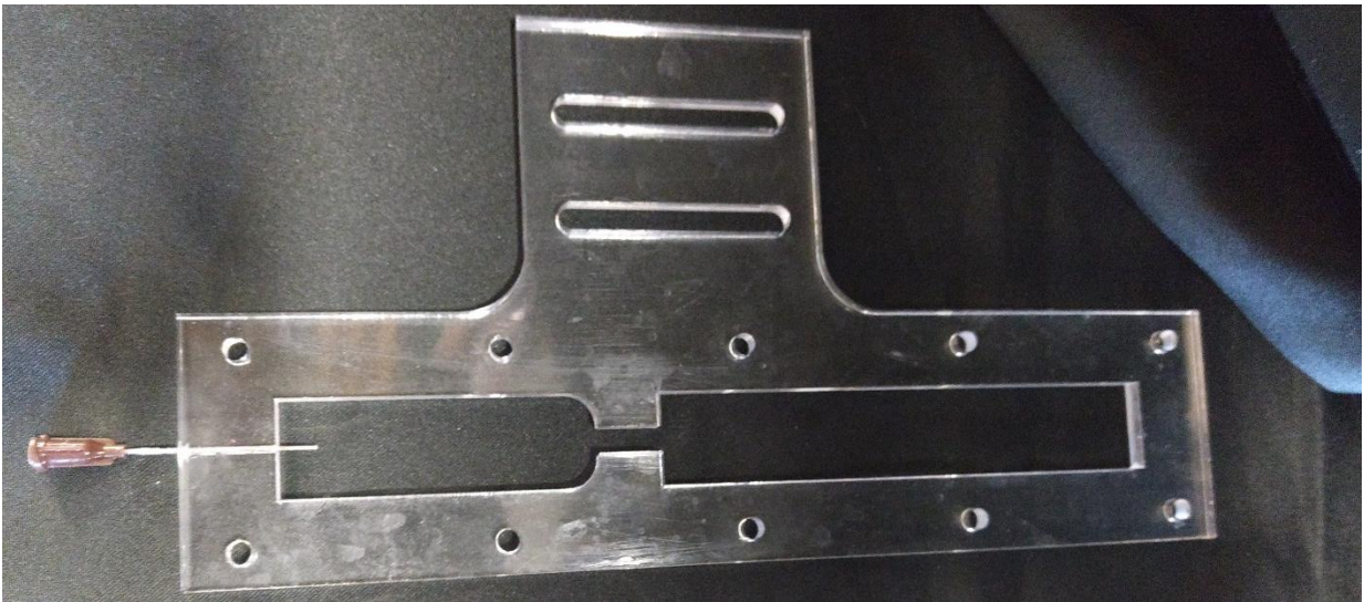
Figure 41 – Flow channel used for rising droplet experiment.
