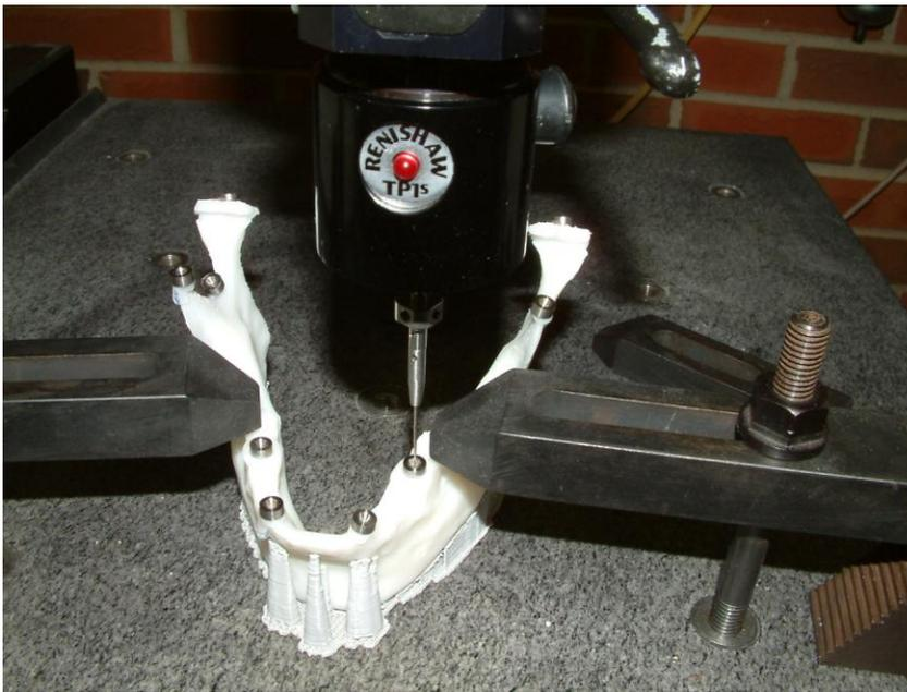
**Figure 4.2:** Mandible rapid prototype model with markers in CMM
