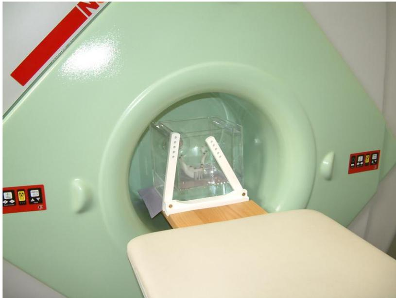
**Figure 4.3:** Mandible rapid prototype model in plexiglass box in NewTom 3G
