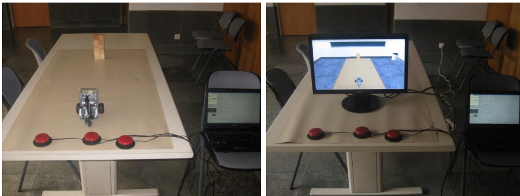
Figure 5: Experimental setups with the physical and the virtual robots
