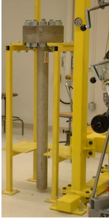
Figure 2.4: The separator of the SFE process (Length: 1.52 m, Inner diameter: 0.0833 m)
