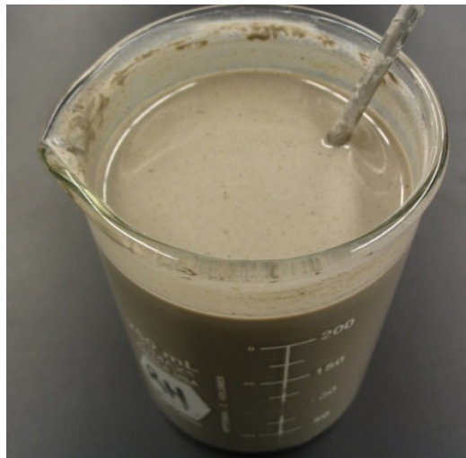
Figure 4.3: Drill cuttings slurry, after blending but prior to dilution
