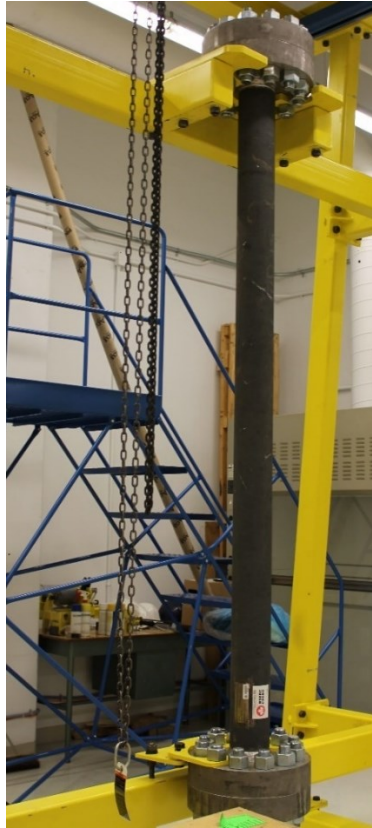
Figure 2.3: The extraction vessel of the SFE process (Length: 2.45 m, Inner diameter: 0.0833 m)
