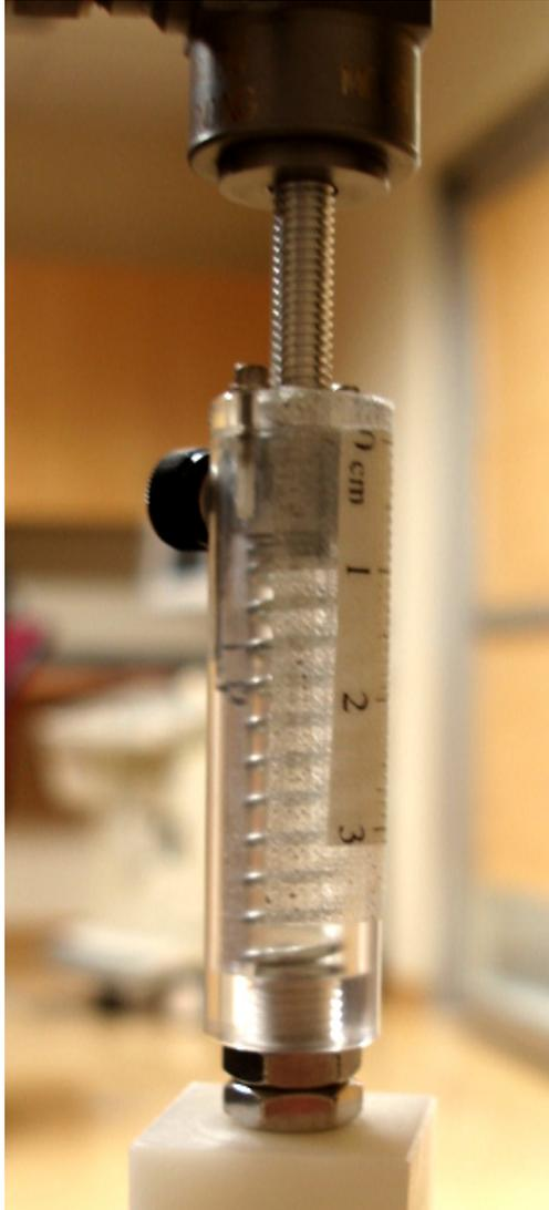
***Figure B.3: Compression spring force gauge in its experimental setup state.***
