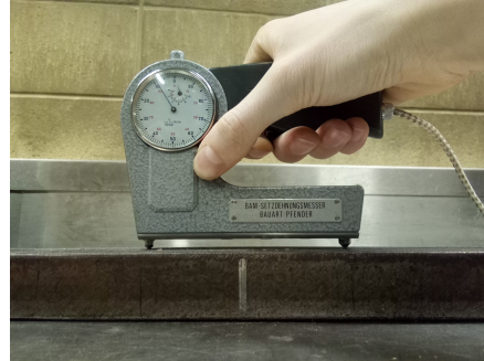
Figure 3.3: Extensometer used for gauge length measurements
