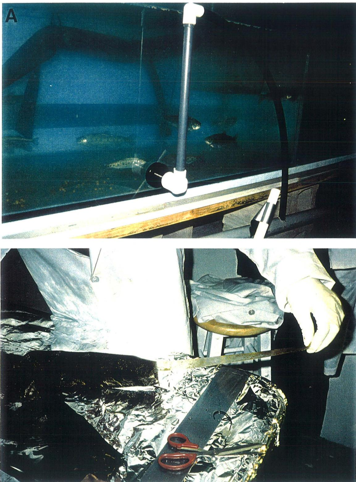
Figure 8. Photograph of a SPMD Deployed in a Tank (a) and Removal from the Holding Net (b)
