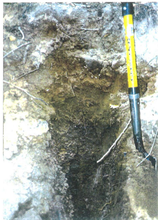
Kinosis soil. Orthic Gray Luvisol on sandy loam to clay loam stony till.
