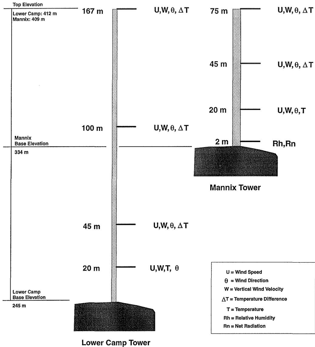
Figure 2.4 Schematic of the meteorological sensor placement at the Lower Camp and Mannix monitoring stations.
