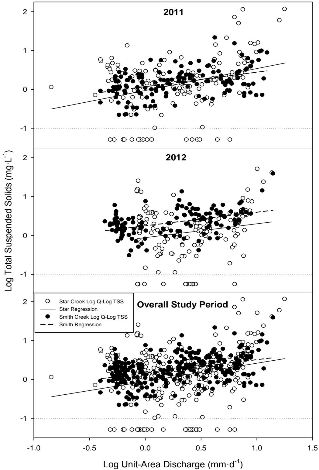
Figure 2-10. Log TSS – Log unit-area discharge relationships for 2011, 2012 and the overall study period for Star and Smith Creeks. Horizontal dotted line indicates limit of detection (LOD = 0.1 mg/L). Data below line was estimated using 1/2 of LOD.
