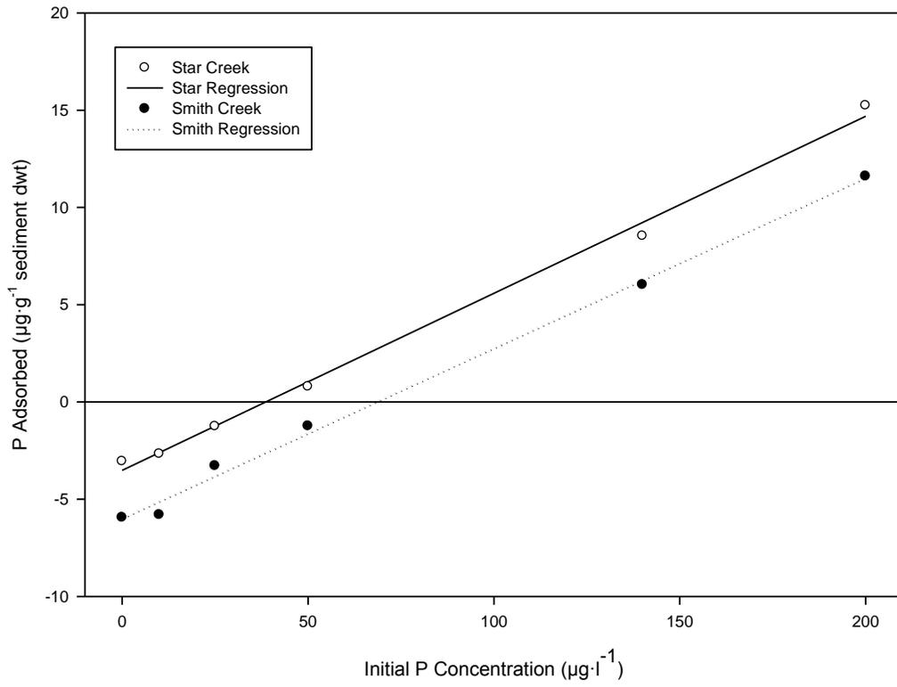
Figure 3-6. Bed sediment P sorption curves for Star and Smith Creeks in 2011. EPC<sub>0</sub> Star = 39 µg·L<sup>-1</sup>. EPC<sub>0</sub> Smith = 68 µg·L<sup>-1</sup>.
