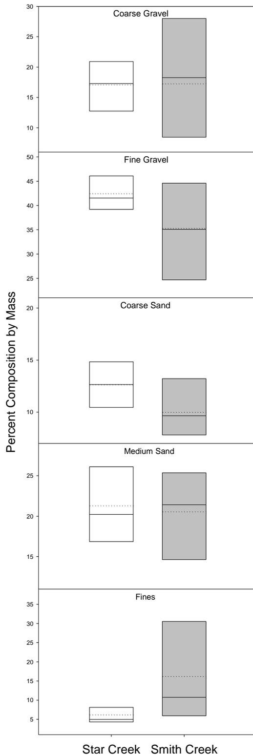
Figure 3-3. Distribution of coarse particle size distributions of bed sediments in Star and Smith Creeks in 2011. Horizontal line in boxplots indicates median, dashed line indicates mean, upper and lower box positions indicate 75th and 25th percentiles.
