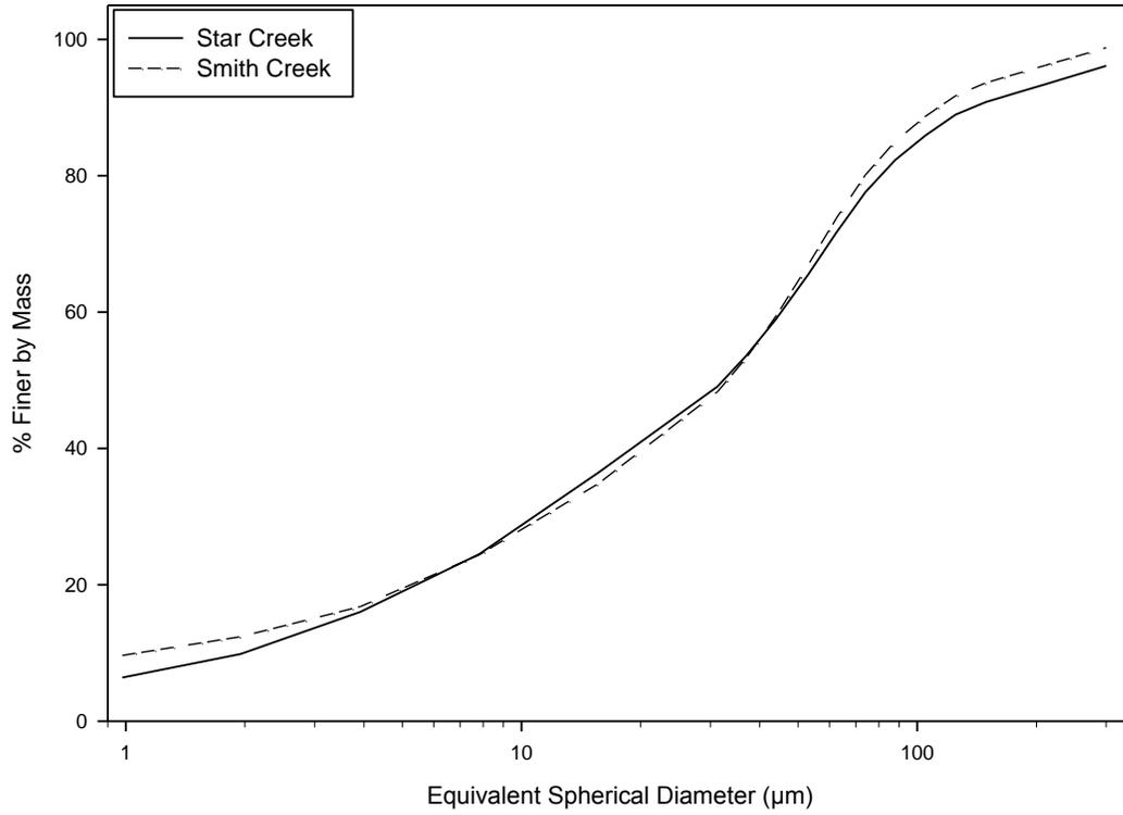
Figure 3-4. Particle size distribution for fine fractions of bed sediments of Smith and Star Creeks in 2011.
