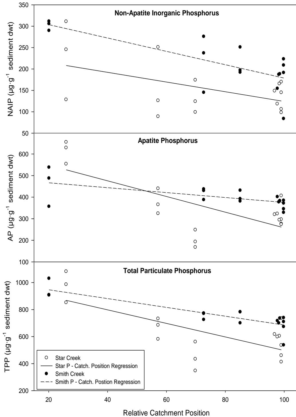
Figure 2-12. Relationship between relative reach position within catchments and concentration of sediment P species. Zero and 100 indicate most upstream and downstream reach positions, respectively.
