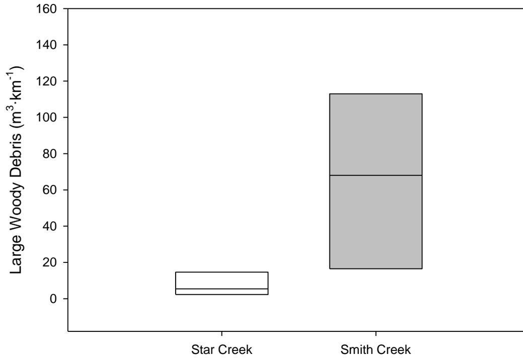
Figure 3-7. Distribution of large woody debris (LWD) volumes in Star and Smith Creeks in 2012. Horizontal line in boxplots indicates median, upper and lower box positions indicate 75<sup>th</sup> and 25<sup>th</sup> percentiles.
