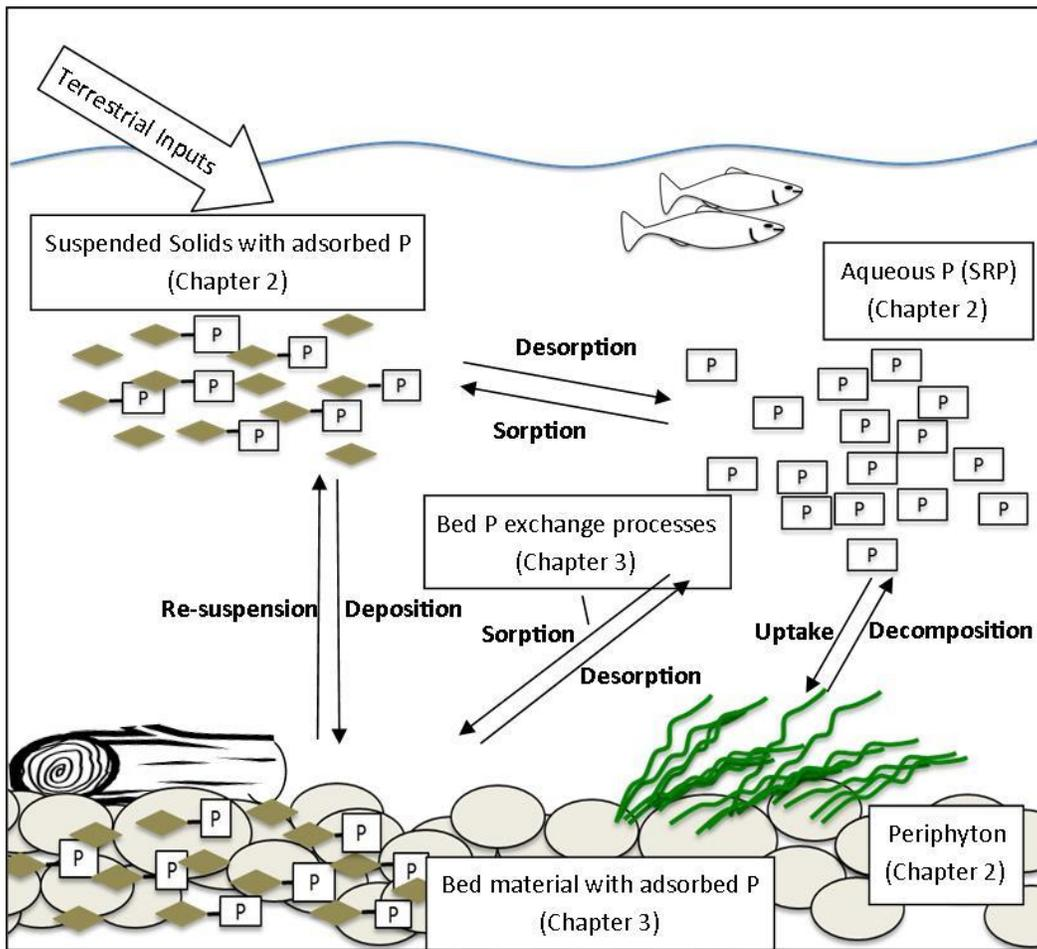
Figure 1-1. Conceptual diagram of stream sediment-phosphorus dynamics, illustrating processes which govern concentrations of each pool of phosphorus/sediment and where each were addressed in the present study.
