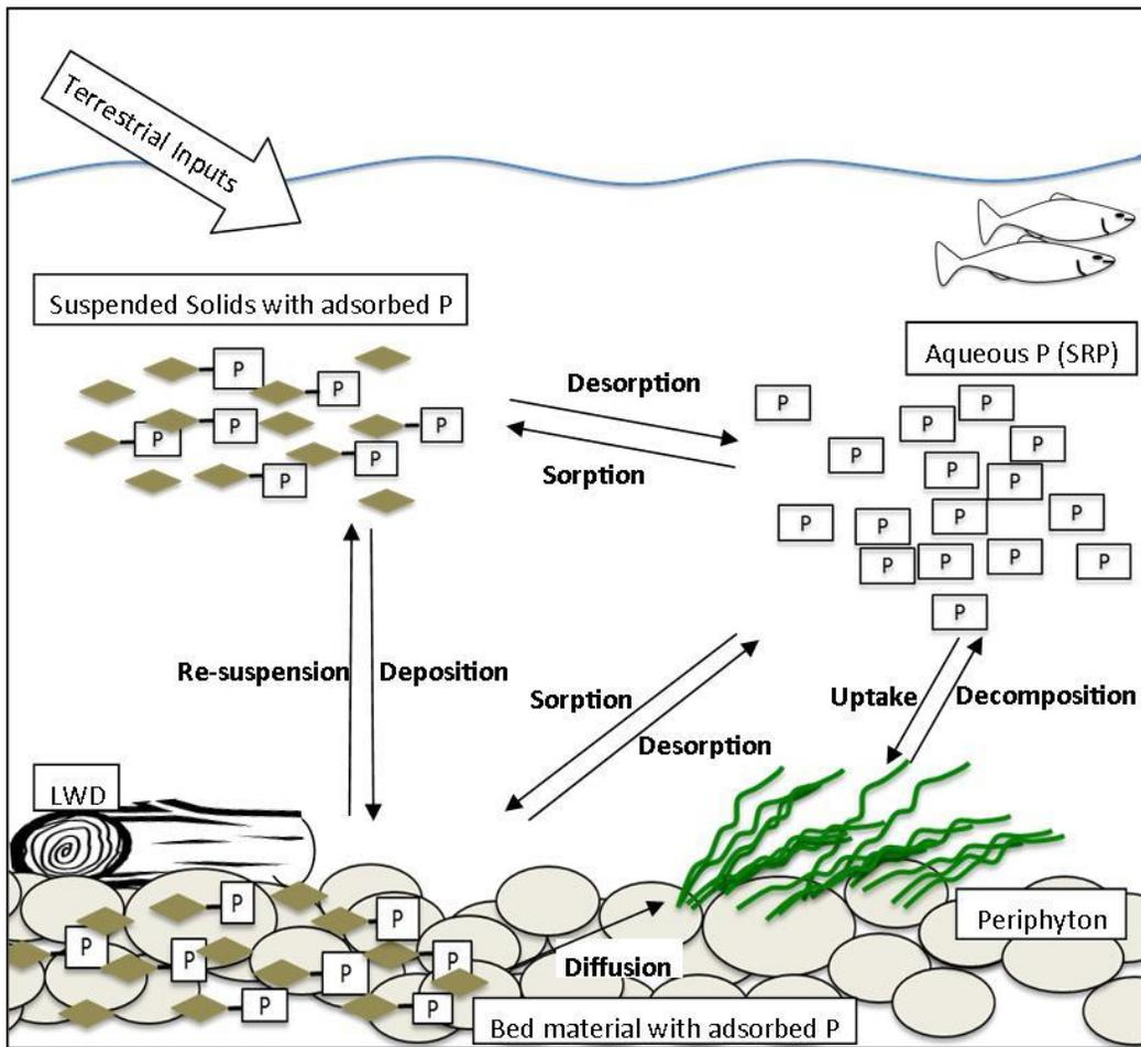
Figure 4-1. Conceptual diagram of stream sediment-phosphorus dynamics, illustrating various processes which govern concentrations of each pool of phosphorus.
