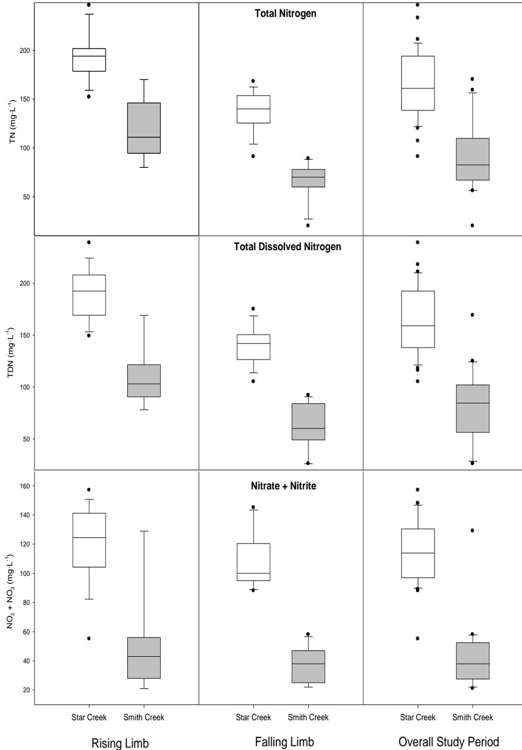
Figure 2-14. Distribution of concentrations of three aqueous nitrogen forms by flow category and overall study period in Star and Smith Creeks. Horizontal line in boxplots indicates median, dashed line indicates mean, upper and lower box position indicates 75th and 25th percentiles, whiskers indicate 95th and 5th percentiles, solid dots indicate outliers.
