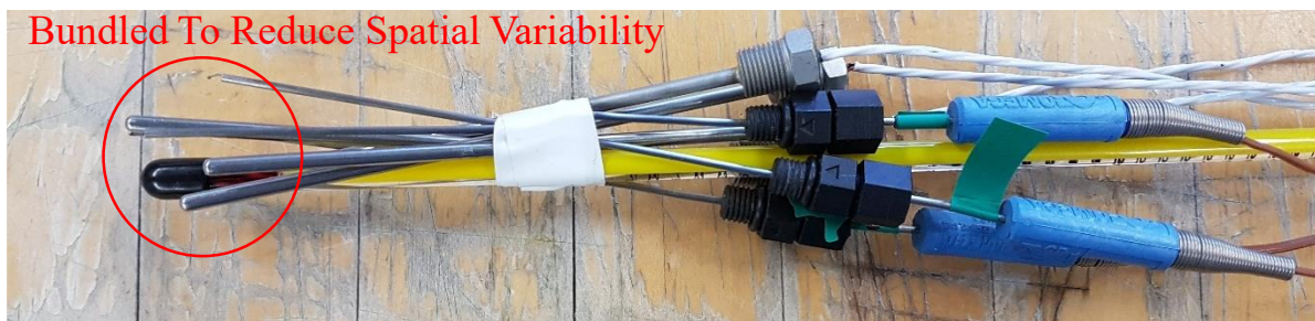
Figure 4-8: Image of the Thermocouple and RTD Bundle
