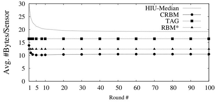
Figure 3.14: Comparison between HIU-Median and CRBM using the default values. HIU-Median starts with a high average performance of approximately 28 bytes per sensor in the first round, which then drops to about 20 bytes by the fifth round and remains stable. CRBM starts at 14 bytes, drops to 10 bytes by the fifth round, and maintains this level. TAG and RBM\* maintain constant average performances of 16 and 12 bytes per sensor, respectively, throughout the 100 rounds.
