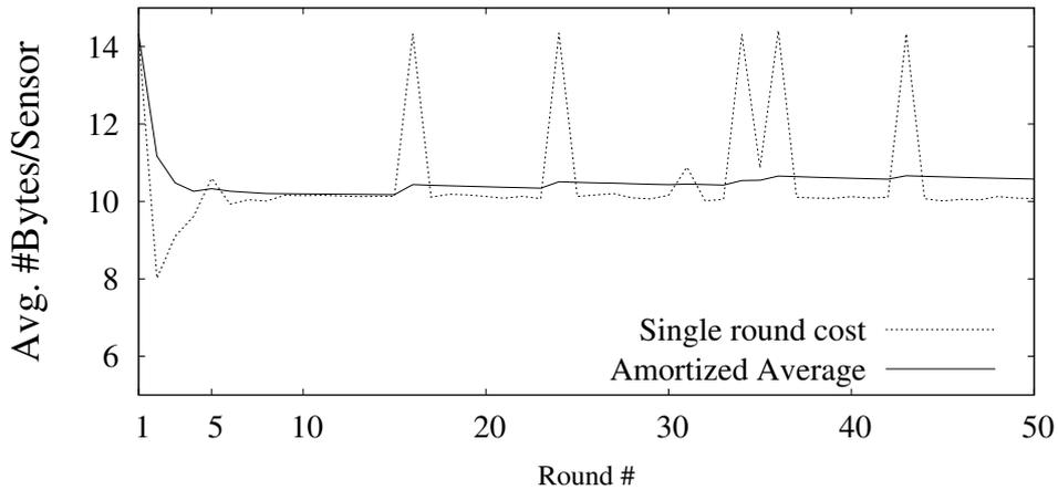
Figure 3.12: Per-round cost vs. Amortized average for the CRBM algorithm
