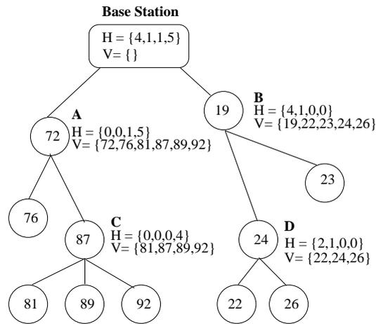
Figure 3.1: Processing a median query.
