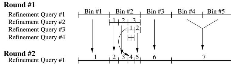
Figure 3.4: Example for constructing the first refinement in the CRBM algorithm
