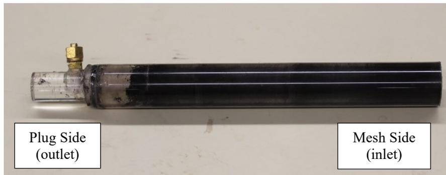
**Figure 2-2. A 25-cm-long crushed-shale pack used in the horizontal and vertical imbibition experiments.**
