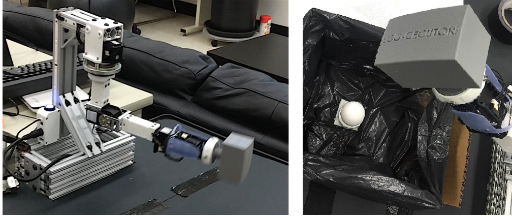
Figure 3.3: Experimental setup, showing the robot arm in motion for the first experiment (left) and the robot arm poised to impact an egg during the second experiment (right).
