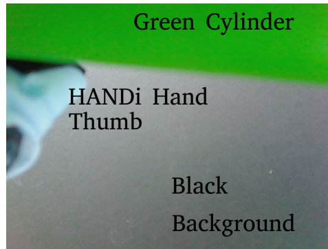
Figure 5.5: The camera's 480 x 640 RGB view of the green cylinder (top) against the black background with the Thumb of the HANDi Hand (left) in view.
