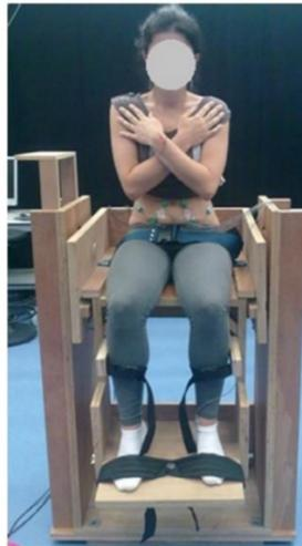
Figure 2-5: An unstable sitting apparatus with one degree of freedom for fundamental investigations of seated balance. Reprinted from [111], with permission (© 2014 Elsevier).
